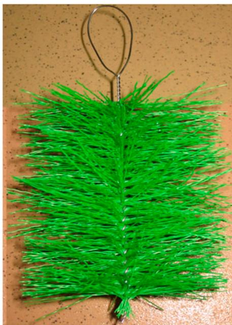
Fig. 2. A three-dimensional elastic inert carrier made from PET.
