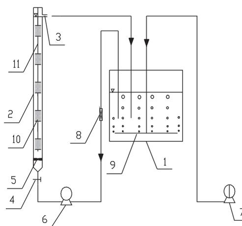
Fig. 1. Schematic diagram of biological culture reactor (1 feed tank; 2 organic glass cylinder; 3 effluent outlet; 4 water valve; 5 circular perforated plate; 6 water pump; 7 air pump; 8 flowmeter; 9 gas distributor; 10 three-dimensional elastic inert carrier; and 11 connecting string).
