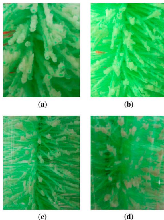
Fig. 3. Biofilms cultured in four reactors (a), (b), (c), and (d) indicated the biofilms on inert carriers at depth of 50 cm in R4, R3, R2, and R1, respectively. Photographs were taken by Canon DIGITAL IXUS 55 before sampling. The attachment of biofilm on internal surface of cylinders of reactors made the photographs a bit obscure.
