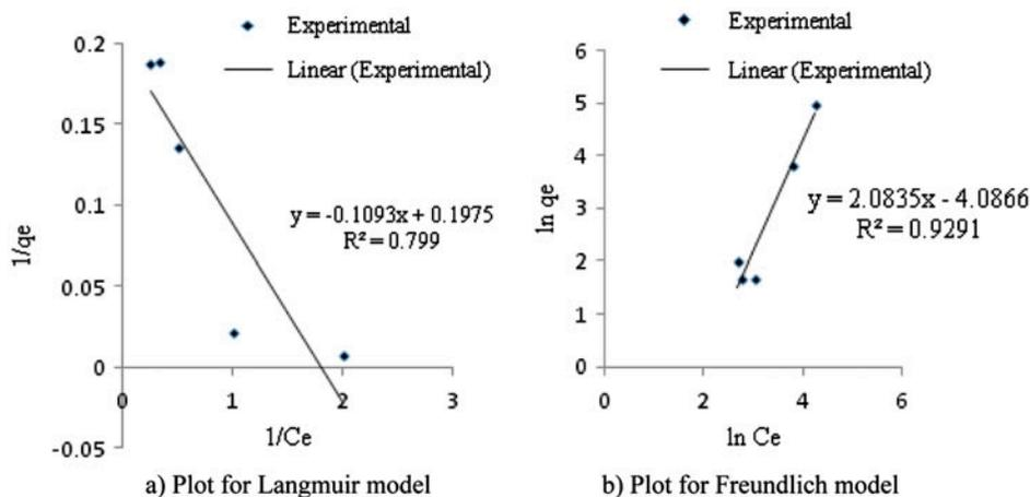
Fig. 9. Langmuir and Freundlich model for coagulation with chitosan as the coagulant.
