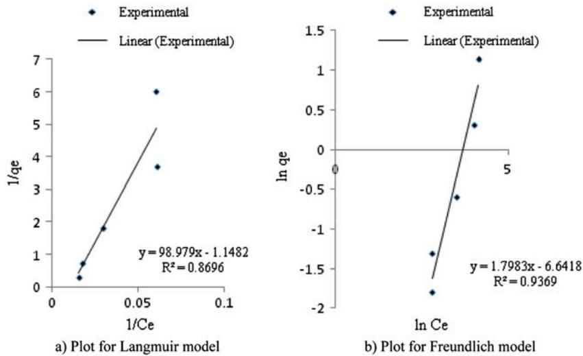
Fig. 10. Langmuir and Freundlich models for coagulation with *M. oleifera* as the coagulant.
