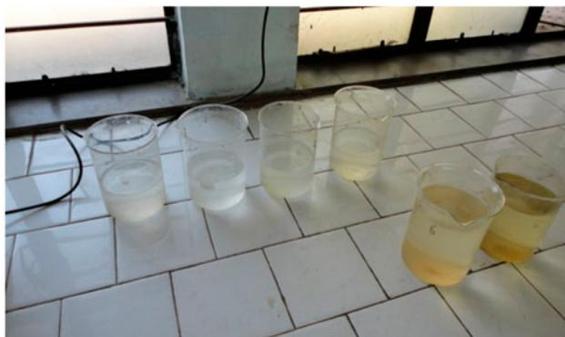
Fig. 2. Jars showing removal of turbidity for various dosages of coagulants.
