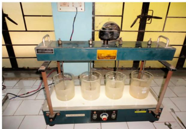
Fig. 1. Jar test apparatus used in the experimentation.
