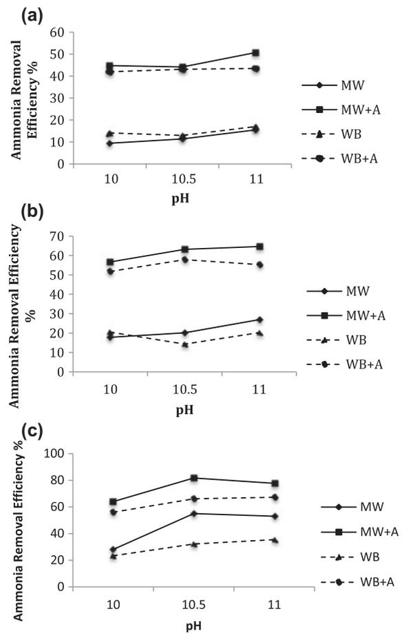
Fig. 4. Ammonia removal rate with MW and M + A at three different radiation time levels: (a) 60 s, (b) 90 s, and (c) 120 s. WB and WB + A with the same final temperature levels: (a) 65°C, (b) 85°C, and (c) 95°C.
