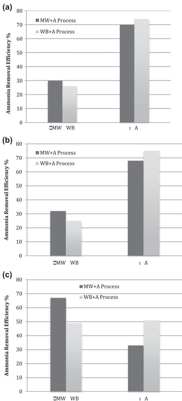
Fig. 7. Contribution of MW WB and aeration (A) during the MW + A and WB + A process under MW different radiation time (WB temperature) (a) 60 s (65°C), (b) 90 s (85°C), and (c) 120 s (95°C).
