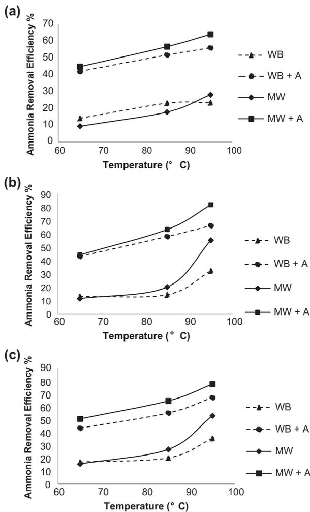
Fig. 5. Ammonia removal using WB and WB + A (MW and MW + A) processes with three final temperature levels: 65, 85, and 95°C (corresponding MW irradiation time levels: 60 s, 90 s, and 120 s) under pH of (a) 10, (b) 10.5, and (c) 11.
