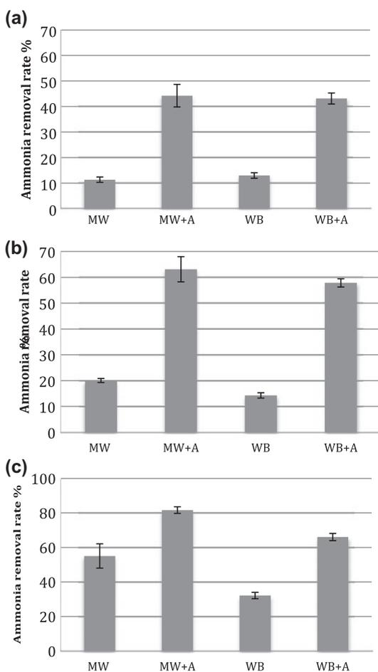
Fig. 6. Ammonia removal using MW and MW + A (WB and WB + A) processes with three MW irradiation time (WB temperature) levels: (a) 60 s (65°C), (b) 90 s (85°C), and (c) 120 s (95°C).
