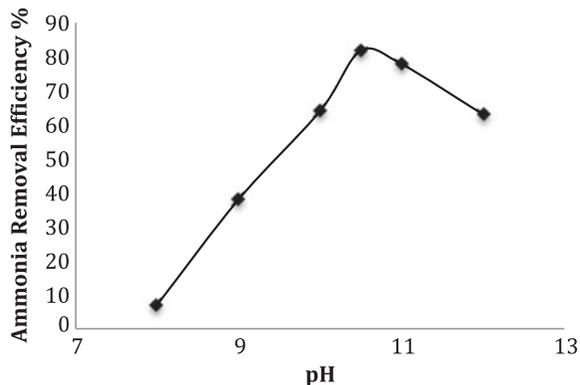
Fig. 3. Preliminary test result of pH, using 50% of the maximum MW power output, 120-s MW radiation time, and the aeration time was 10 min.
