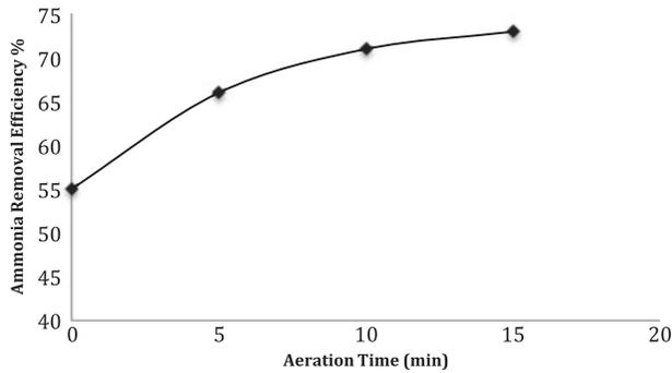
Fig. 2. Preliminary test result of aeration time, using pH 11, 60% of the maximum microwave output, 100 s of radiation time.
