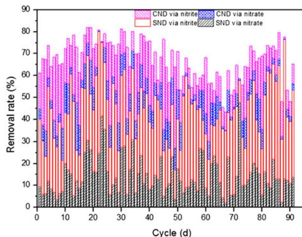
Fig. 5. Four forms of biological nitrogen removal.
