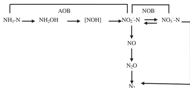
Fig. 1. Biological nitrogen removal process.
