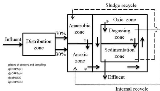
Fig. 2. Schematic diagram of pilot-scale reactor.
