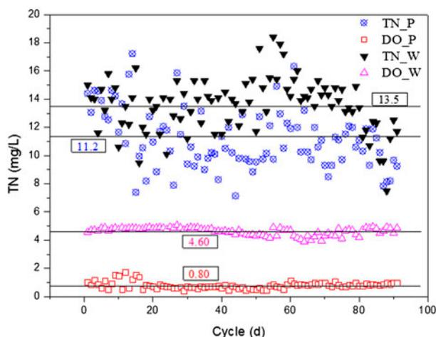
Fig. 6. Nitrogen removal performance and DO level.
