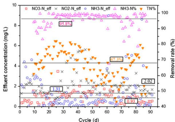
Fig. 3. Nitrogen performance in the pilot reactor (cycle 1 in this figure was actually cycle 49 for the pilot reactor).
