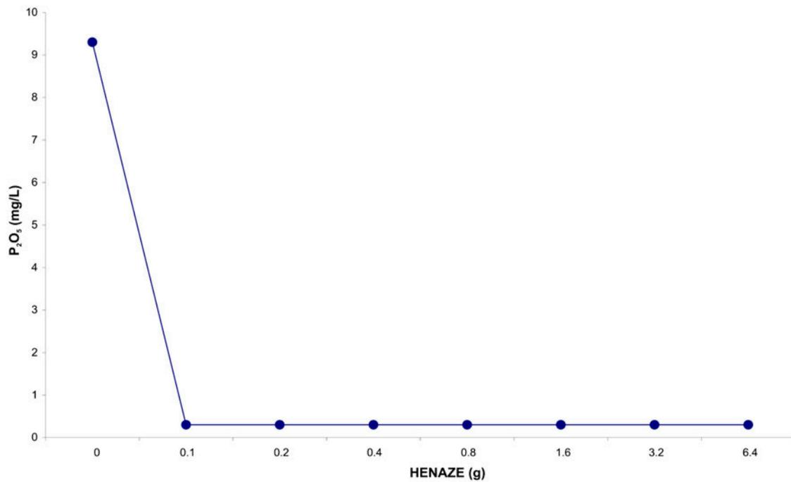
Fig. 7. Decrease in P<sub>2</sub>O<sub>5</sub> concentration with the addition of variable HENAZE proportions.
