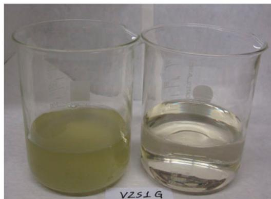
Fig. 4. (Left) Initial Sindos industrial area wastewater (VZS1) and (Right) The overflowing clear water after the treatment with 6.4 g of HENAZE (VZS1G).
