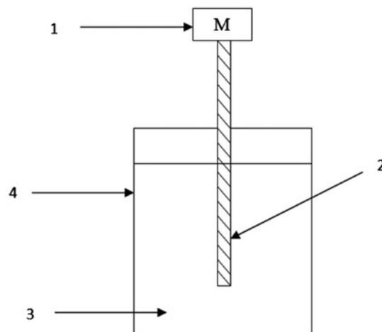
Fig. 1. Schematic diagram of the experimental setup. Notes: (1) Digital Motor, (2) Finned rotating zinc cylinder, (3)  $\text{CuSO}_4$  solution, and (4) Plexiglass container.
