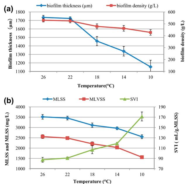
Fig. 3. Changes in biofilm characteristics for varying applied temperature in a modified A<sup>2</sup>O reactor based on measurement of biofilm thickness and density (a) and sludge biomass concentration (b). Concentrations of sludge biomass were determined in terms of mixed liquor suspended solids (diamond), mixed liquor volatile suspended solids (square) and SVI. SVI = SV<sub>30</sub>/MLSS. Error bars are defined as standard error of the mean ( $n = 3$ , technical replicates).
