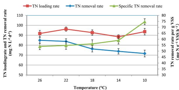
Fig. 2. Changes in the TNRRs, TNLRs, and specific TN removal rates in modified A<sup>2</sup>O system. Error bars are defined as standard error of the mean ( $n = 3$ , technical replicates).
