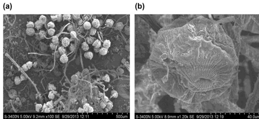
Fig. 6. SEM pictures of the biofilm of experiments with suspended carrier: (a) biofilm on suspended carrier and (b) partial enlarged image of (a).
