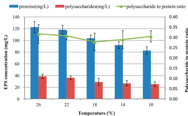
Fig. 4. EPS correlation with temperature. Total EPS was extracted from the sludge biomass and quantified for the extracellular polysaccharides (PS) and extracellular proteins (PN) components. Error bars are defined as standard error of the mean ( $n = 3$ , technical replicates).
