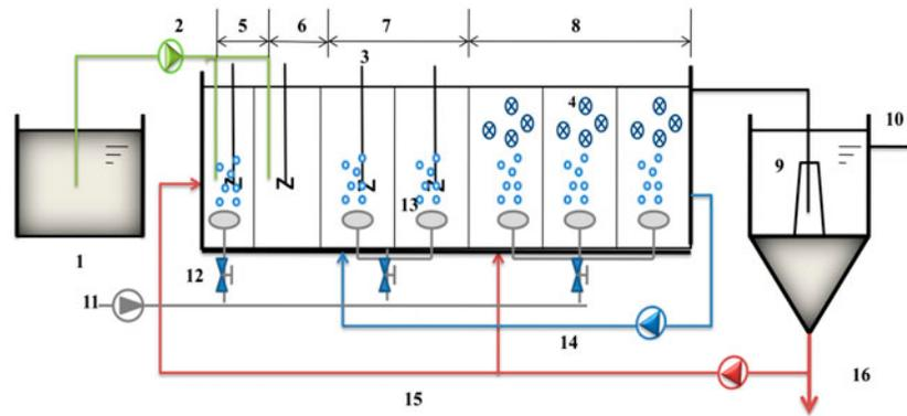
Fig. 1. Schematic diagram of the lab-scale modified A<sup>2</sup>O reactor.
