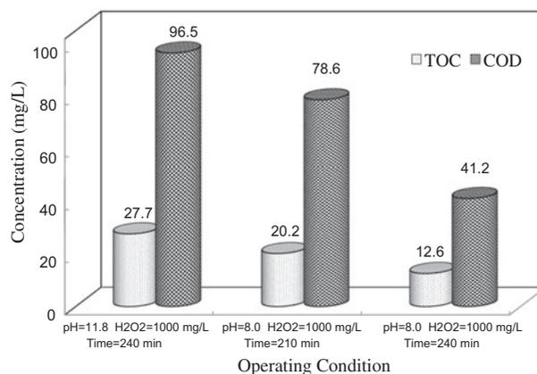
Fig. 8.  $\text{H}_2\text{O}_2/\text{UV}$  operating conditions of TOC < 30 mg/L.
