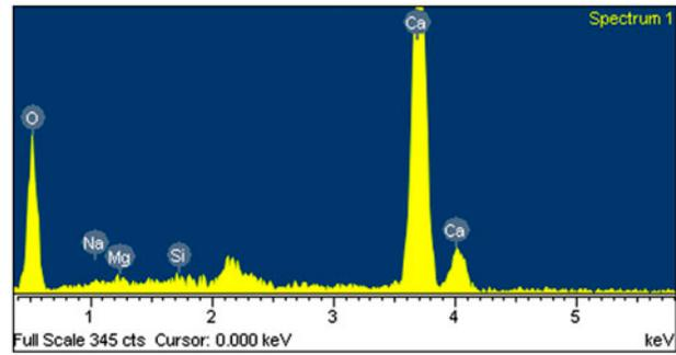
Fig. 6. Element analysis of 1,000°C-calcined OSP.
