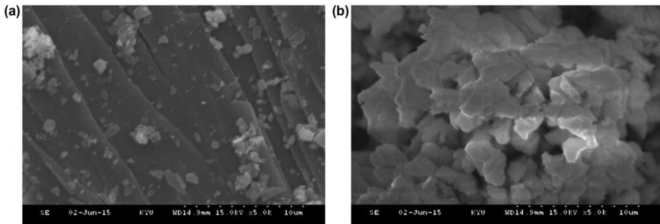
Fig. 5. (a) SEM image of original OSP and (b) SEM image of 1,000°C-calcined OSP.
