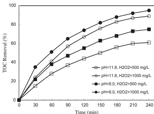
Fig. 7. TOC removal by  $\text{H}_2\text{O}_2/\text{UV}$  oxidation.
