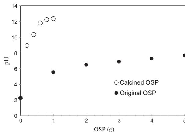
Fig. 4. Solution pH after adding OSP.
