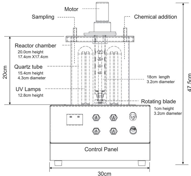
Fig. 1. Experimental setup of the batch photo reactor.
