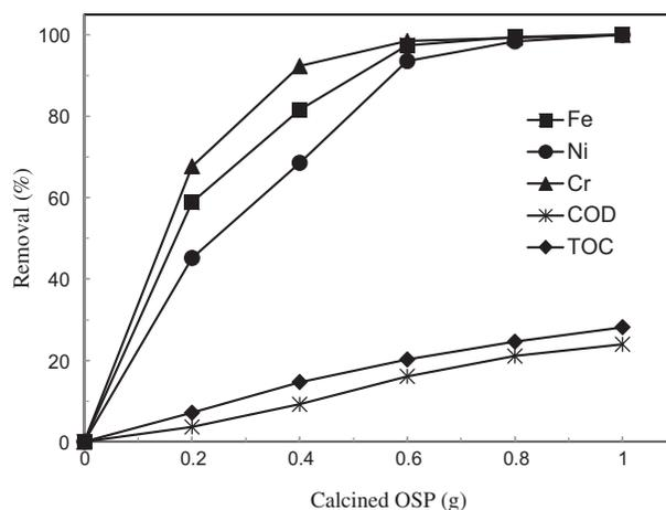
Fig. 3. Effect of calcined OSP dose on removing organics and heavy metals.
