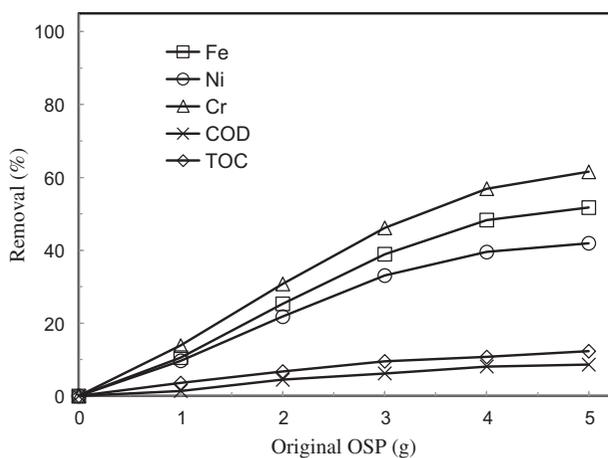
Fig. 2. Effect of original OSP dose on removing organics and heavy metals.
