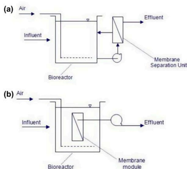
Fig. 1. Schematic configurations of (a) external MBR and (b) submerged MBR.
