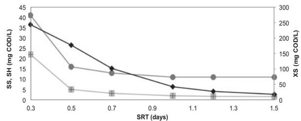
Fig. 6. Removal potential of different COD fractions in sewage as a function of sludge age—■  $S_5$ : readily biodegradable substrate, ●  $S_H$ : readily hydrolysable substrate ◆  $X_5$ : slowly biodegradable substrate.
