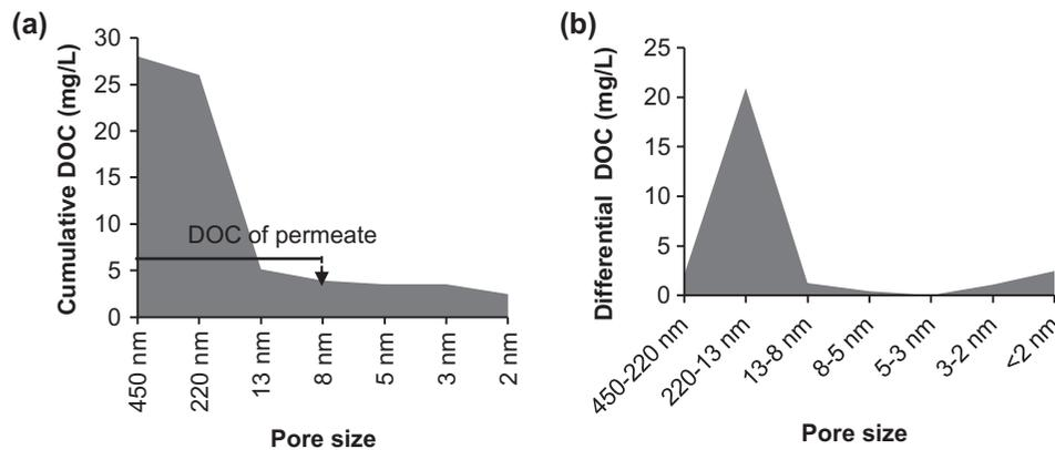
Fig. 5. (a) Cumulative and (b) differential PSD profiles of DOC in the reactor volume for SRT of 0.5 d.
