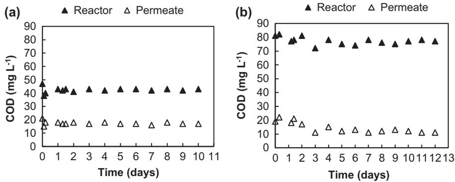
Fig. 3. Observed COD profiles at steady state for an HRT of 1.0 h and (a) SRT of 0.5 d and (b) SRT of 2.0 d [107].
