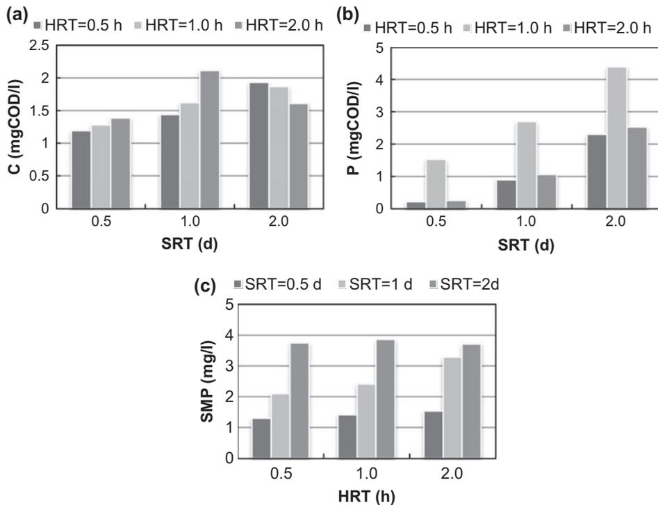
Fig. 4. Generation of (a) carbohydrates, (b) proteins, and (c) SMPs as a function of SRT [107].
