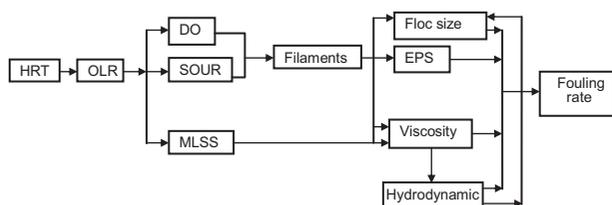
Fig. 2. Schematic relationship of HRT with sludge characteristics and membrane performance [57].
