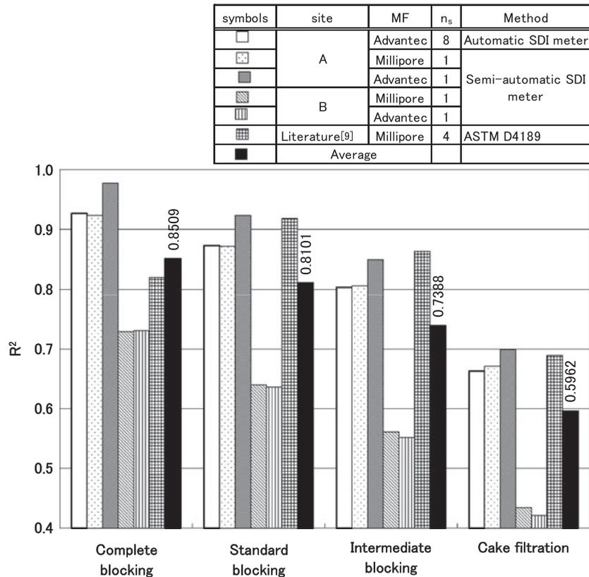
Fig. 9. Comparison of the goodness of fit between measured SDI and calculated SDI in different sample temperatures by the coefficient of determination  $R^2$  (filtered seawater after pretreatment).
