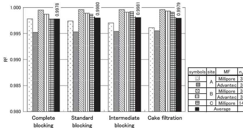
Fig. 5. Comparison of the goodness of fit between the measured filtration curves and calculated filtration curves by the coefficient of determination  $R^2$  (filtered seawater after pretreatment at site A, B, and C).
