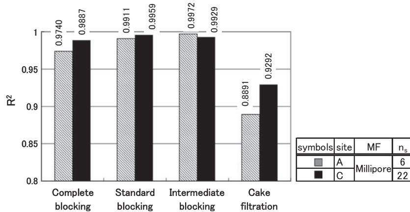
Fig. 3. Comparison of the goodness of fit between the measured filtration curves and calculated filtration curves by the coefficient of determination  $R^2$  (raw seawater at site A and site C).
