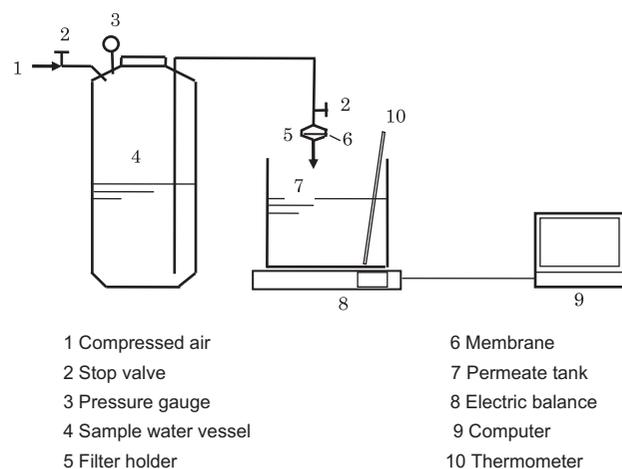
Fig. 1. Schematic diagram of filtration system for the measurements of filtration curve and SDI.
