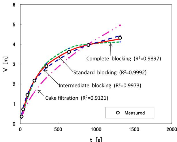
Fig. 2. Typical comparative example of the measured filtration curve and the calculated filtration curves by each filtration model (raw seawater at site A).
