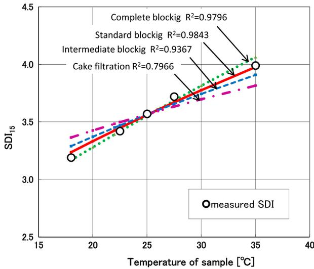
Fig. 8. Typical comparative example of measured SDI and calculated SDI of each model at different temperature (filtered seawater after pretreatment at site A).
