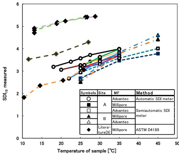
Fig. 6. Results of SDI measurements at different sample temperature (symbols tied with the line represent the same sample).
