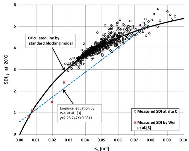
Fig. 11. Relationship between  $k_s$  and SDI (filtered seawater after pretreatment at site C).
