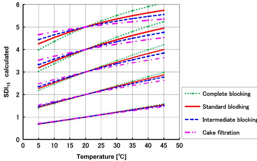
Fig. 7. Theoretical evaluation of the temperature effect on SDI by each filtration model.
