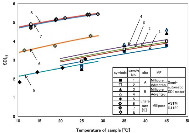
Fig. 10. Comparison between measured SDI and calculated SDI (solid lines represent the calculated lines by standard blocking model).
