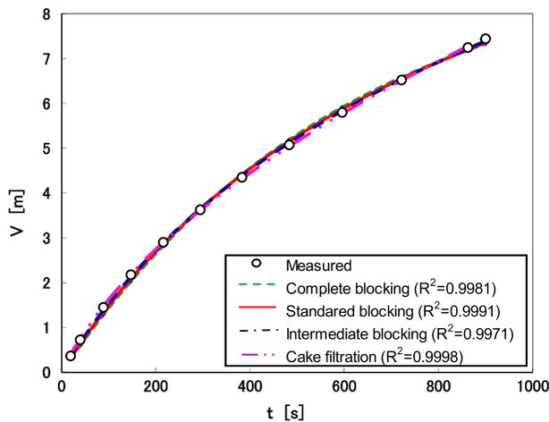
Fig. 4. Typical comparative example of measured filtration curve and calculated filtration curves by each filtration model (filtered seawater after pretreatment at site C).
