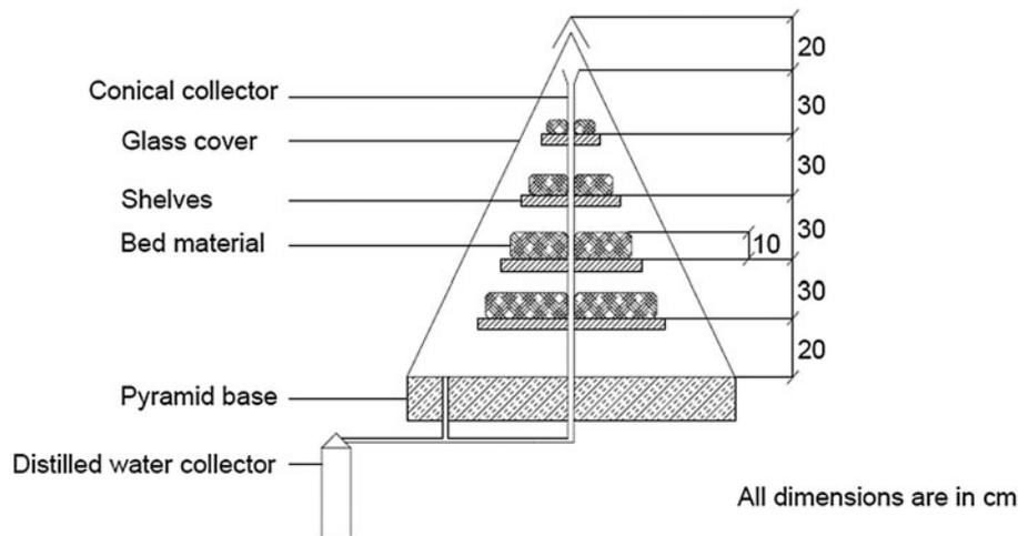
Fig. 16. Schematic diagram of pyramidal multi shelf solar still [37].
