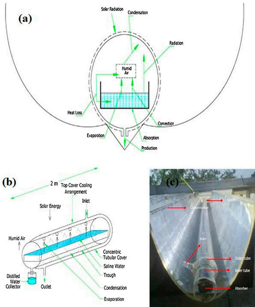
Fig. 14. Schematic diagram of concentric tubular solar still (a) Cross-section, (b) 3D View, and (c) Experimental photograph of concentric tubular solar still [34].
