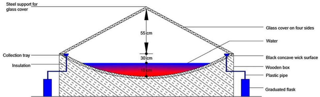
Fig. 1. Schematic diagram of a concave solar still with wick [13].
