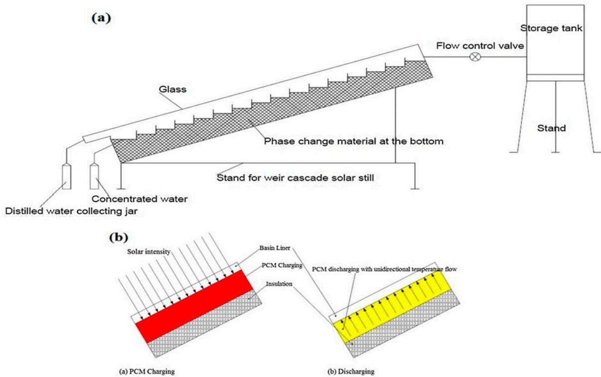
Fig. 8. Schematic diagram of (a) weir cascaded solar still with PCM [20] and (b) heat flow from PCM in charging and discharging modes.
