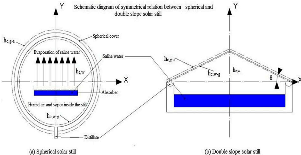
Fig. 12. Mode of heat transfer and condensation in (a) spherical and (b) double slope solar still with axis symmetry.
