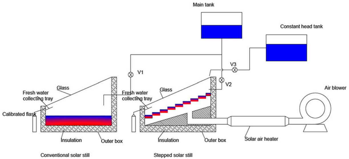
Fig. 6. Sectional view of a stepped solar still with solar air heater [18].
