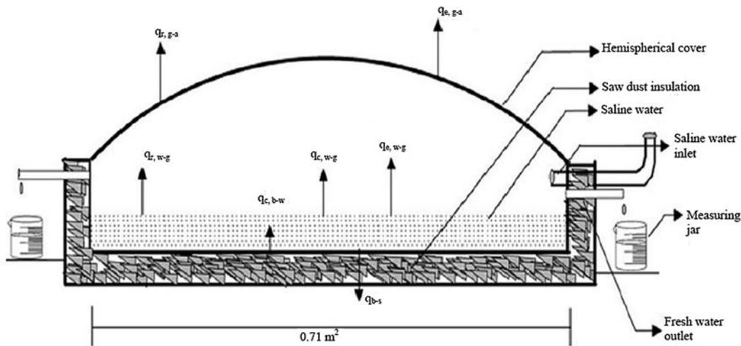
Fig. 9. Schematic diagram of a hemispherical cover solar still [22].
