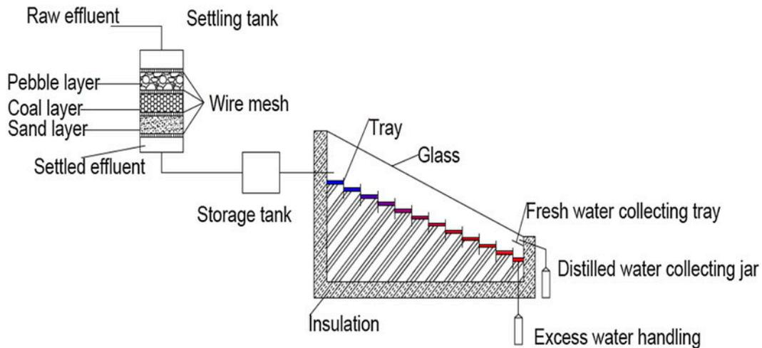
Fig. 5. Schematic diagram of a stepped solar still integrated to solar pond [17].
