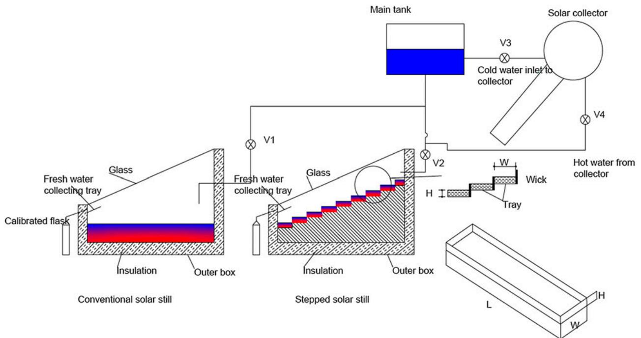
Fig. 2. Schematic diagram of a stepped solar still with wick as absorbing material [14].
