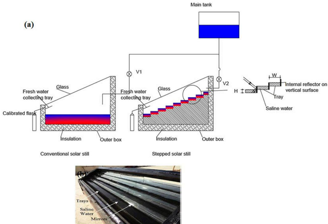
Fig. 4. (a) Schematic diagram of a stepped solar still with reflectors (internal) and (b) experimental picture of a solar still with reflectors (internal) [16].
