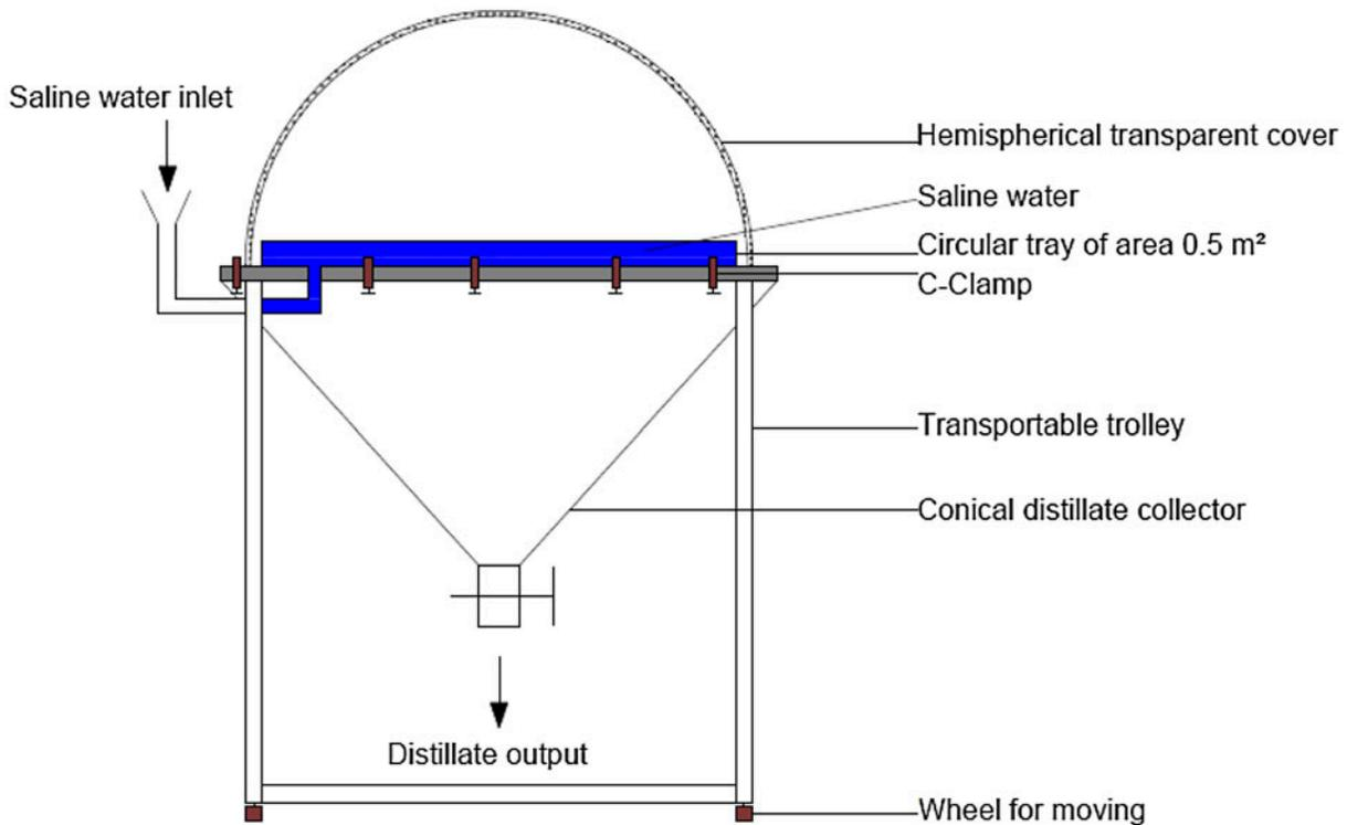
Fig. 10. Schematic diagram of a transportable hemispherical cover solar still [23].
