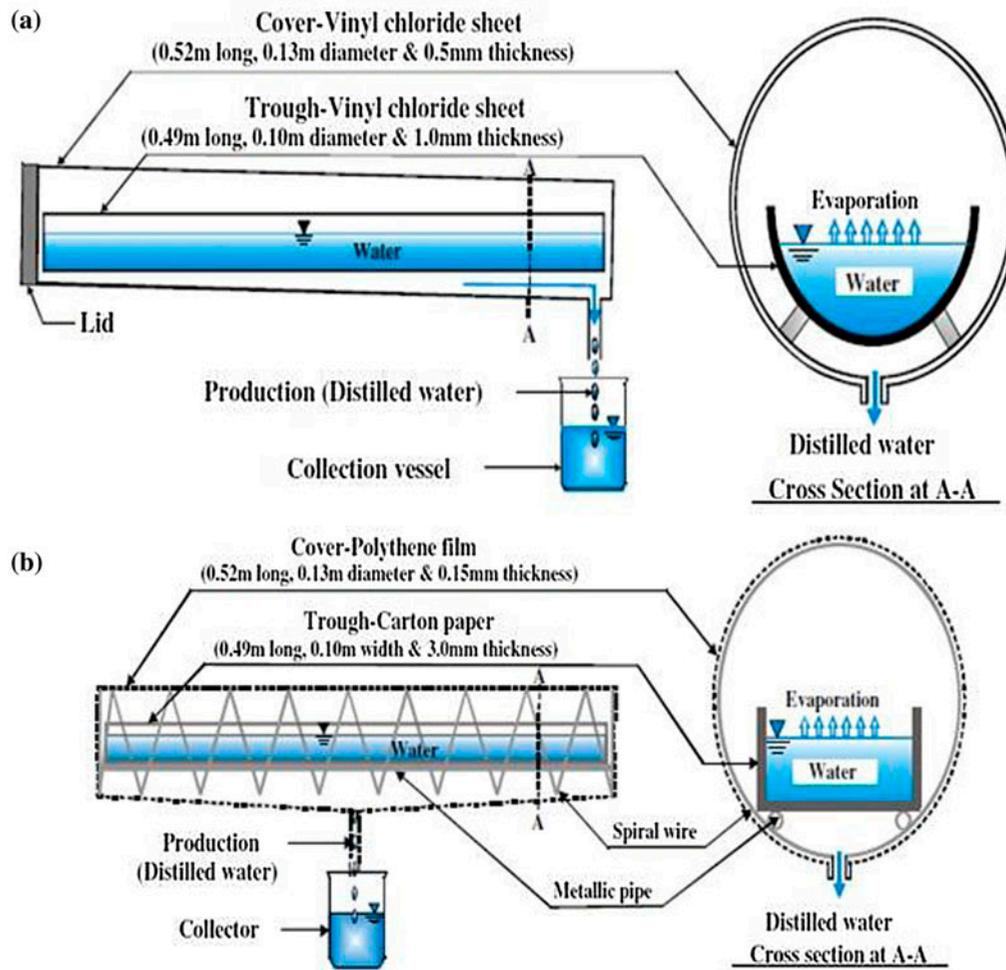
Fig. 13. Schematic diagram of a tubular solar still (a) semicircular trough (b) rectangular trough [29].
