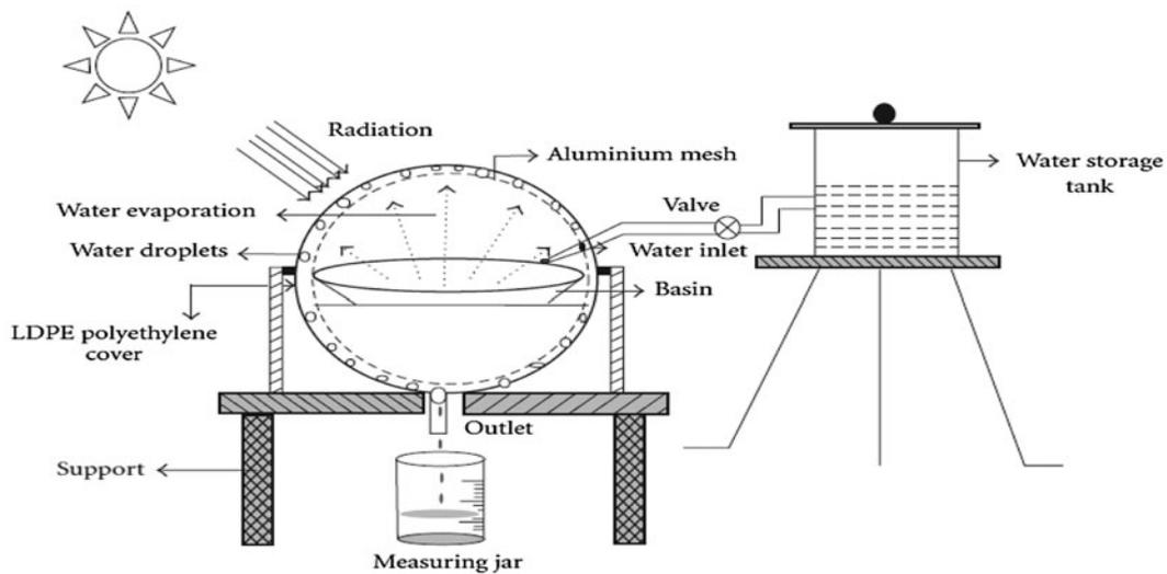
Fig. 11. Schematic diagram of a spherical solar still [24].
