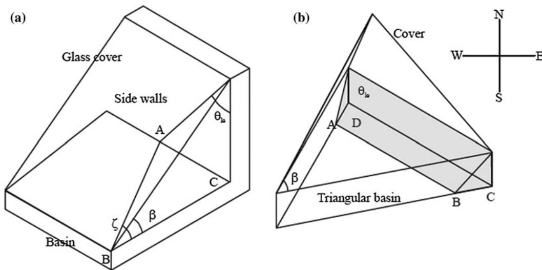
Fig. 17. Schematic diagram of a triangular pyramid solar still [39].
