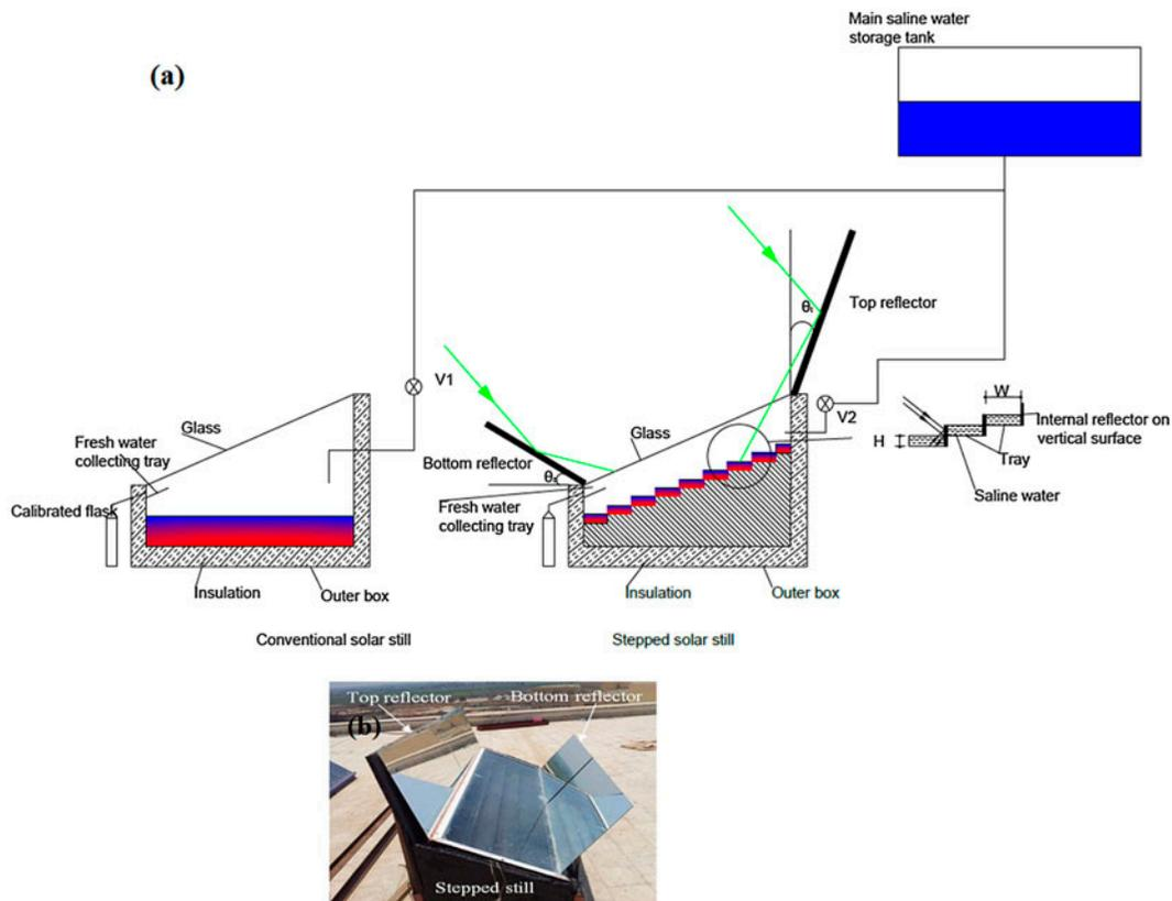
Fig. 3. (a) Schematic diagram of a stepped solar still with reflectors (Internal and External) and (b) experimental picture of a solar still with reflector (internal and external) [15].
