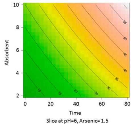
Fig. 5. Contour plots for the effect of time and adsorbent dosage on arsenic adsorption using MMT. Values on contour plots represent arsenic removal (%).
