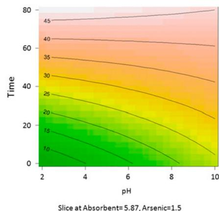
Fig. 2. Contour plots for the effect of pH and time on arsenic adsorption using MMT. Values on contour plots represent arsenic removal (%).
