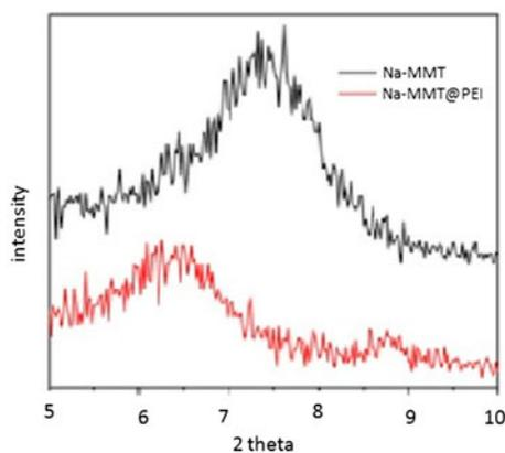
Fig. 1. X-ray diffraction patterns of MMT and MMT@PEI.
