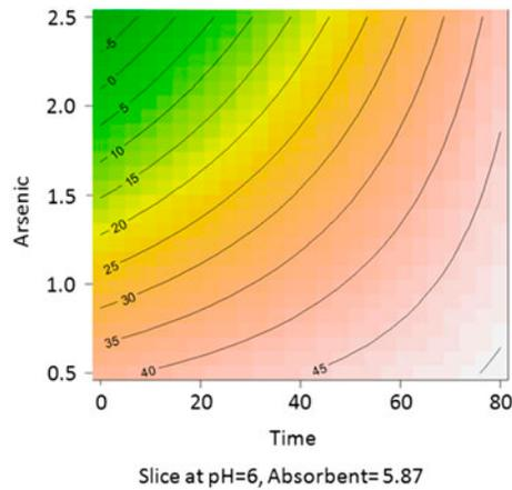
Fig. 6. Contour plots for the effect of time and arsenic concentration on arsenic adsorption using MMT. Values on contour plots represent arsenic removal (%).
