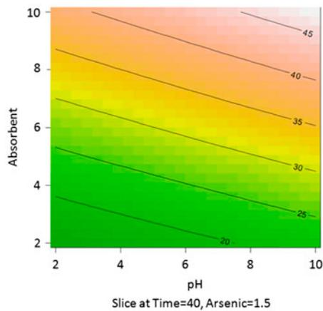
Fig. 3. Contour plots for the effect of pH and adsorbent dosage on arsenic adsorption using MMT. Values on contour plots represent arsenic removal (%).
