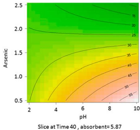
Fig. 4. Contour plots for the effect of pH and arsenic concentration on arsenic adsorption using MMT. Values on contour plots represent arsenic removal (%).
