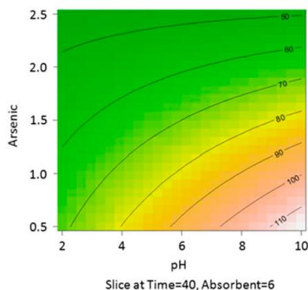
Fig. 8. Contour plots for the effect of pH and arsenic concentration on arsenic adsorption using MMT@PEI. Values on contour plots represent arsenic removal (%).
