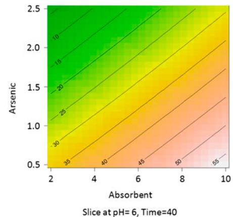
Fig. 7. Contour plots for the effect of adsorbent dosage and arsenic concentration on arsenic adsorption using MMT. Values on contour plots represent arsenic removal (%).
