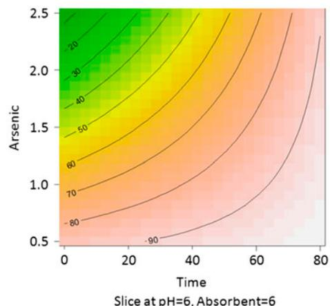
Fig. 9. Contour plots for the effect of time and arsenic concentration on arsenic adsorption using MMT@PEI. Values on contour plots represent arsenic removal (%).
