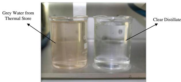
Fig. 12. Samples of gray water and clear distillate.
