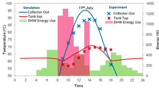
Fig. 10. DHW temperature and energy profile.
