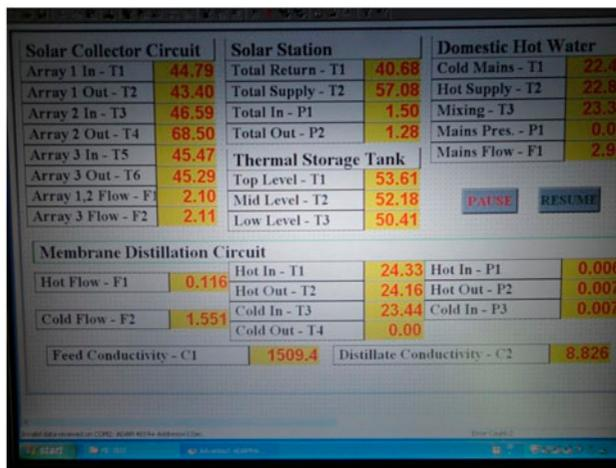
Fig. 11. Data acquisition interface of SDHW-MD system.
