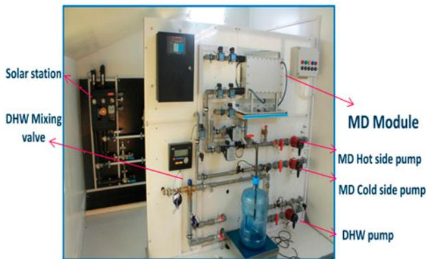
Fig. 6. MD system with solar station.
