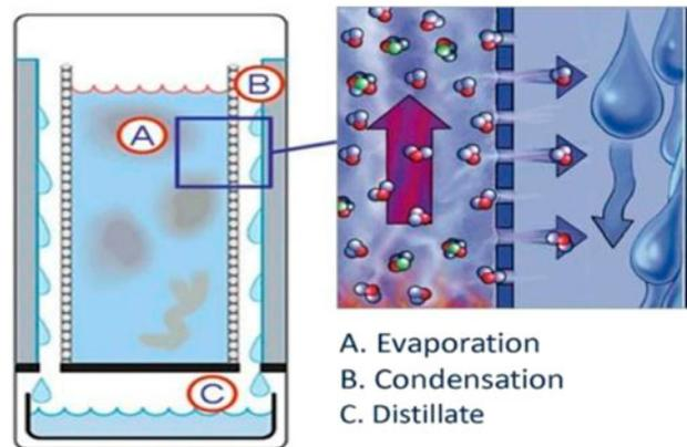
Fig. 2. AGMD technique (image on right-hand side courtesy of Scarab development AB).
