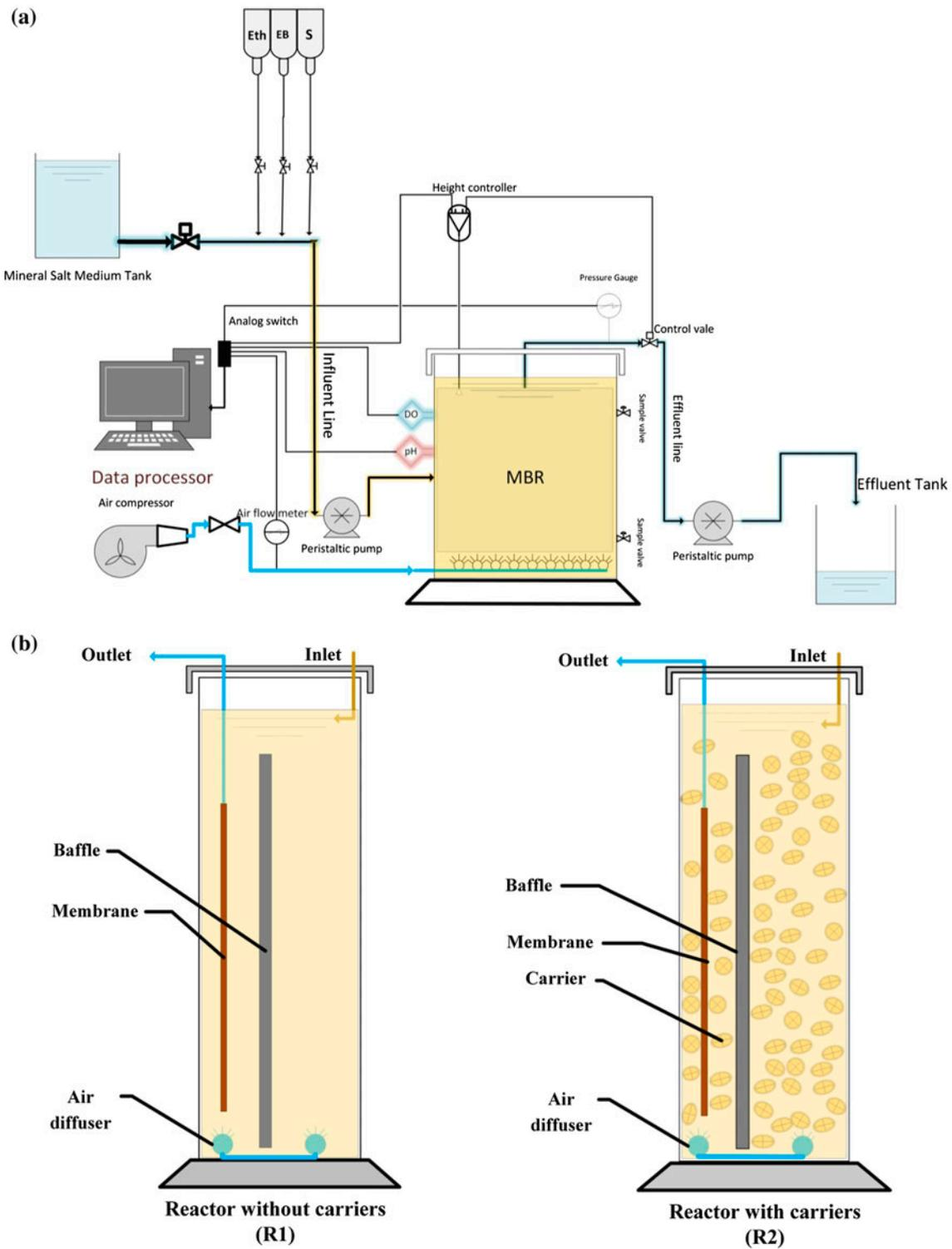
Fig. 1. (a) Schematic process flow diagram and (b) side view of the two reactors.
