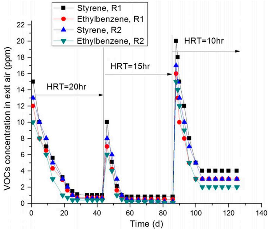
Fig. 3. Ethylbenzene and styrene concentration in the exit air during the operation of the MBRs HRT of 20 h (days 0–43rd), 15 h (days 44–85th), and 10 h (days 86–125th).
