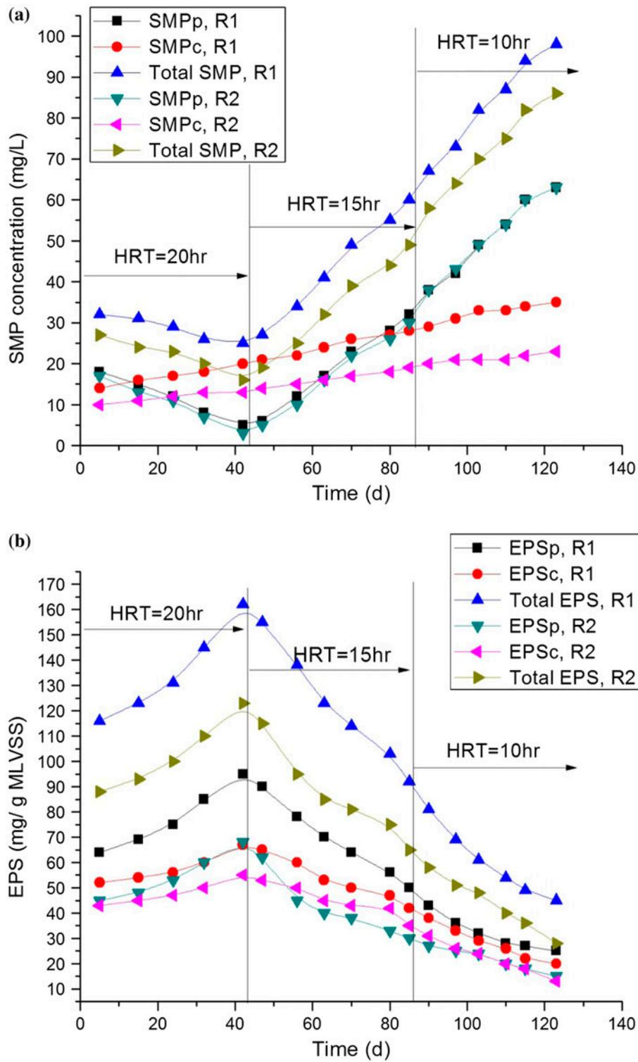
Fig. 6. (a) Variation of SMP, SMP<sub>p</sub>, and SMP<sub>c</sub> concentration and (b) variation of EPS, EPS<sub>p</sub>, and EPS<sub>c</sub> concentration during the operation of the MBRs.
