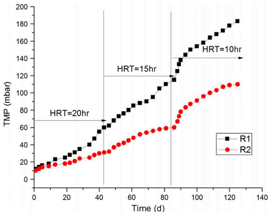
Fig. 5. Variations of TMP during operation HRT of 20 h (days 0–43rd), 15 h (days 44–85th), and 10 h (days 86–125th).
