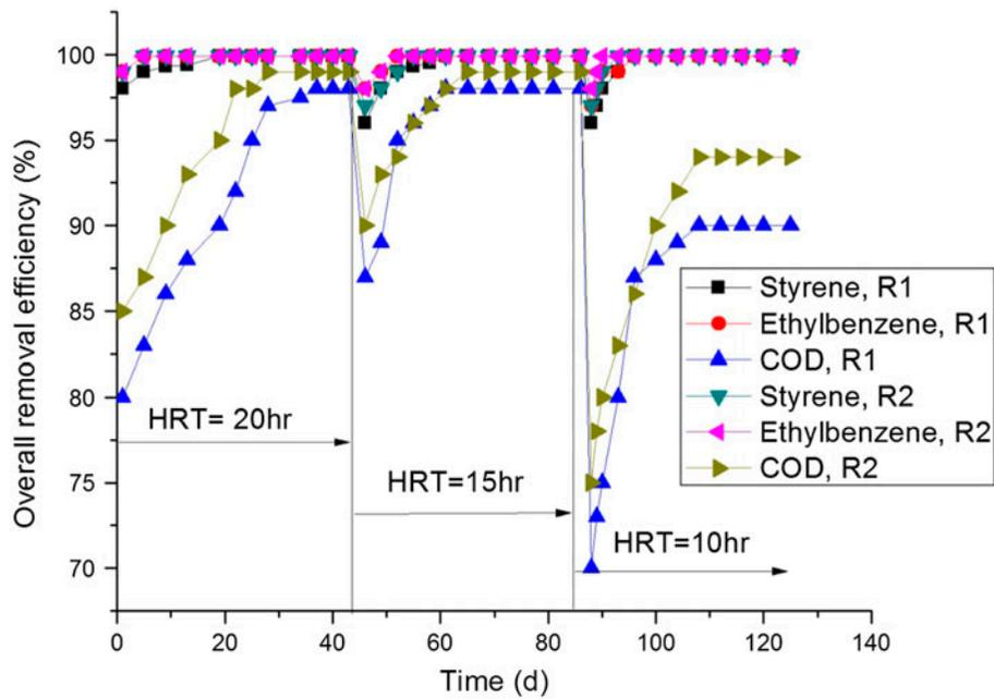
Fig. 2. Variations of COD, styrene, and ethylbenzene removal during the operation of the MBRs HRT of 20 h (days 0–43rd), 15 h (days 44–85th), and 10 h (days 86–125th).
