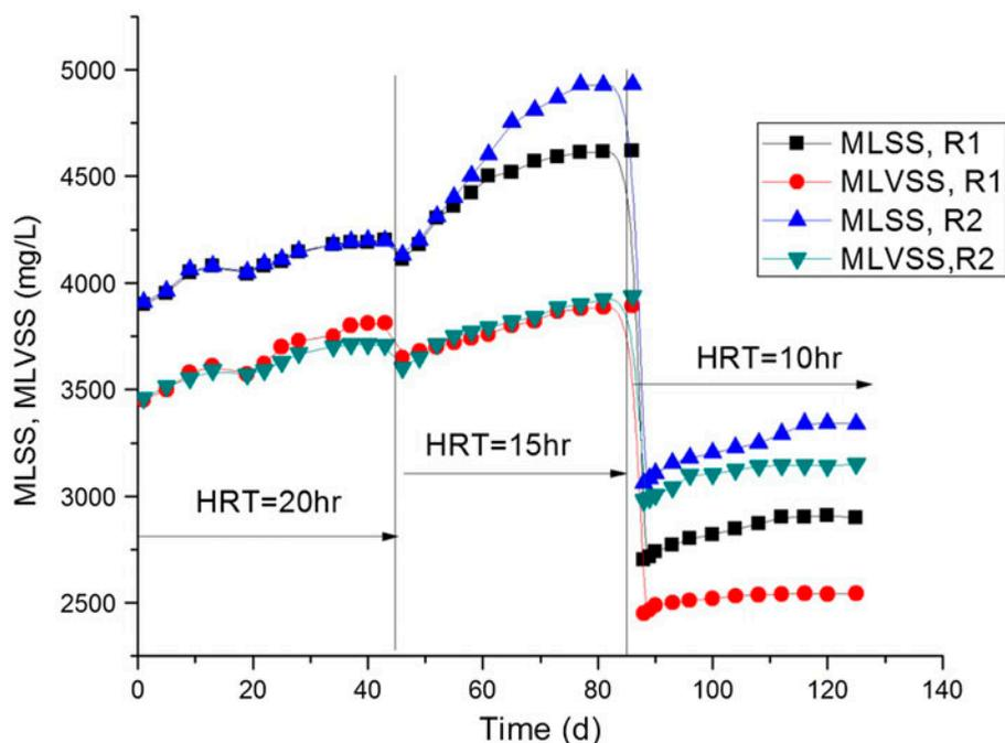
Fig. 4. Variations of MLSS and MLVSS during the operation of the MBRs HRT of 20 h (days 0–43rd), 15 h (days 44–85th), and 10 h (days 86–125th).
