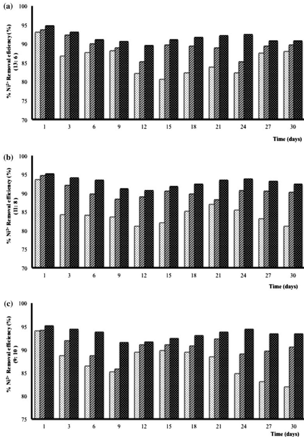
Fig. 4.  $\text{Ni}^{2+}$  removal efficiency profiles of the SBR system operated with SIWW +  $\text{Ni}^{2+}$  at various ox:an ratios in the reaction step. (a) 13:6, (b) 11:8, and (c) 9:10. Symbols: □: anoxic 1, ▨: oxic 1, ■: settle.
