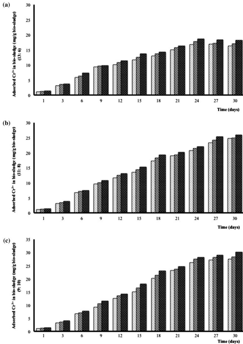
Fig. 7.  $Cr^{3+}$  profile of bio-sludge in the SBR system operated with SIWW +  $Cr^{3+}$  at various oxidic:anoxic ratios in the reaction step: (a) 13:6, (b) 11:8, and (c) 9:10. Symbols: □: anoxic, ▨: oxidic, and ■: settle.
