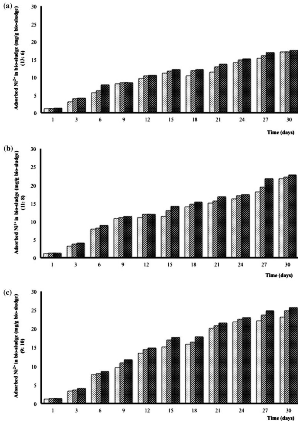
Fig. 6.  $\text{Ni}^{2+}$  profile of bio-sludge in the SBR system operated with SIWW +  $\text{Ni}^{2+}$  at various oxo:anoxic ratios in the reaction step. (a) 13:6, (b) 11:8, and (c) 9:10. Symbols: □: anoxic 1, ▨: oxic 1, and ■: settle.
