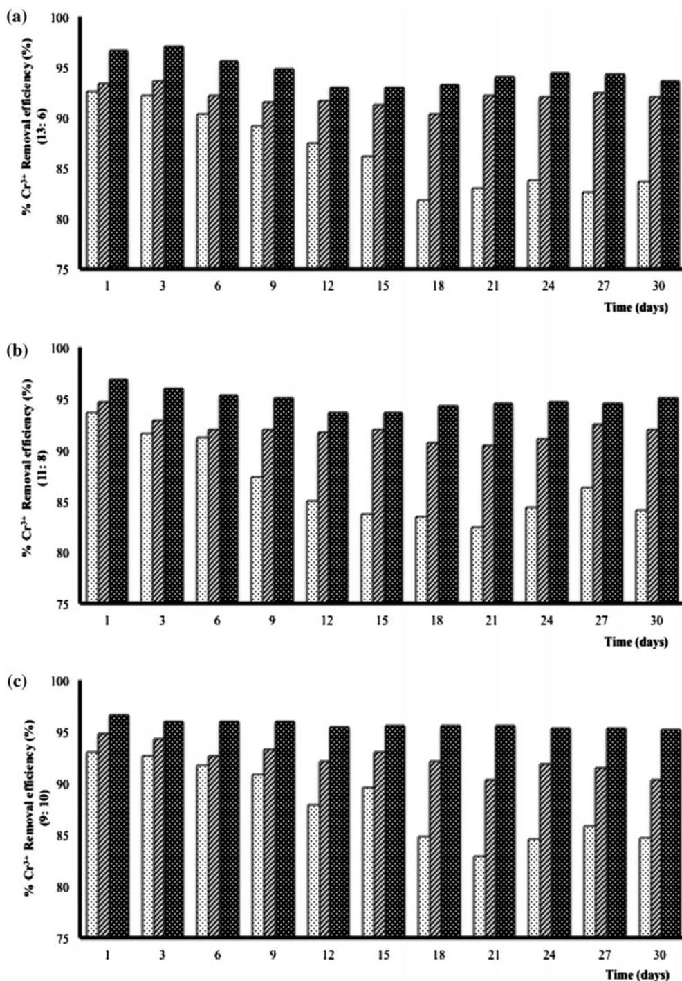
Fig. 5. Cr<sup>3+</sup> removal efficiency profiles of the SBR system operated with SIWW + Cr<sup>3+</sup> at various oxo:anoxic ratios in the reaction step. (a) 13:6, (b) 11:8, and (c) 9:10. Symbols: □: anoxic 1, ▨: oxic 1, and ■: settle.
