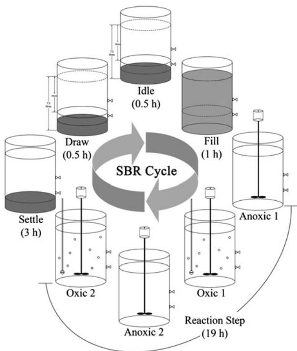
Fig. 2. Flow diagram of the SBR treatment system operation steps of each cycle.
