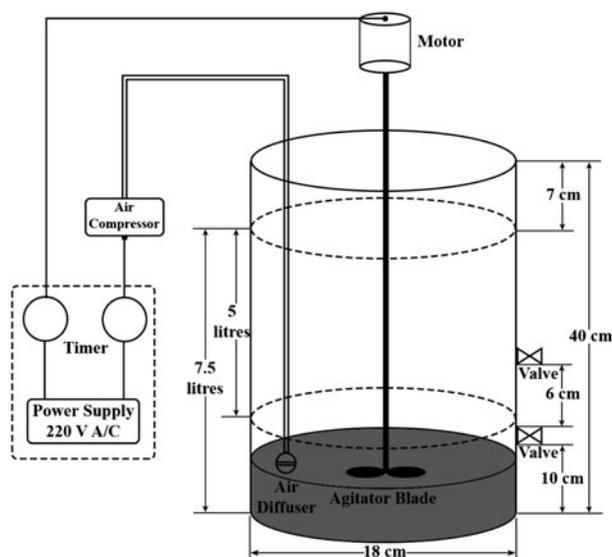
Fig. 1. Schematic diagram of SBR treatment system.
