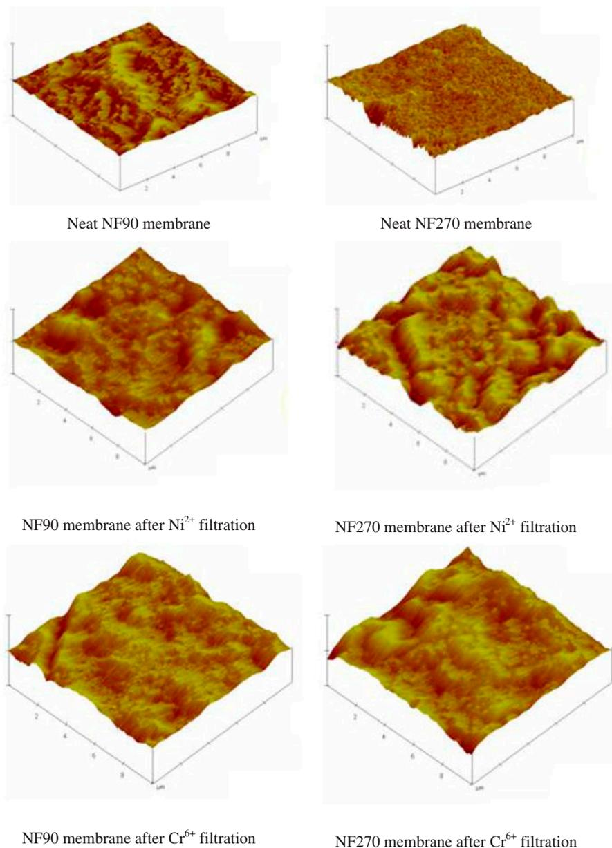
Fig. 11. AFM images of NF membranes before and after metal filtration.
