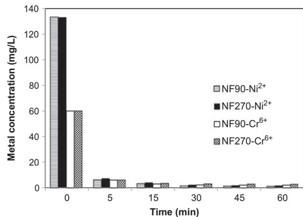
Fig. 10. Variation of metal concentration during NF process using NF90 and NF270 membranes at 30 bar and pH 10.
