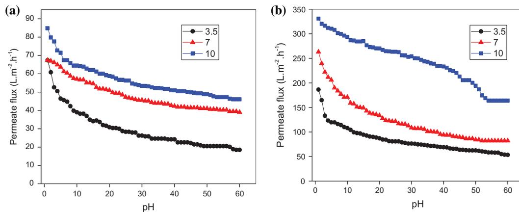
Fig. 8. Effect of pH on flux decline of (a)  $\text{Ni}^{2+}$  and (b)  $\text{Cr}^{6+}$  for NF270 ( $\text{Ni}^{2+}$  concentration of feed:  $133 \pm 5$  ppm;  $\text{Cr}^{6+}$  concentration of feed:  $60 \pm 3$  ppm; pressure: 30 bar; time: 120 min; temperature:  $25 \pm 1$  °C).
