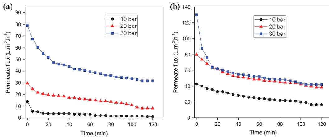
Fig. 4. Effects of pressure on flux decline of (a)  $\text{Ni}^{2+}$  and (b)  $\text{Cr}^{6+}$  for NF90 ( $\text{Ni}^{2+}$  concentration of feed:  $133 \pm 5$  ppm;  $\text{Cr}^{6+}$  concentration of feed:  $60 \pm 3$  ppm; pH 10; time: 120 min; temperature:  $25 \pm 1^\circ\text{C}$ ).
