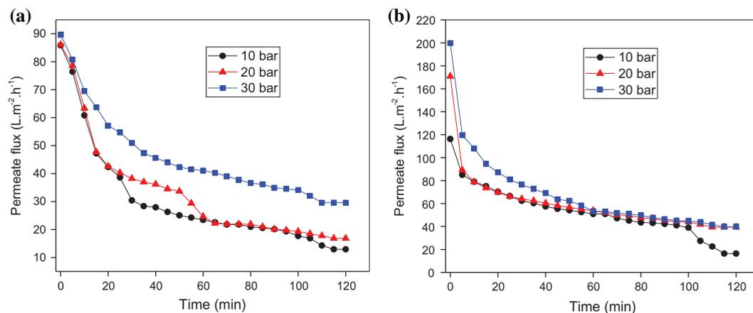
Fig. 5. Effects of pressure on flux decline of (a)  $\text{Ni}^{2+}$  and (b)  $\text{Cr}^{6+}$  for NF270 ( $\text{Ni}^{2+}$  concentration of feed:  $133 \pm 5$  ppm;  $\text{Cr}^{6+}$  concentration of feed:  $60 \pm 3$  ppm; pH 10; time: 120 min; temperature:  $25 \pm 1^\circ\text{C}$ ).
