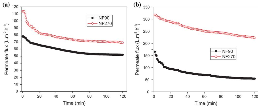
Fig. 9. Variation of flux decline as a function of time on rejection of (a)  $\text{Ni}^{2+}$  and (b)  $\text{Cr}^{6+}$  for NF90 and NF270 membranes ( $\text{Ni}^{2+}$  concentration of feed:  $133 \pm 5$  ppm;  $\text{Cr}^{6+}$  concentration of feed:  $60 \pm 3$  ppm; pressure: 30 bar; pH 10; time: 120 min; temperature:  $25 \pm 1$  °C).
