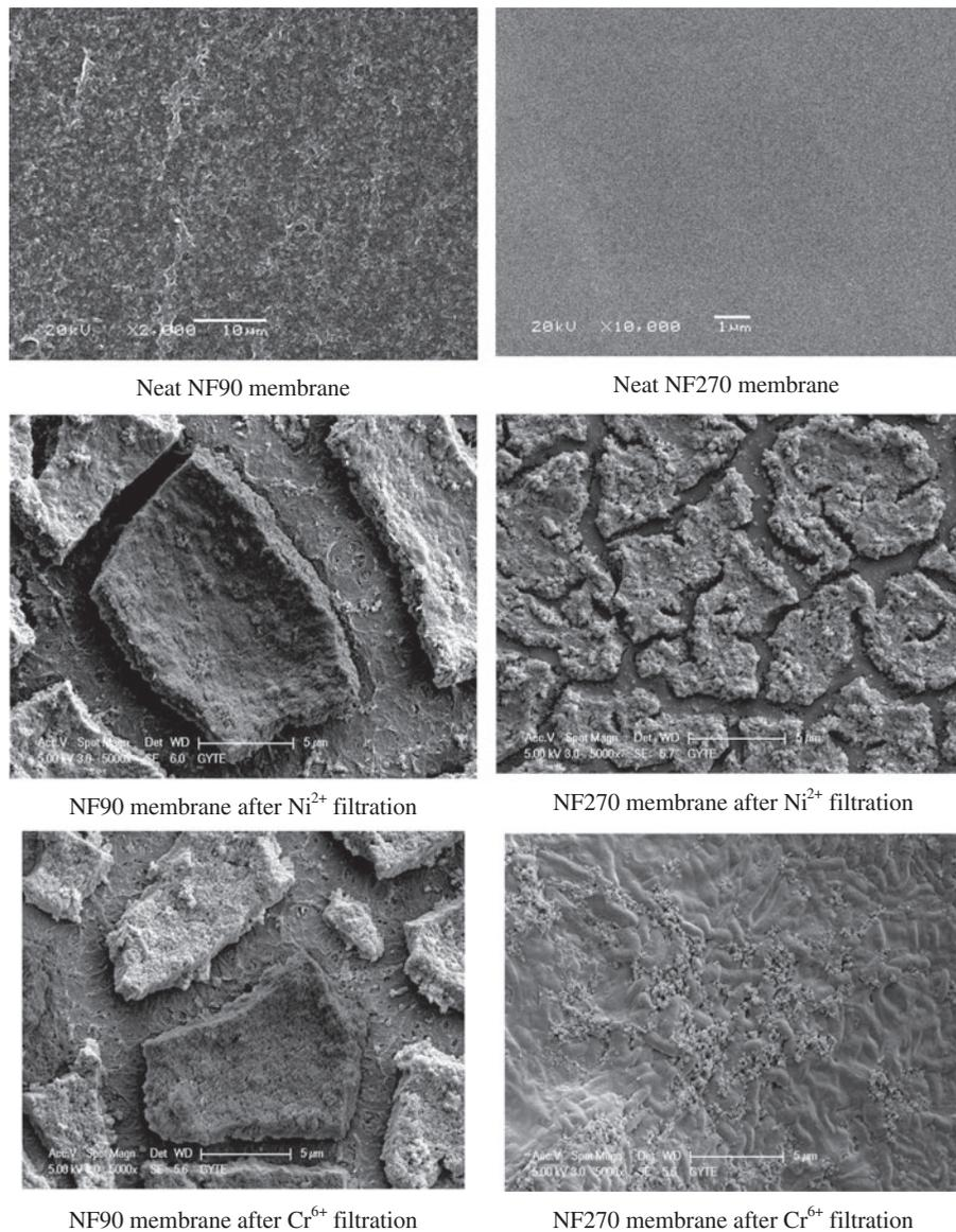
Fig. 12. SEM images of NF membranes before and after metal filtration.
