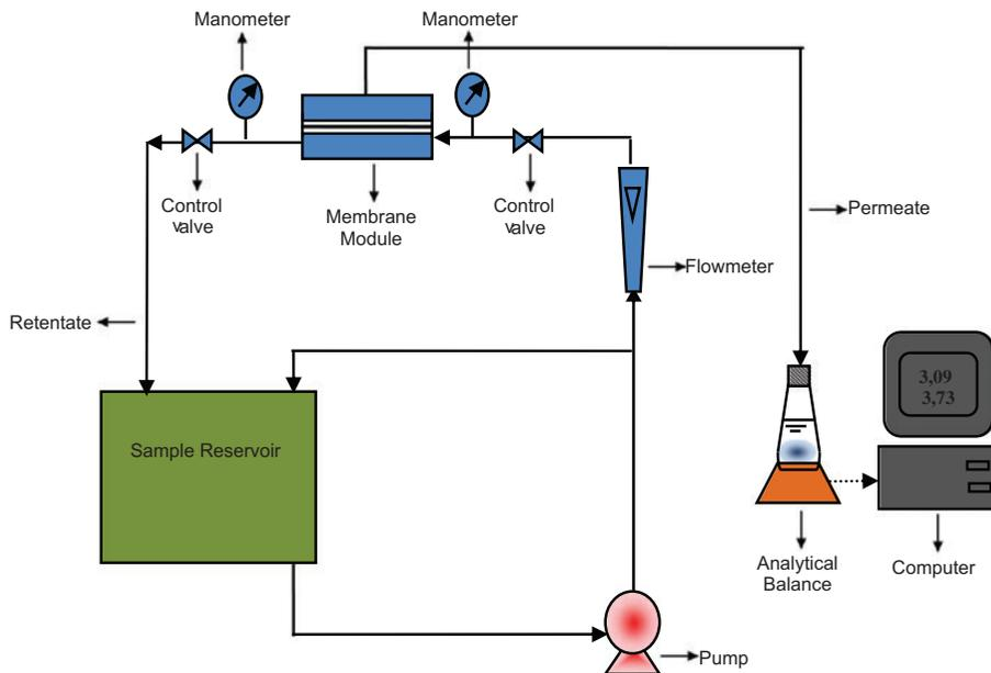
Fig. 2. Schematic diagram of the cross-flow NF experimental set-up.
