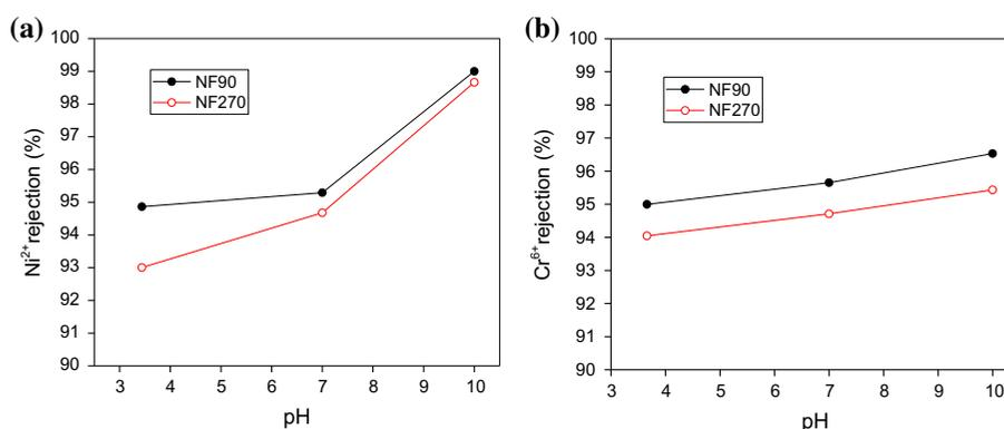
Fig. 6. Effect of pH on rejection of (a)  $\text{Ni}^{2+}$  and (b)  $\text{Cr}^{6+}$  for NF90 and NF270 membranes ( $\text{Ni}^{2+}$  concentration of feed:  $133 \pm 5$  ppm;  $\text{Cr}^{6+}$  concentration of feed:  $60 \pm 3$  ppm; pressure: 10 bar; time: 120 min; temperature:  $25 \pm 1^\circ\text{C}$ ).
