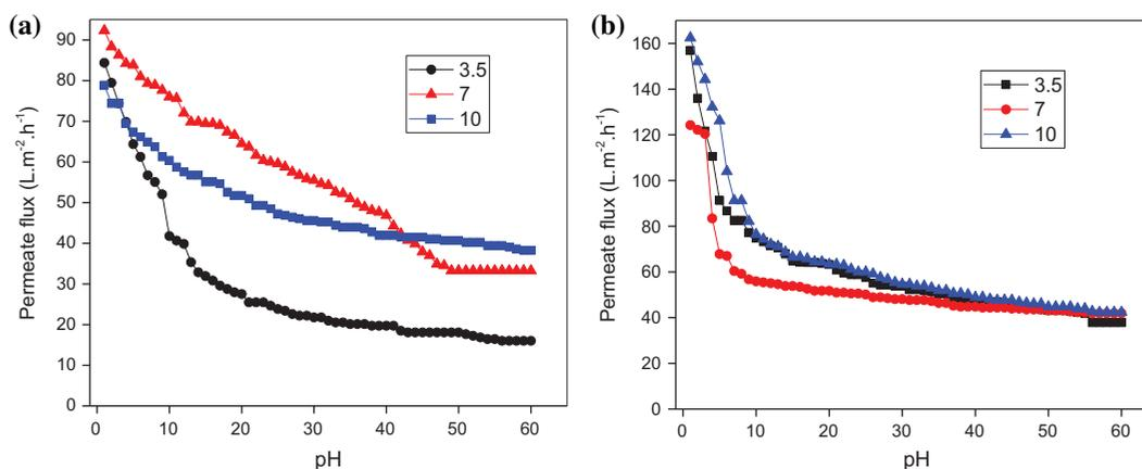
Fig. 7. Effect of pH on flux decline of (a)  $\text{Ni}^{2+}$  and (b)  $\text{Cr}^{6+}$  for NF90 ( $\text{Ni}^{2+}$  concentration of feed:  $133 \pm 5$  ppm;  $\text{Cr}^{6+}$  concentration of feed:  $60 \pm 3$  ppm; pressure: 30 bar; time: 120 min; temperature:  $25 \pm 1^\circ\text{C}$ ).
