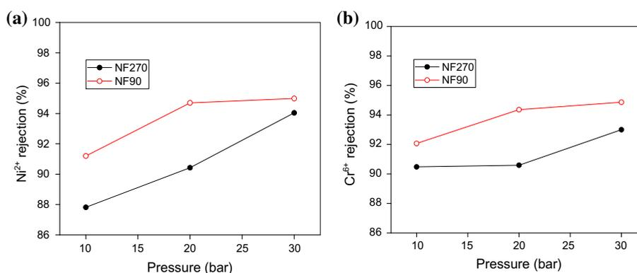
Fig. 3. Effects of pressure on rejection of (a) Ni<sup>2+</sup> and (b) Cr<sup>6+</sup> for NF90 and NF270 (Ni<sup>2+</sup> concentration of feed: 133 ± 5 ppm; Cr<sup>6+</sup> concentration of feed: 60 ± 3 ppm; pH 10; time: 120 min; temperature: 25 ± 1 °C).
