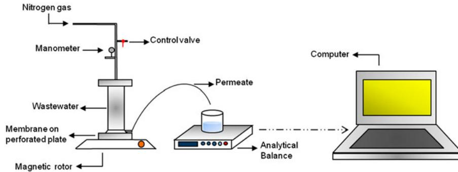
Fig. 1. Schematic diagram of the dead-end NF experimental set-up.
