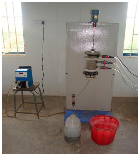
Fig. 1. Schematic diagram of the electrocoagulation (EC) reactors.
