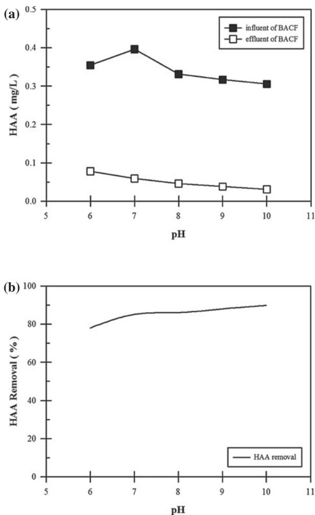
Fig. 1. Effect of pH on the removal of HAAs by BACF: the average concentrations are geometrical mean values of triplicate measurements (the operation conditions: temperature = 20.4°C, EBCT = 50 min). (a) Concentration of HAAs at different pH between influent and effluent of BACF and (b) variation of HAAs removal at different pH by BACF.
