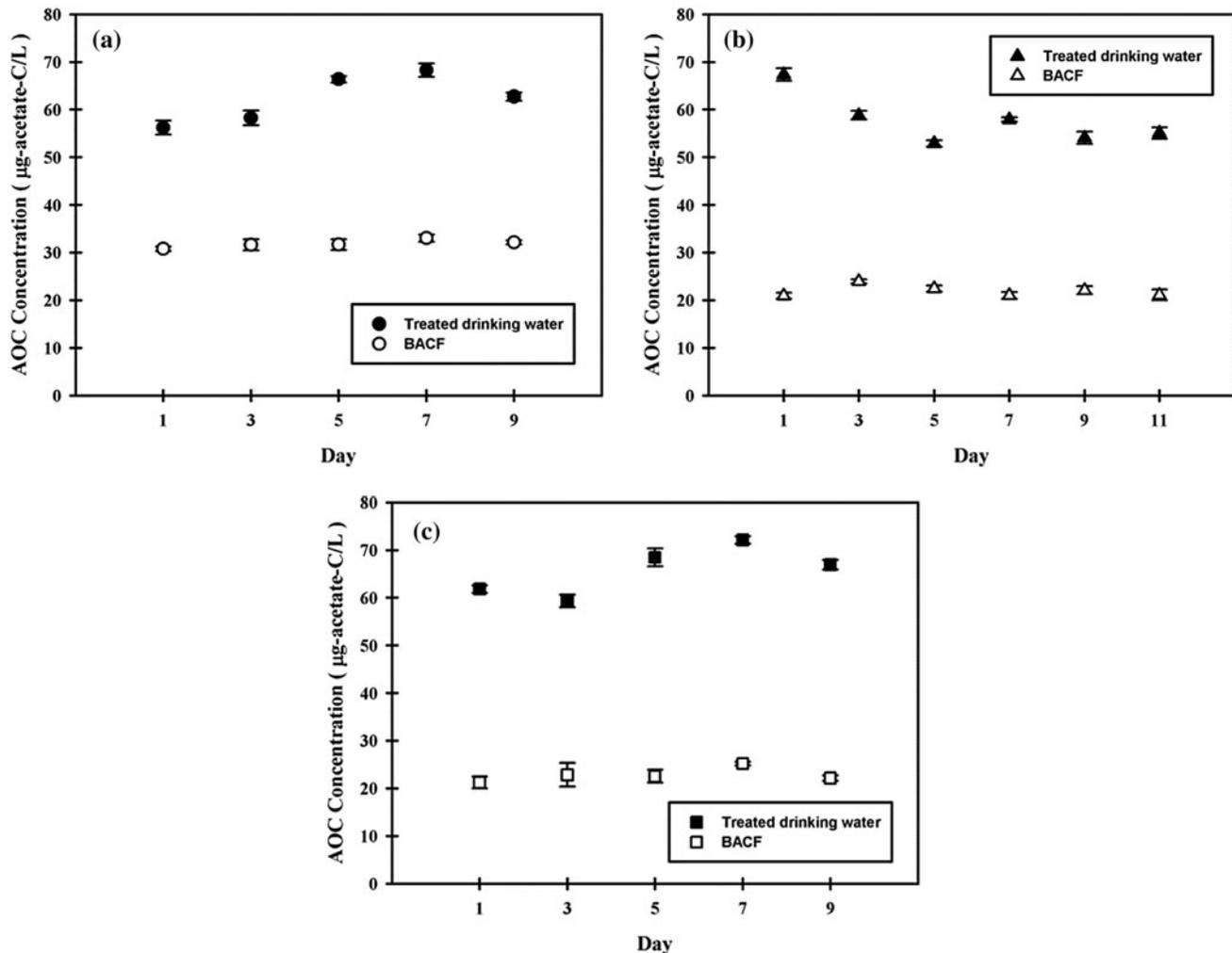
Fig. 4. Changes in concentration of AOC with respect to time by BACF under neutral conditions: (a) EBCT 30 min, (b) EBCT 40 min, and (c) EBCT 50 min. Influent conditions: temperature =  $24.0 \pm 2.0$  °C, pH  $7.2 \pm 0.1$ , and free residual chlorine =  $0.6 \pm 0.09$  mg/L. The average concentrations at all times are geometrical mean values of triplicate measurements, and the standard deviation was less than 5% for all data points.
