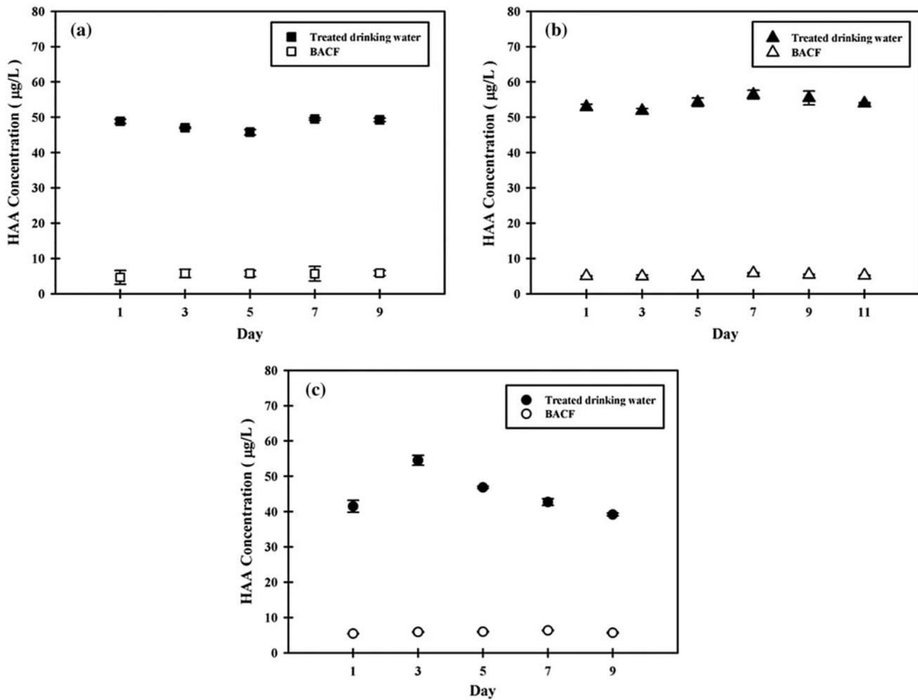
Fig. 2. Changes in concentration of haloacetic acids with respect to time by BACF at neutral conditions: (a) EBCT 30 min, (b) EBCT 40 min, and (c) EBCT 50 min. Error bars indicate the standard deviation from triplicate measurements.
