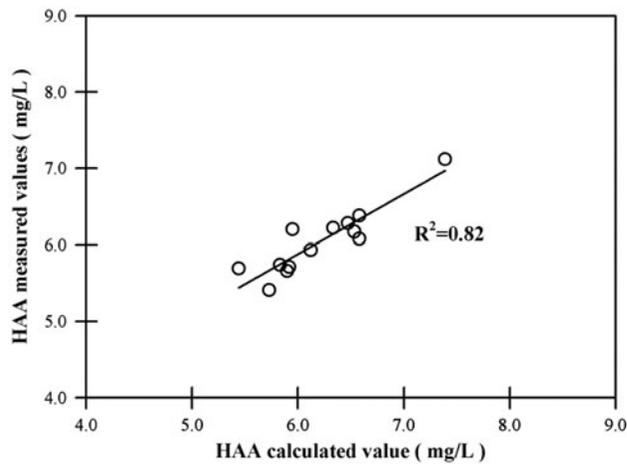
Fig. 3. Comparison between verified HAA5 values using Eq. (1) and the measured values in the effluent of BACF system. Errors were less than 5%.
