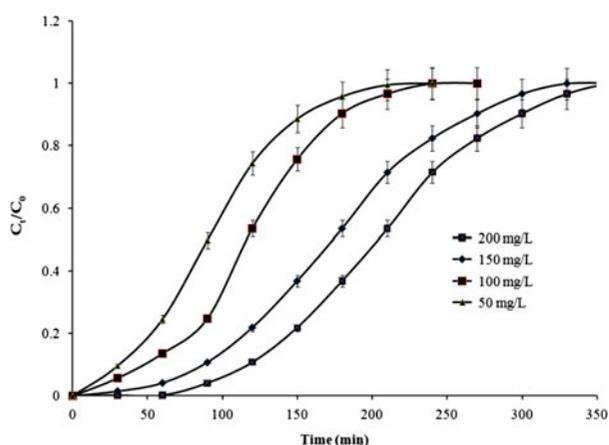
Fig. 3. Breakthrough curves for biosorption of MG by PLP at different initial dye concentration ( $m = 8$  g;  $Z = 5$  cm;  $F = 10$  mL min<sup>-1</sup>; pH 9.0; Temp. = 303 K).
