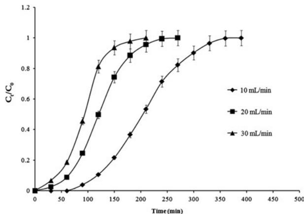
Fig. 1. Breakthrough curves for biosorption of MG by PLP at different feed flow rate ( $m = 8 \text{ g}$ ;  $Z = 5 \text{ cm}$ ;  $C_0 = 50 \text{ mg L}^{-1}$ ;  $\text{pH } 9.0$ ;  $\text{Temp.} = 303 \text{ K}$ ).
