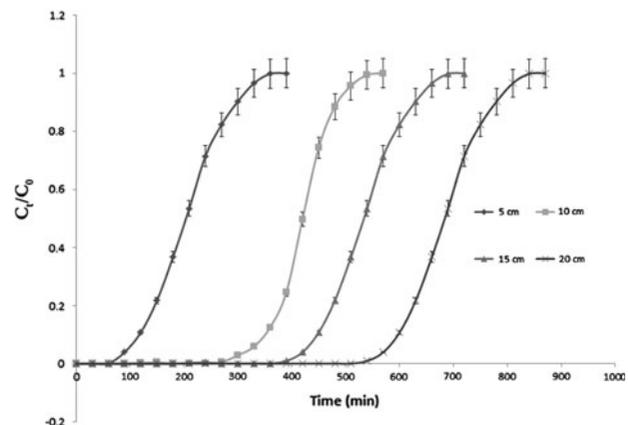
Fig. 2. Breakthrough curves for biosorption of MG by PLP at different bed heights ( $F = 10 \text{ mL min}^{-1}$ ;  $C_0 = 50 \text{ mg L}^{-1}$ ;  $\text{pH } 9.0$ ;  $\text{Temp.} = 303 \text{ K}$ ).
