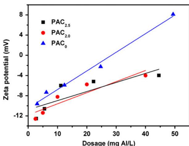
Fig. 5. Zeta potential of surface water after being treated by PAC.
