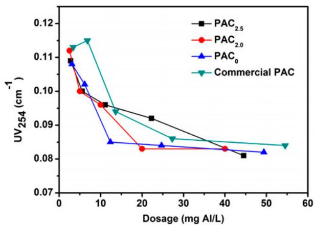
Fig. 2.  $UV_{254}$  of surface water after being treated by PAC.
