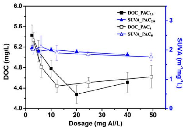
Fig. 3. DOC concentration and SUVA value of surface water after being treated by PAC<sub>2.0</sub> and PAC<sub>0</sub>.
