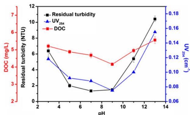
Fig. 6. Residual turbidity, UV<sub>254</sub>, and DOC concentration of surface water after being treated by moderate PAC<sub>2.0</sub> under the varied pH.
