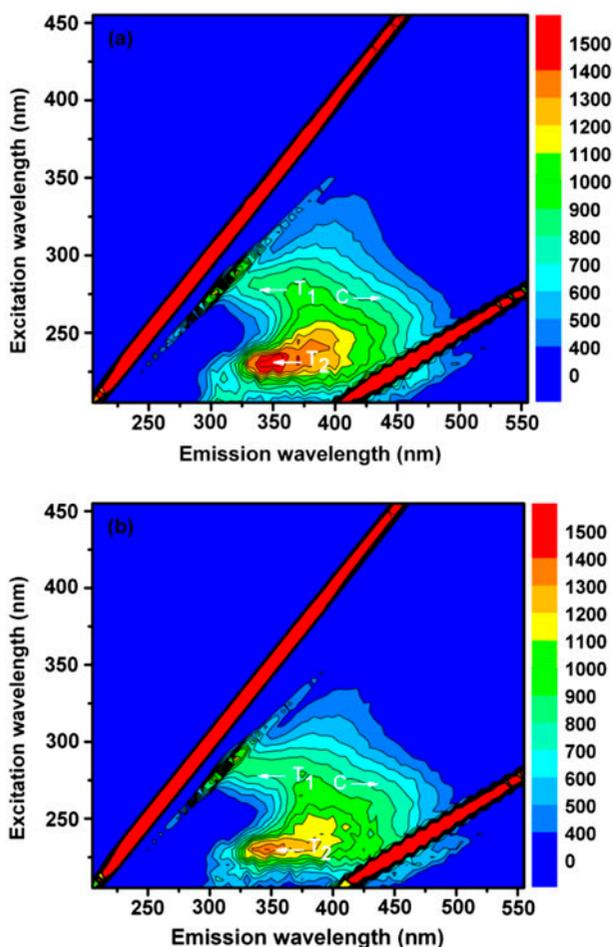
Fig. 4. FEEM spectra of surface water: (a) before and (b) after being treated by moderate  $PAC_{2.0}$ .
