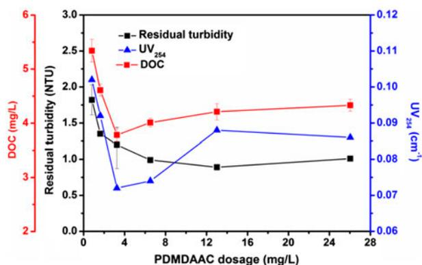
Fig. 7. Residual turbidity, UV<sub>254</sub>, and DOC concentration of surface water after being treated by a composite coagulant of PAC-PDMDAAC at pH 9.0.
