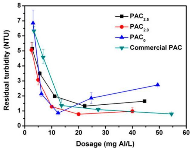
Fig. 1. Residual turbidity of surface water after being treated by PAC.
