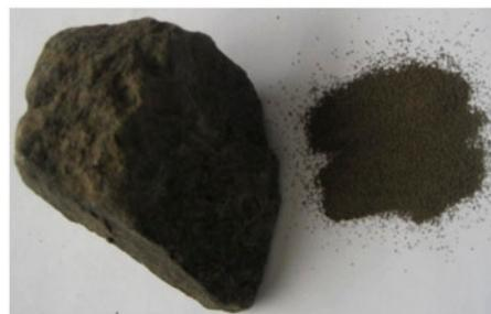
Fig. 1. Mineral waste from coal mining (MWCM).
