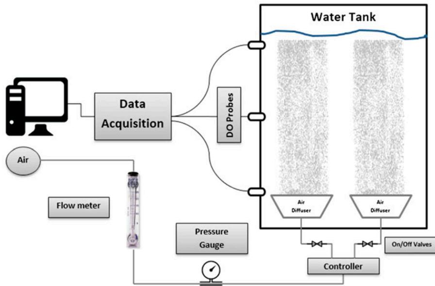
Fig. 1. DO measurement setup for real size aeration membranes.
