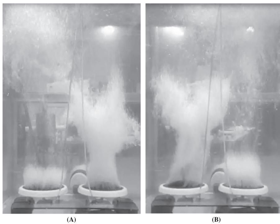
Fig. 5. On and off flow patterns (A) the right diffuser is on and the left is off, and (B) the left diffuser is on and the right is off.
