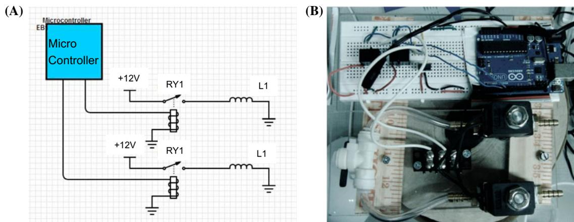
Fig. 2. (A) Circuit schematic diagram and (B) flow control circuit design layout.
