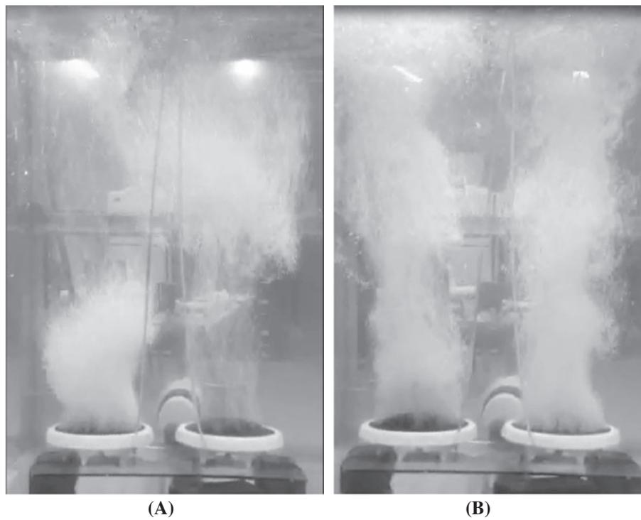
Fig. 4. Comparison between (A) pulsating flow and (B) steady state flow.
