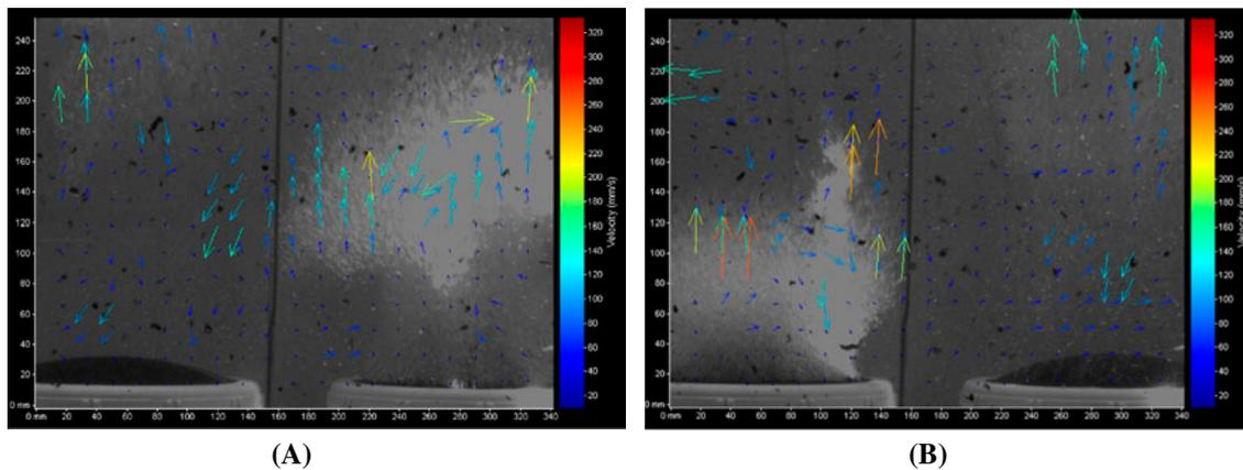
Fig. 6. Velocity vectors for pulsation flow system (A) the right diffuser is on and the left is off, and (B) the left diffuser is on and the right is off.
