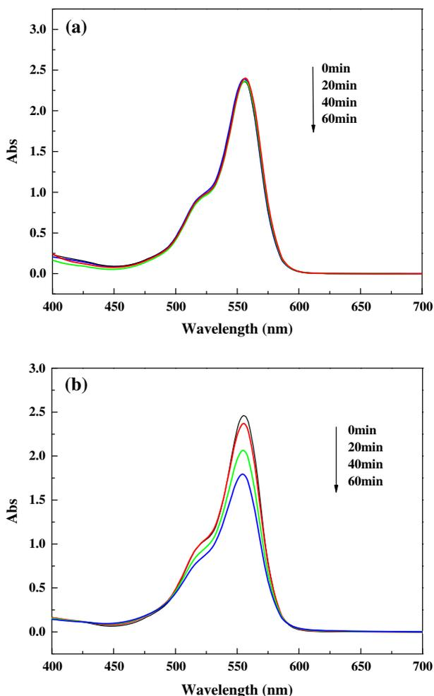
Fig. 3. UV-vis spectra of the complexation between Fe(III) and RhB: (a) dark and (b) xenon lamp irradiation. Experimental conditions: 0.052 mM [RhB]<sub>0</sub>, 1 mM [Fe<sup>3+</sup>]<sub>0</sub>, pH<sub>initial</sub> = 3.0.
