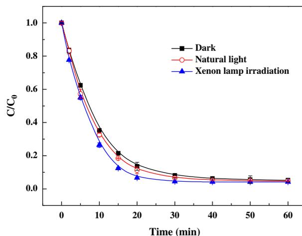
Fig. 2. Effect of different light environments on RhB degradation efficiencies. Experimental conditions: 0.052 mM [RhB]<sub>0</sub>, 1 mM [Fe<sup>3+</sup>]<sub>0</sub>, 1 mM [PS]<sub>0</sub>, pH<sub>initial</sub> = 3.0.
