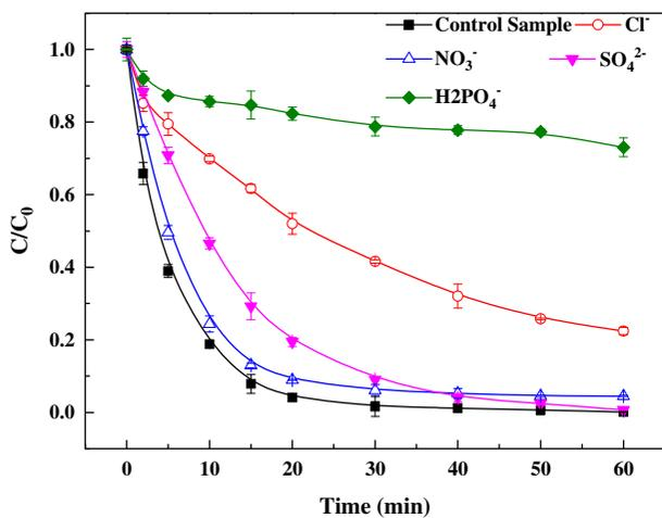
Fig. 6. Effect of different inorganic salts on RhB degradation efficiencies. Experimental conditions: 0.052 mM [RhB]<sub>0</sub>, 1 mM [Fe<sup>3+</sup>]<sub>0</sub>, 1 mM [PS]<sub>0</sub>, 1 mM [anion]<sub>0</sub>, pH<sub>initial</sub> = 3.0.
