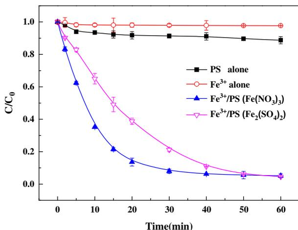
Fig. 1. Degradation of RhB under different reaction conditions. Experimental conditions: 0.052 mM [RhB]<sub>0</sub>, 1 mM [Fe<sup>3+</sup>]<sub>0</sub>, 1 mM [PS]<sub>0</sub>, pH<sub>initial</sub> = 3.0.
