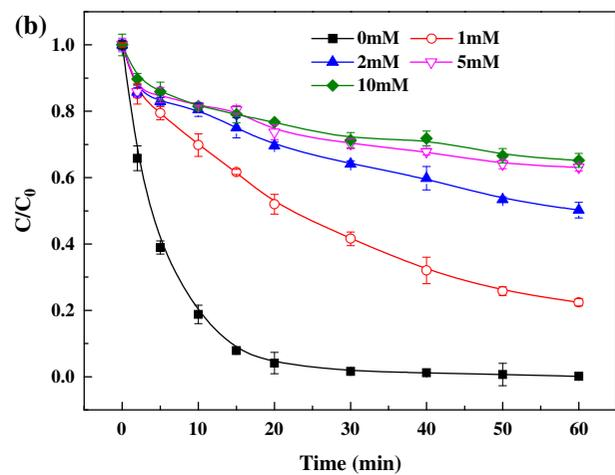
Fig. 7. Effects of different SO<sub>4</sub><sup>2-</sup> (a) and Cl<sup>-</sup> (b) concentrations on RhB degradation efficiencies. Experimental conditions: 0.052 mM [RhB]<sub>0</sub>, 1 mM [Fe<sup>3+</sup>]<sub>0</sub>, 1 mM [PS]<sub>0</sub>, pH<sub>initial</sub> = 3.0.
