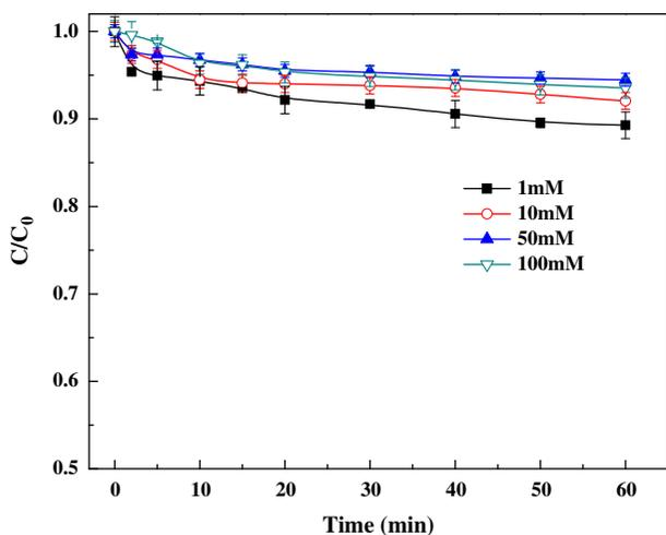
Fig. 8. RhB degradation efficiencies in the PS/Cl<sup>-</sup> system. Experimental conditions: 0.052 mM [RhB]<sub>0</sub>, 1 mM [Fe<sup>3+</sup>]<sub>0</sub>, 1 mM [PS]<sub>0</sub>, pH<sub>initial</sub> = 3.0.
