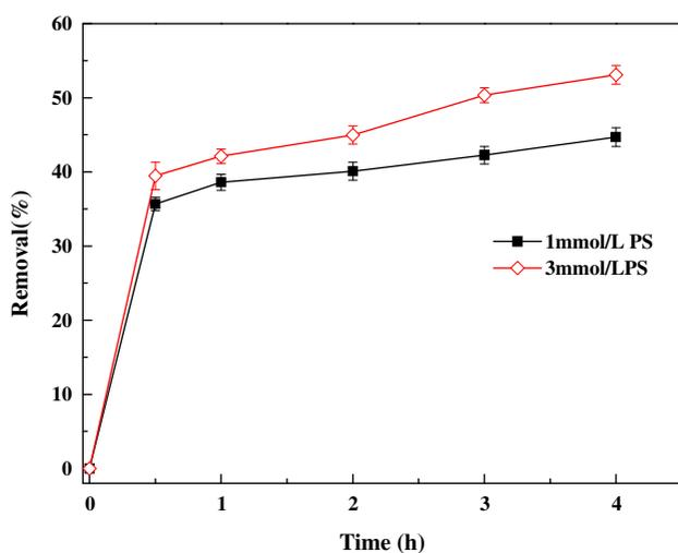
Fig. 9. TOC removal efficiencies of the RhB solution under different PS concentrations. Experimental conditions: 0.052 mM [RhB]<sub>0</sub>, 1 mM [Fe<sup>3+</sup>]<sub>0</sub>, pH<sub>initial</sub> = 3.0.
