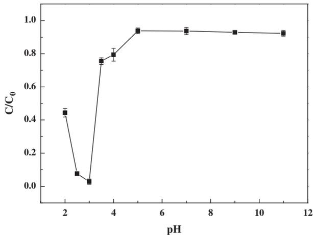
Fig. 5. Effect of initial pH on RhB degradation efficiencies in 60 min. Experimental conditions: 0.052 mM [RhB]<sub>0</sub>, 1 mM [Fe<sup>3+</sup>]<sub>0</sub>, 1 mM [PS]<sub>0</sub>.
