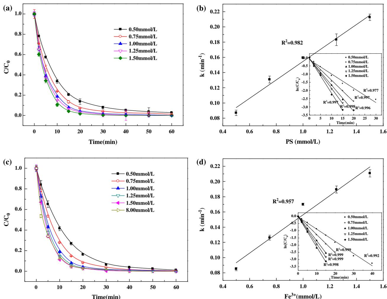
Fig. 4. Effects of (a and b) PS and (c and d) Fe<sup>3+</sup> concentration on RhB degradation. Experimental conditions: 0.052 mM [RhB]<sub>0</sub>, pH<sub>initial</sub> = 3.0, 1 mM [Fe<sup>3+</sup>]<sub>0</sub> (a and b), 1 mM [PS]<sub>0</sub> (c and d).
