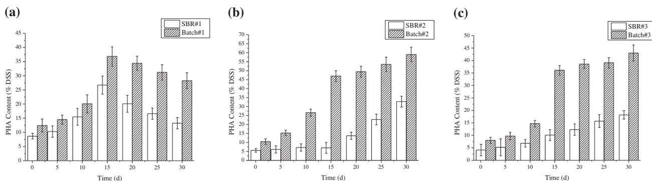
Fig. 5. Maximum PHA content achieved in the SBRs and in the batch tests: (a) SBR #1, (b) SBR #2, and (c) SBR #3.
