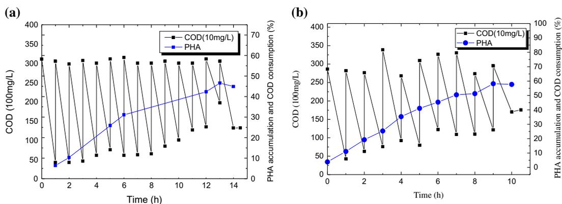
Fig. 7. COD consumption and PHA accumulation in Batch #2: (a) 15 d and (b) 30 d.
