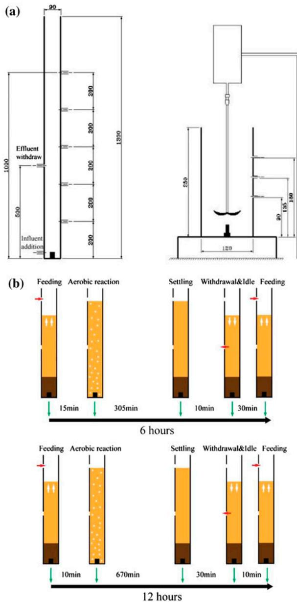
Fig. 1. The regime of one operating cycle for different feeding mode (a) SDD mode used in SBR #1 and SBR #2 and (b) ADF mode used in SBR #3.
