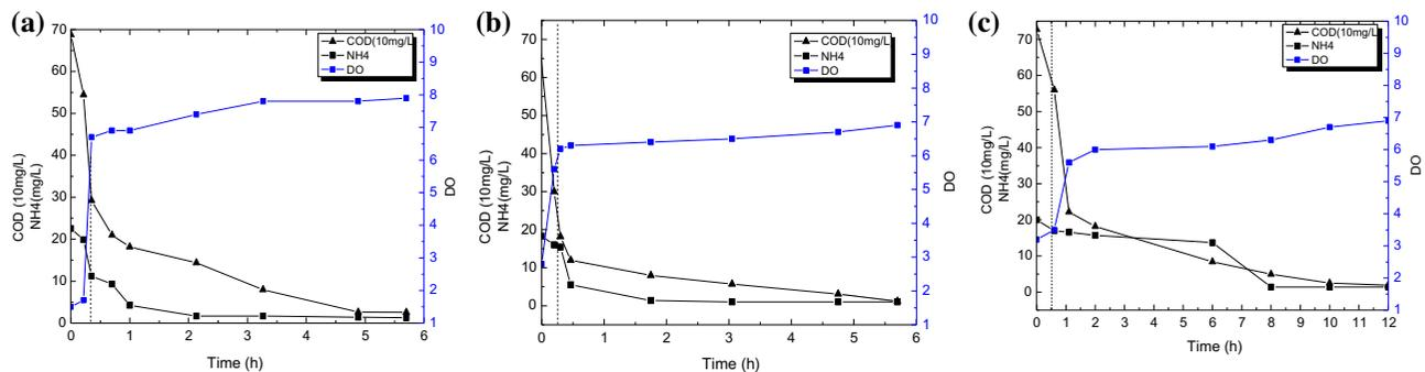
Fig. 4. Time profiles of the different parameters in a cycle of the: SBR #1 (a), SBR #2 (b), and SBR #3 (c) on day 15. Dashed lines mark the end of the feast phase.
