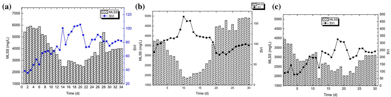
Fig. 3. The profile of the concentration of MLSS and SVI in the SBRs throughout the experiment: (a) SBR #1, (b) SBR #2, and (c) SBR #3.
