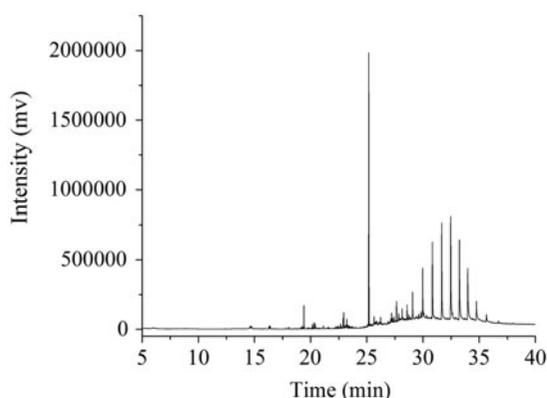
Fig. 1. The gas chromatograms of influent in the BESIR<sup>®</sup> process.
