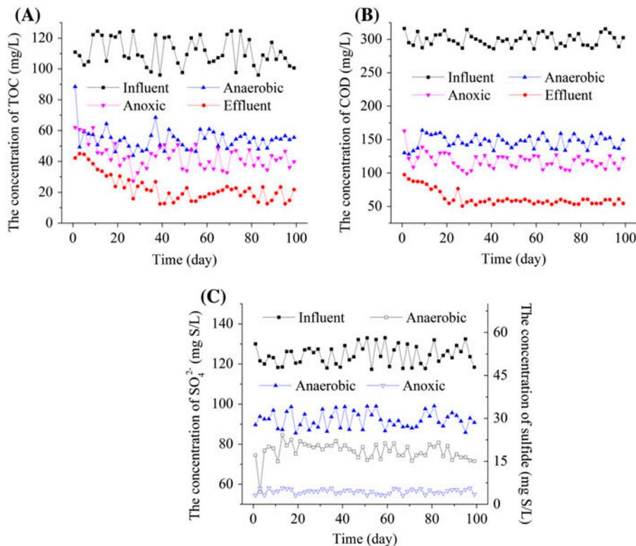
Fig. 3. (A) The organic removal and sulfur transformation efficiencies of the BEST<sup>®</sup> process, (B) TOC and COD removal efficiencies of each reactor, and (C) the sulfate concentration of influent and anaerobic effluent (represented by black lines and symbols), and the sulfide concentration of anaerobic and anoxic effluents (represented by blue lines and symbols).
