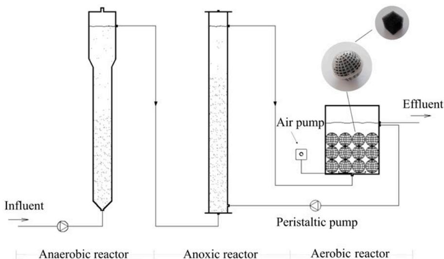
Fig. 2. Schematic diagram of the BESIR<sup>®</sup> process.
