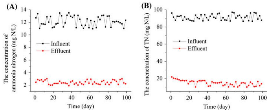
Fig. 4. The nitrogen removal efficiencies of the BES1<sup>®</sup> process: (A) the ammonia nitrogen concentration of influent and effluent and (B) the TN concentration of influent and effluent.
