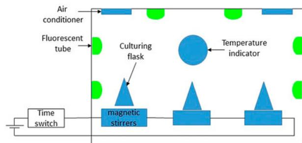
Fig. 1. Front view pattern of the designed photobioreactor.
