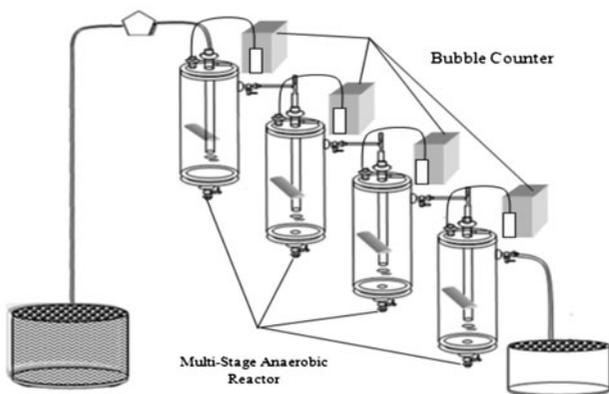
Fig. 1. Multi-stage anaerobic bioreactor.
