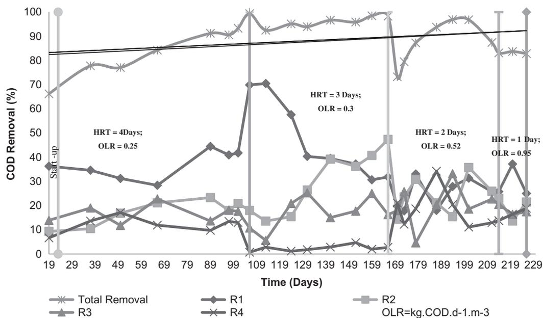
Fig. 3. COD removal profile of the bioreactor.
