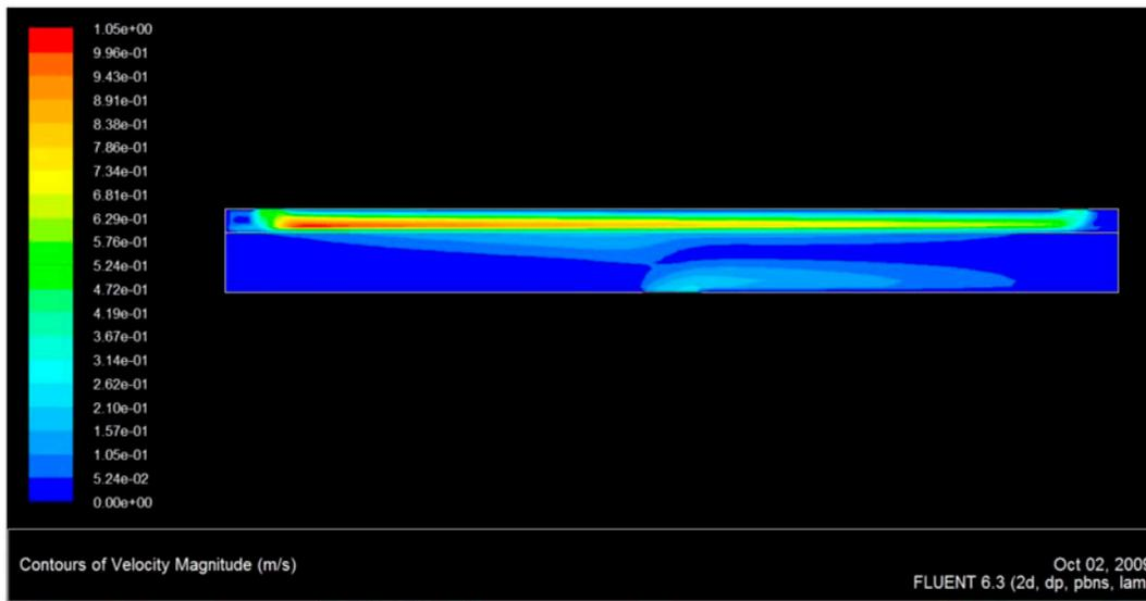
Fig. 6. Vector of velocity in flat sheet membrane module (feed canal height = 0.4 cm).
