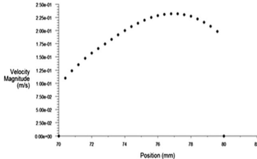
Fig. 8. Vector of velocity at outlet of permeate in flat sheet module (feed canal height = 2 cm).
