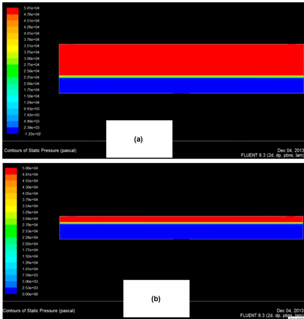
Fig. 2. Counter of pressure in flat sheet membrane module (a) feed canal height = 2 cm and (b) feed canal height = 0.4 cm.
