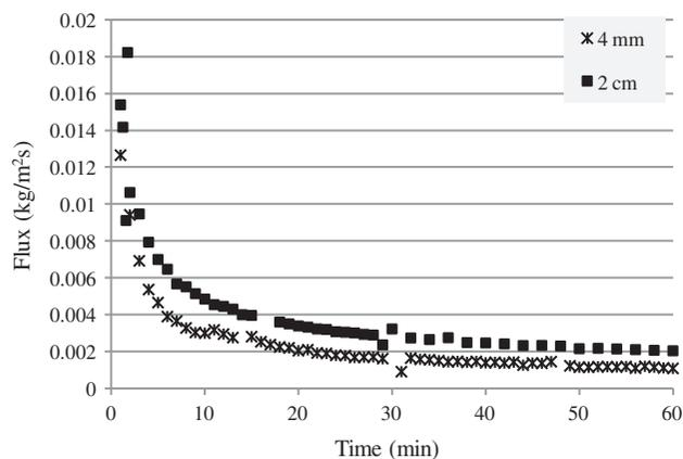
Fig. 9. Experimental data of the effect of feed canal height on permeate flux during membrane clarification of pomegranate juice.
