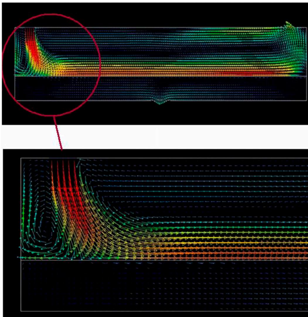
Fig. 3. Vector of flow in flat sheet membrane module (feed canal height = 2 cm).
