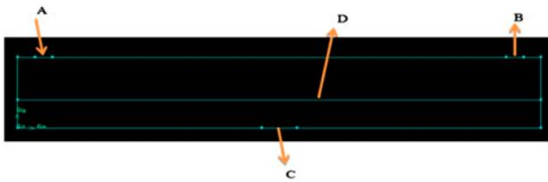
Fig. 1. Geometry of the membrane module which was used to clarify pomegranate juice (A–D are feed entrance, retentate exit, permeate exit, and membrane, respectively).
