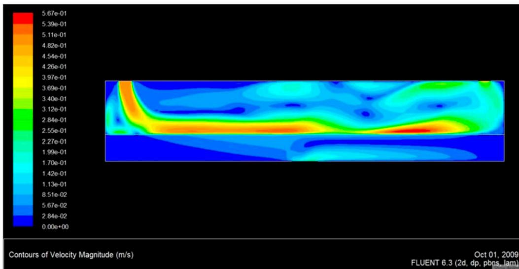
Fig. 5. Vector of velocity in flat sheet membrane module (feed canal height = 2 cm).
