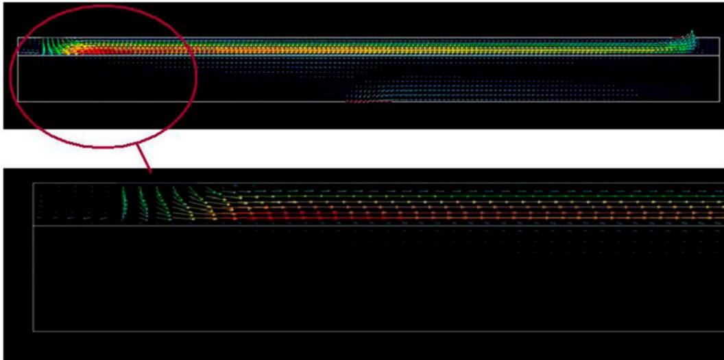
Fig. 4. Vector of flow in flat sheet membrane module (feed canal height = 0.4 cm).
