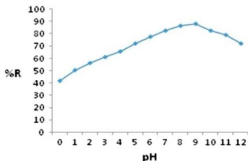
Fig. 5. Effect of pH on percentage removal of methylene blue dye by PANI–NiFe<sub>2</sub>O<sub>4</sub> catalyst dose 8 g/lt at 40 mg/L.
