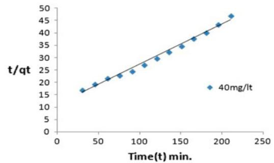
Fig. 9. Pseudo-second-order kinetics plots for the removal of methylene blue at 40 mg/L dye concentration: adsorbent dose 8 g/L and pH 9.
