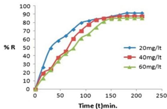
Fig. 6. Effect of contact time and initial concentration of methylene blue dye on % removal at adsorbent dose 8 g/L at pH 9.
