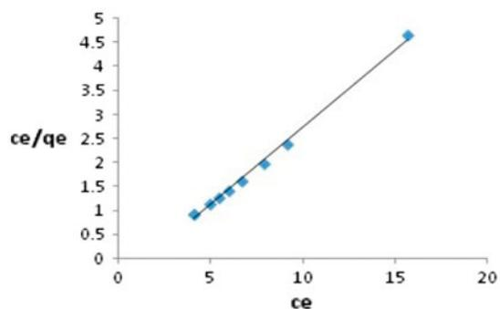
Fig. 11. Langmuir plot for adsorption of methylene blue by PANI–NiFe<sub>2</sub>O<sub>4</sub>.
