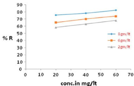
Fig. 4. Effect of initial dye conc. on percentage removal of methylene blue dye for different adsorbent doses with contact time 165 min and pH 9.
