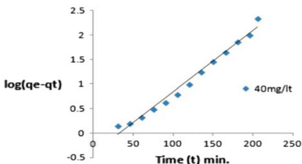
Fig. 8. Pseudo-first-order kinetics plots for the removal of methylene blue at 40 mg/L dye concentration: adsorbent dose 8 g/L and pH 9.
