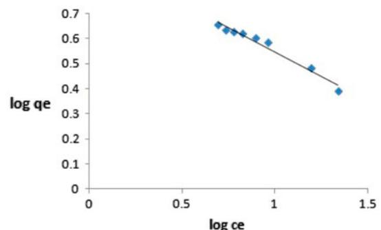
Fig. 10. Freundlich plot for adsorption of methylene blue by PANI-NiFe<sub>2</sub>O<sub>4</sub>.
