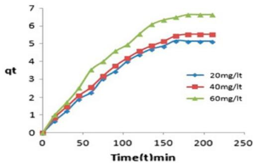
Fig. 7. Amount of dye adsorbed  $q_t$  (mg/g) with time for different initial dye concentrations: pH 9 and adsorbent dose 8 g/L.
