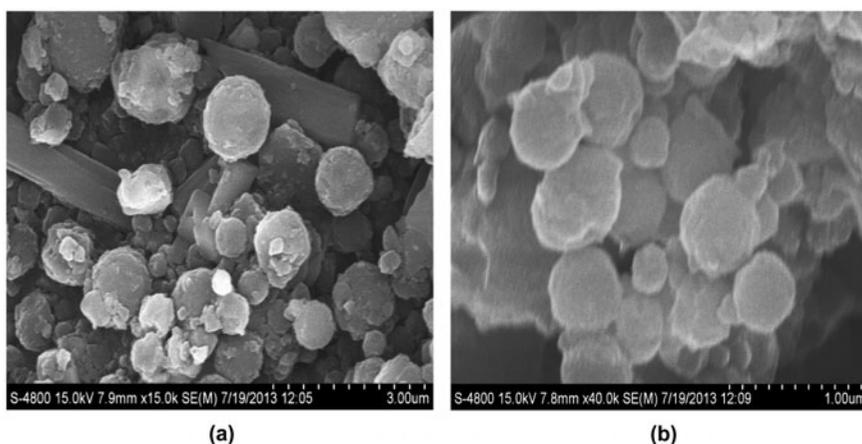
Fig. 2. (a) SEM images of prepared PANI–NiFe<sub>2</sub>O<sub>4</sub> nanocomposite before adsorption; (b) SEM image of PANI–NiFe<sub>2</sub>O<sub>4</sub> nanocomposite after adsorption of dye.
