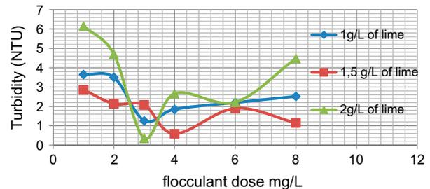
Fig. 10. Effect of the flocculant dose on lime removal.
