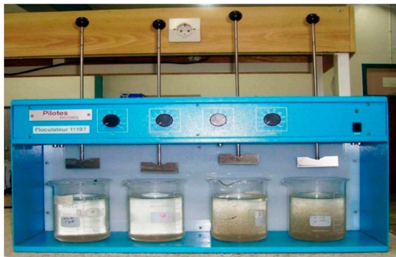
Fig. 1. The jar test (flocculator 11197) (Hydraulics Laboratory Department, Tlemcen University).
