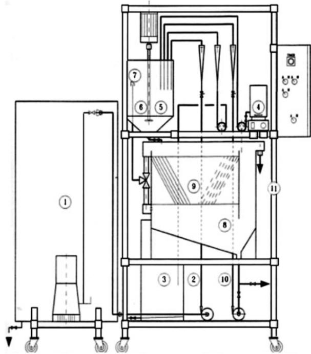
Fig. 3. Experimental device of the “TE 600” pilot.
