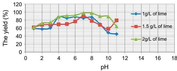
Fig. 11. Effect of pH on coagulation–flocculation.
