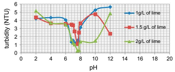
Fig. 12. Effect of pH on coagulation–flocculation.
