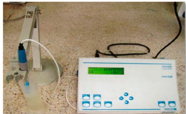
Fig. 5. pH measures (PHM220) (Hydraulics Laboratory Department, Tlemcen University).
