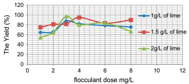
Fig. 9. Effect of the flocculant dose on lime removal.
