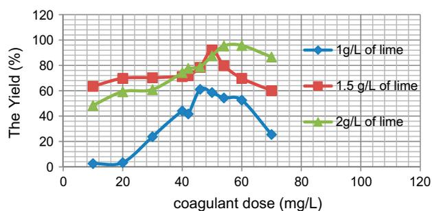
Fig. 6. Effect of the coagulant dose on lime removal.
