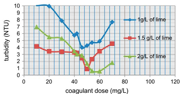
Fig. 7. Effect of the coagulant dose on lime removal.
