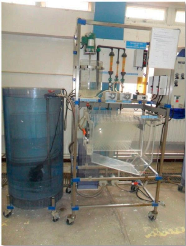
Fig. 2. Pilot of coagulation–flocculation and decantation (TE 600) (Hydraulics Laboratory Department, Tlemcen University).
