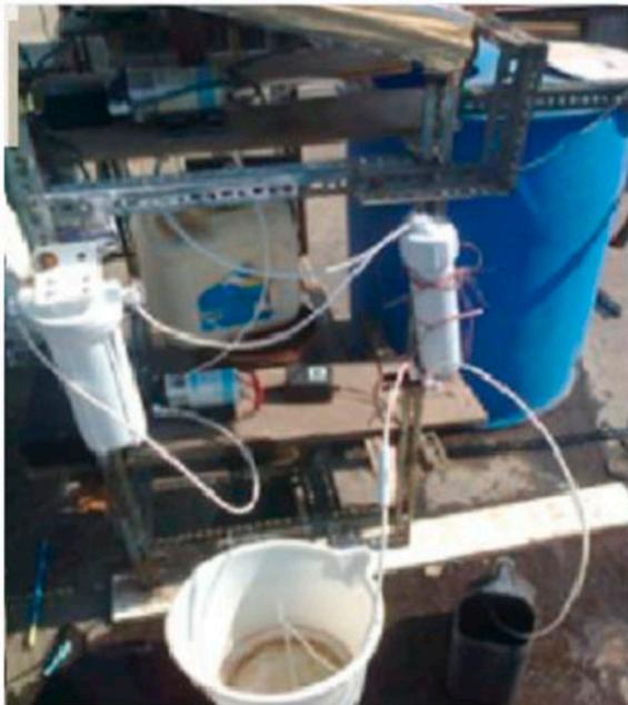
Fig. 1B. Domestic RO plant associated with solar PV panel.
