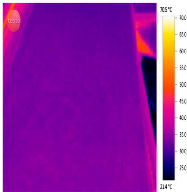
Fig. 3A. Thermal image of PV panel with cooling.
