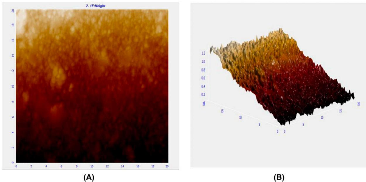
Fig. 5. (A, B) Atomic force microscope images of sodium hypochlorite-treated TFC RO membrane.
