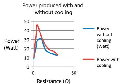
Fig. 4D. Power produced by PV panel at 1,500 h—11.11.2013.
