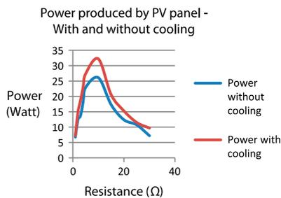
Fig. 4A. Power produced by PV panel at 1,100 h—11.11.2013.
