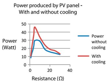
Fig. 4B. Power produced by PV panel at 1,200 h—11.11.2013.
