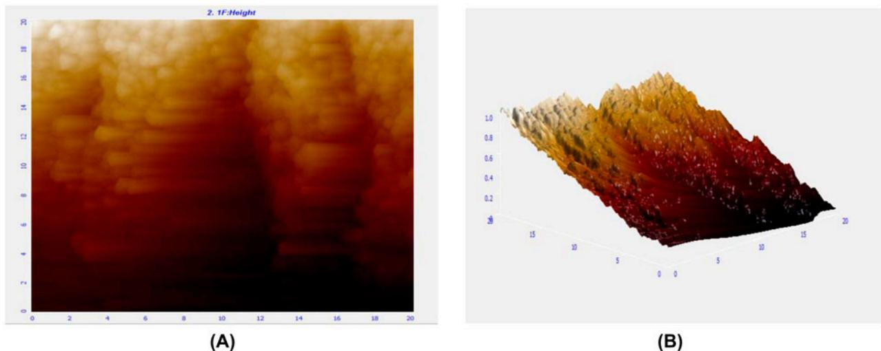
Fig. 6. (A, B) Atomic force microscope images of TFC RO membrane.
