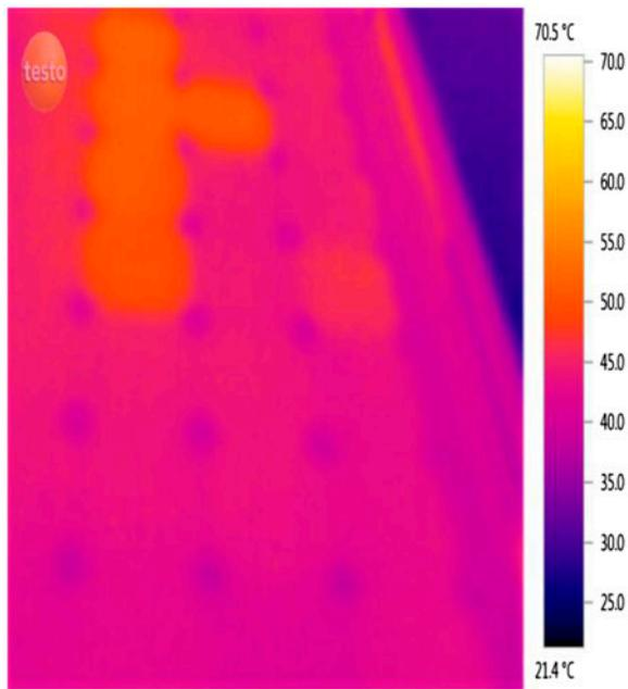
Fig. 3B. Thermal image of PV panel without cooling.
