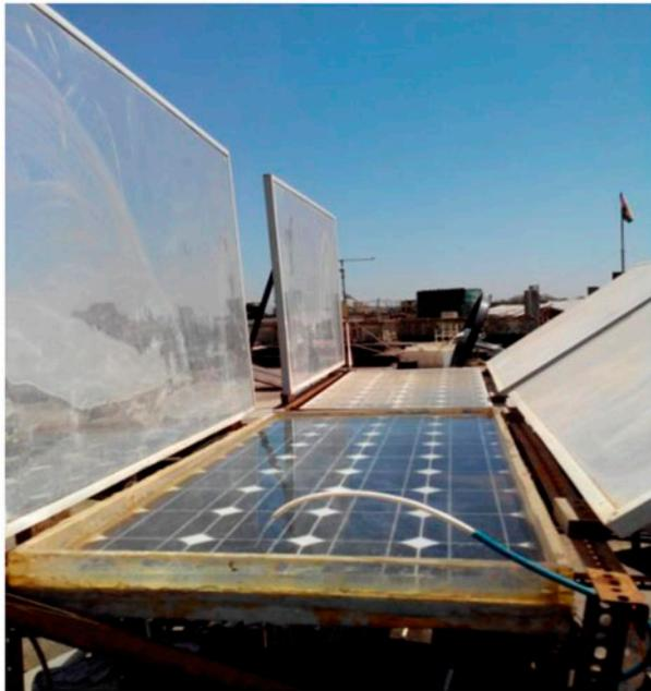
Fig. 1A. Horizontal PV Panel with cooling from top.
