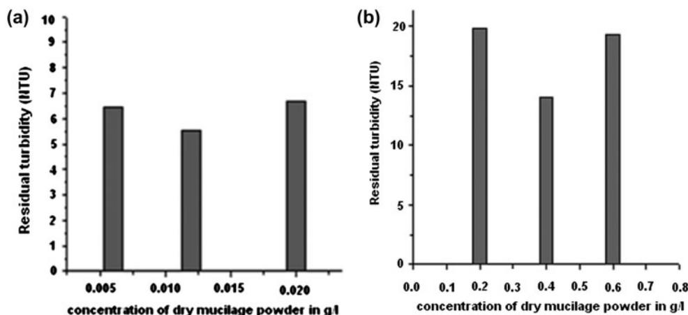
Fig. 7. Water clarifications by *Portulaca* mucilage powder (a) in low turbid water (35 NTU) and (b) in high turbid water (450 NTU).
