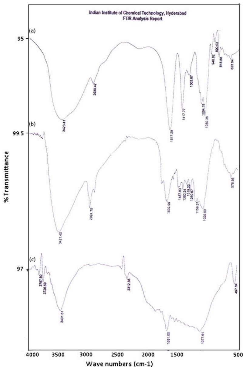
Fig. 3. FTIR spectra of (a) sodium alginate (b) *Portulaca* mucilage (c) PMA beads.
