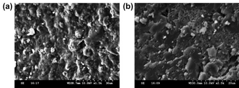
Fig. 2. SEM images of *portulaca* dry mucilage powder (a) before treatment with (450 NTU) turbid water and (b) after treatment with (450 NTU) turbid water.
