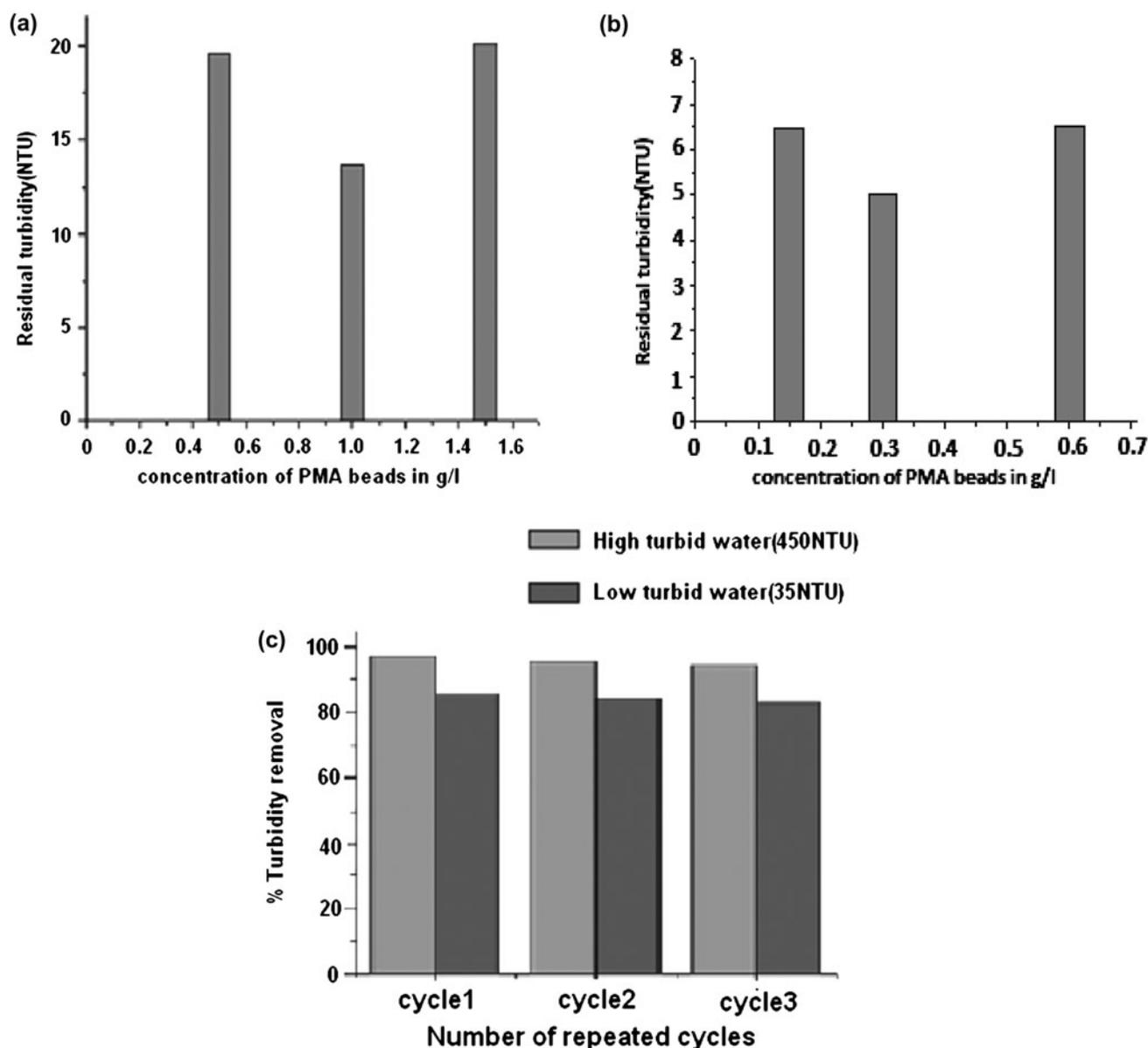
Fig. 6. Water clarifications by PMA beads (a) in high turbid water (450 NTU) (b) in low turbid water (35 NTU) levels (c) capability (%turbidity removal) of recycled PMA beads.
