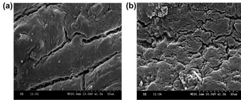
Fig. 1. SEM images of PMA beads (a) before treatment with (450 NTU) turbid water and (b) after treatment with (450 NTU) turbid water.
