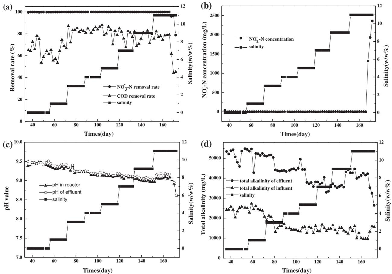
Fig. 1. The change of performance with the salinity in the EGSB reactor: (a) nitrate nitrogen and COD removal rate; (b) nitrite nitrogen accumulated concentration of the effluent; (c) pH in reactor and the effluent and (d) the total alkalinity of the influent and effluent.
