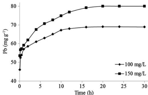
Fig. 4. Effect of agitation time on the adsorption of Pb(II) by HHPACAC.
