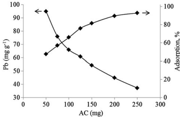
Fig. 5. Effect of HHP-CAC dosage on the adsorption of Pb(II).
