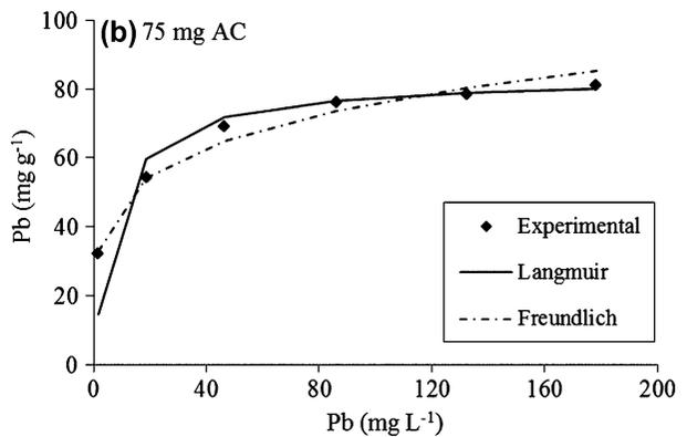
Fig. 7. Experimental, Langmuir, and Freundlich isotherms for the adsorption of Pb(II) onto HHP-CAC at various dosages, (a) 50 mg and (b) 75 mg.
