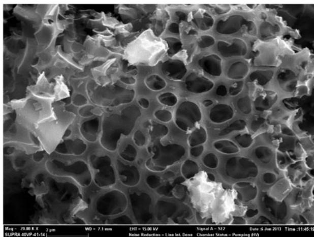
Fig. 1. SEM image of HHPAC (magnification 20,000 $\times$ ).
