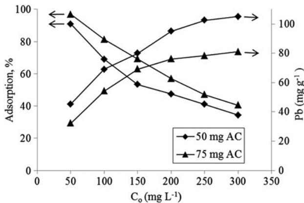
Fig. 6. Effect of Pb(II) initial concentration on the adsorption of Pb(II) onto HHP-CAC at various dosages.
