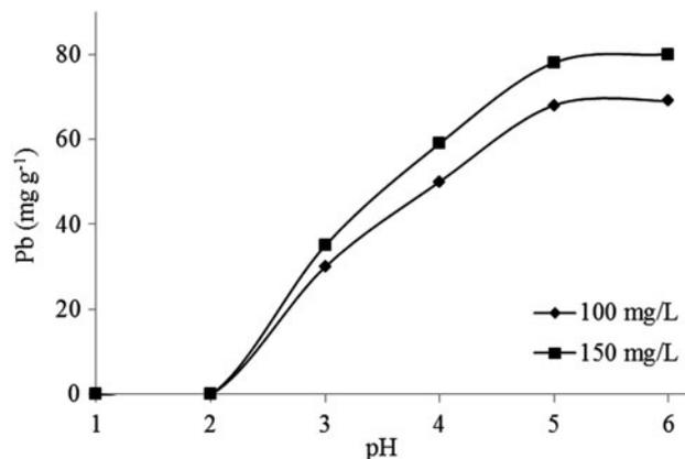
Fig. 3. Effect of initial pH on the adsorption of Pb(II) by HHPAC.
