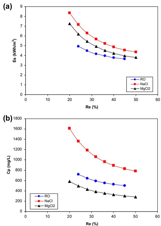
Fig. 6. RO membrane performance for seawater desalination: (a) specific power consumption in the RO, and (b) permeate TDS (feed TDS 35 g/L).
