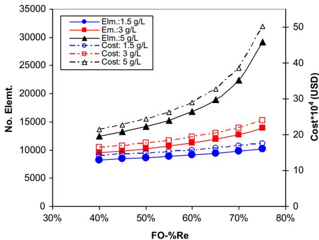
Fig. 8. Number and cost of FO element at different FO recovery rates and feed concentrations.
