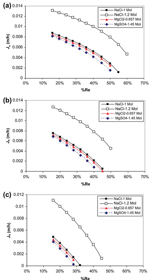
Fig. 3. Solute flux across the FO at different membrane recovery rates (a) seawater salinity 32,000 mg/L (b) seawater salinity 38,000 mg/L, and (c) seawater salinity 45,000 mg/L.
