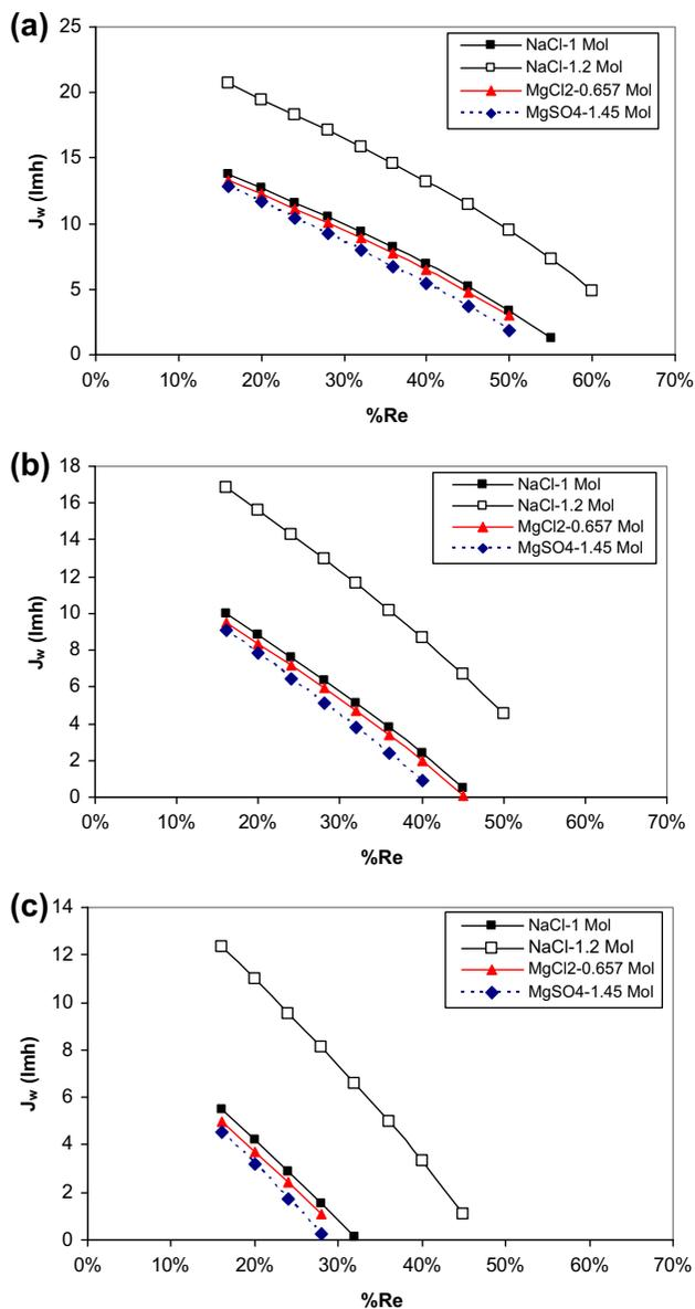
Fig. 2. Water flux through the FO at different membrane recovery rates (a) seawater salinity 32,000 mg/L (b) seawater salinity 38,000 mg/L, and (c) seawater salinity 45,000 mg/L.
