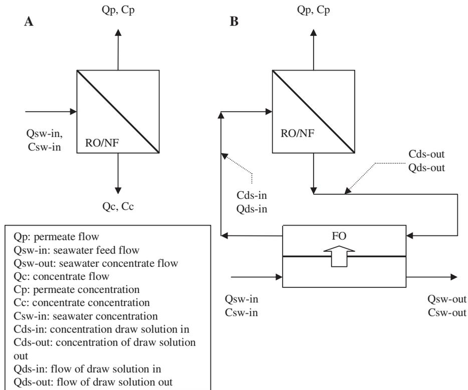
Fig. 1. RO and FO–RO processes diagram Altaee et al. [12].
