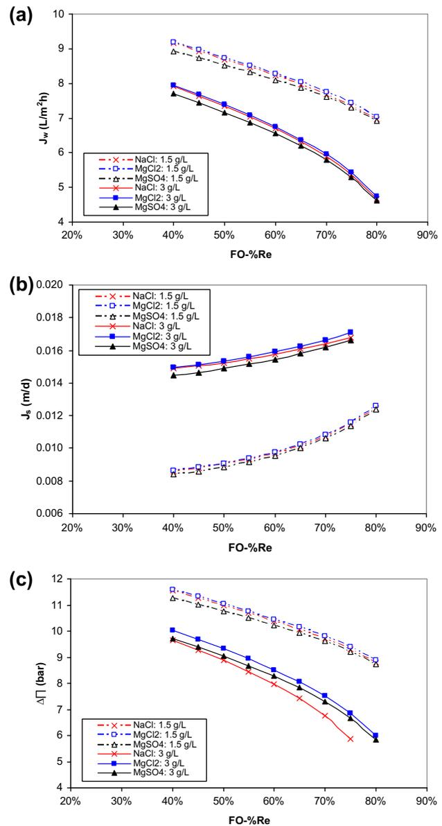
Fig. 4. FO performance at different recovery rates (a) impact on the membrane flux, (b) impact on the solute flux, and (c) impact on the osmotic pressure difference across the membrane.
