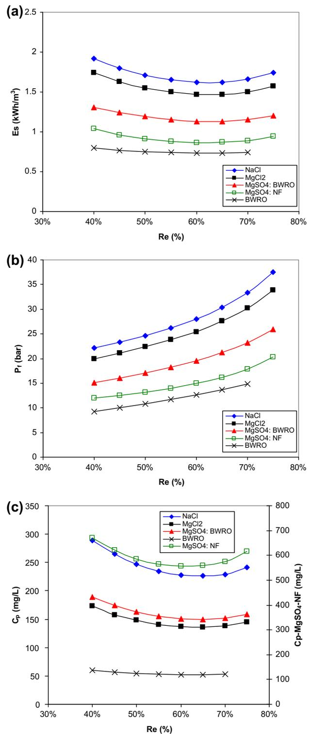
Fig. 7. Performance of BWRO and NF membranes for draw solution regeneration and fresh water extraction: (a) feed pressure, (b) specific power consumption, and (c) permeate TDS.
