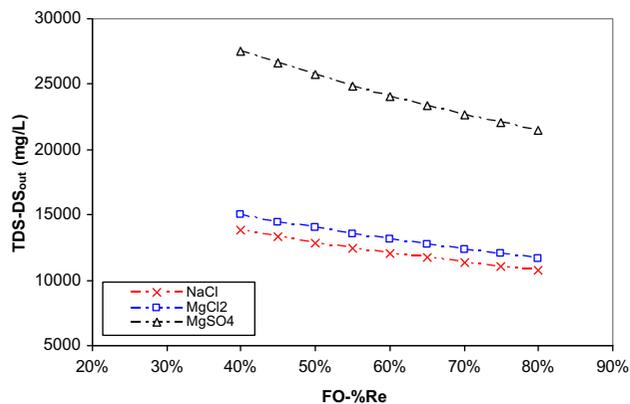
Fig. 5. The concentration of draw solution leaving the FO membrane at different FO recovery rates.
