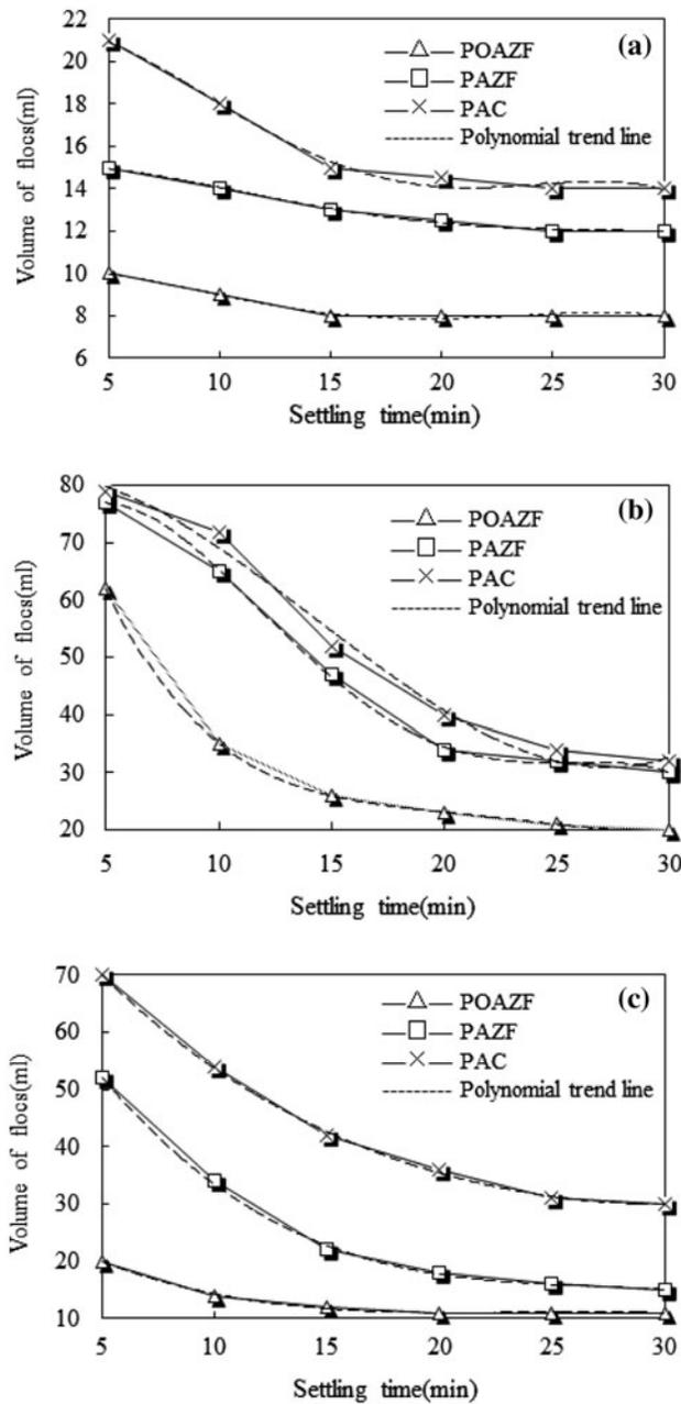
Fig. 3. Influence of settling time from 5 to 30 min and dosage of (a) 60 mg L<sup>-1</sup>, (b) 186 mg L<sup>-1</sup>, and (c) 372 mg L<sup>-1</sup> on settling performance of POAZF, PAZF, and PAC in treating sewage.
