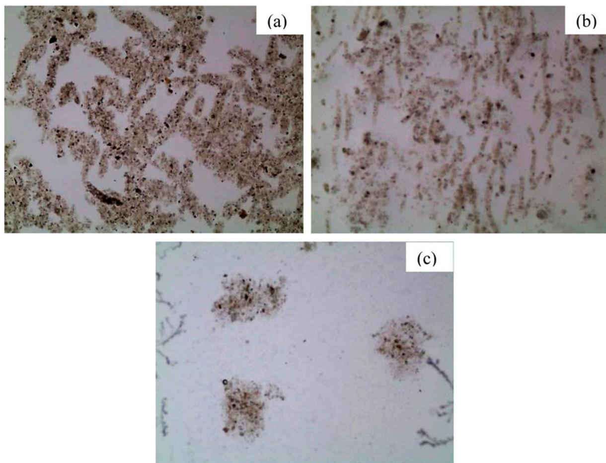
Fig. 2. Image of flocs formed by (a) POAZF, (b) PAZF, and (c) PAC in treating sewage (magnifies 100 diameters). Dosage = 186 mg L<sup>-1</sup>.
