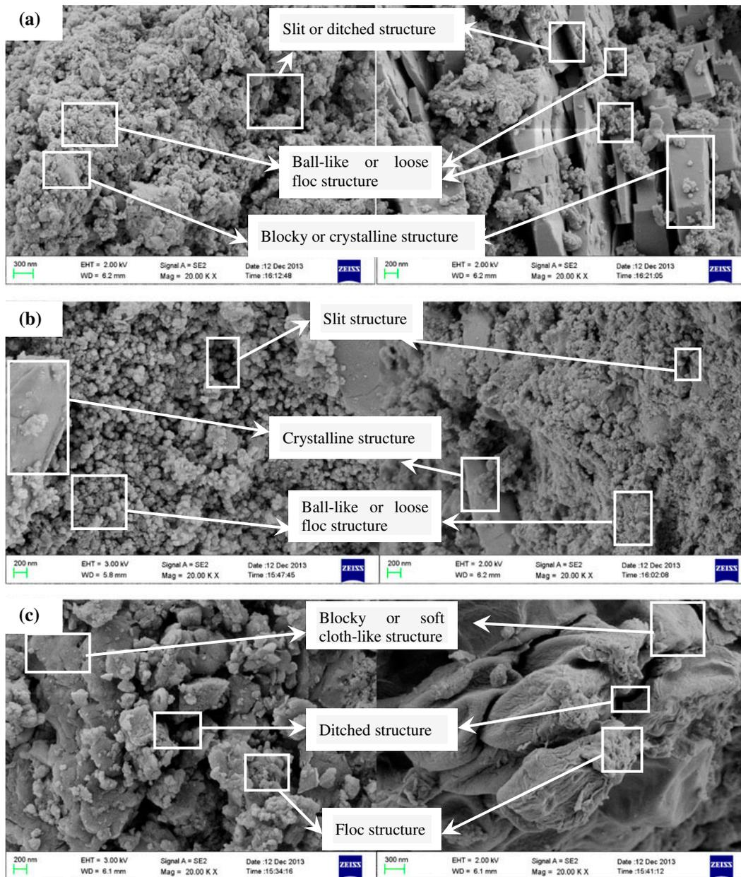
Fig. 5. Surface morphology of dry sludge formed by (a) POAZF, (b) PAZF, and (c) PAC in treating sewage (magnifies 20,000 diameters). Dosage = 186 mg L<sup>-1</sup>.
