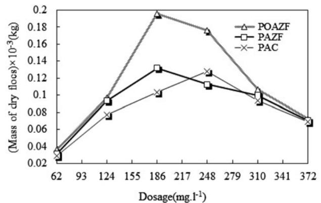
Fig. 6. Influence of dosage on mass of dry sludge formed by POAZF, PAZF, and PAC in treating sewage.
