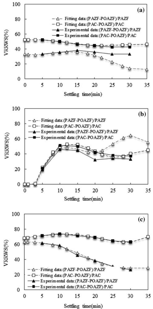
Fig. 4. Comparison of VRRWS of POAZF between experimental data and calculating data in treating sewage at different dosages of (a) 60 mg L<sup>-1</sup>, (b) 186 mg L<sup>-1</sup>, and (c) 372 mg L<sup>-1</sup> and different settling times from 5 to 30 min (comparison with that of PAZF and PAC). VRRWS: volume reduction ratio of wet sludge.
