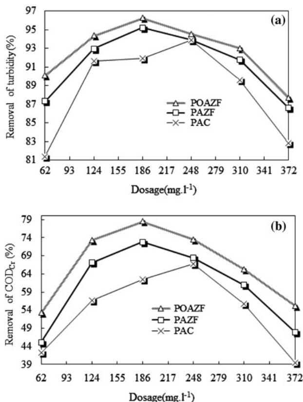
Fig. 1. Influence of dosage on removal of (a) turbidity and (b) COD<sub>Cr</sub> by POAZF, PAZF and PAC in treating sewage.
