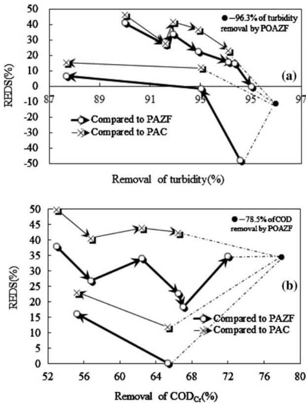
Fig. 7. Influence of removal of (a) turbidity, and (b) organic matters on REDS of POAZF in treating sewage (in contrast to PAZF and PAC). REDS: reduction rate of dry sludge.
