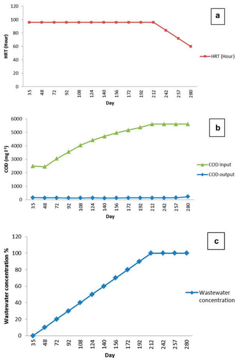
Fig. 5. The exchange of certain parameters in the UAPB reactor process: (a) HRT; (b) input and output COD concentrations; and (c) wastewater concentration.
