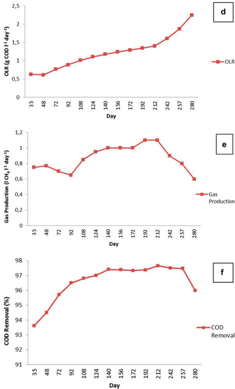
Fig. 6. The exchange of certain parameters in the UAPB reactor process: (d) OLR; (e) gas production; and (f) COD removal.
