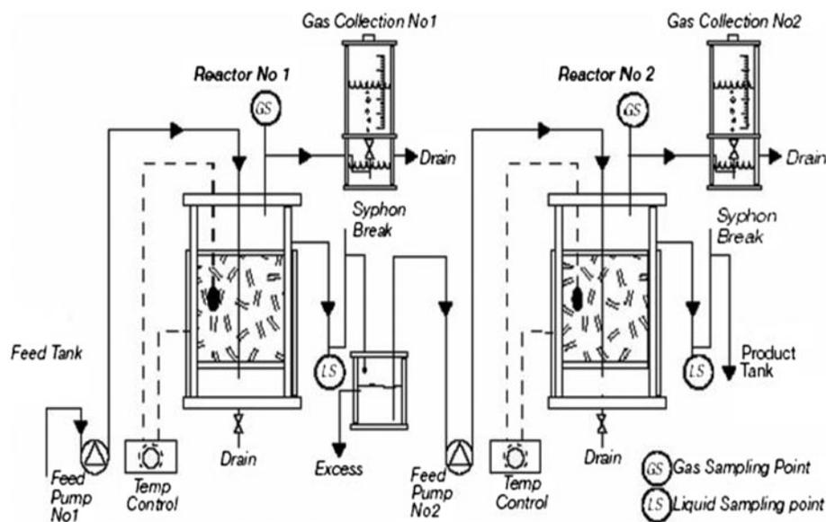
Fig. 1. Design of UAPB reactor (Armfield W8).
