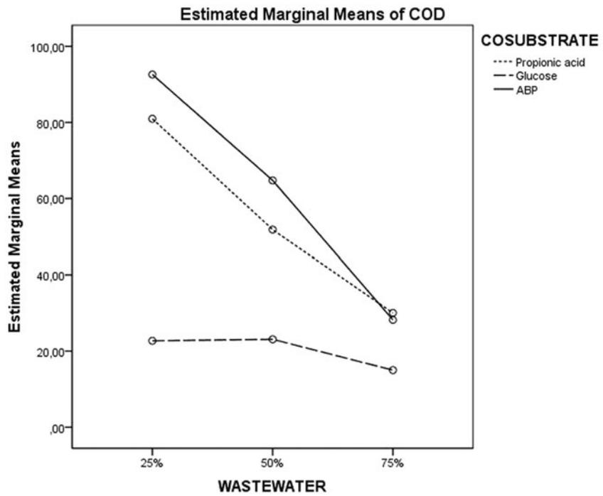
Fig. 3. Profile diagram for co-substrate and wastewater interaction.
