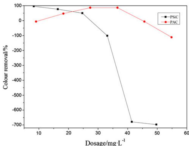
Fig. 6. Color removal of PAC and PSiC<sub>0.9</sub> with different dosage in the treatment of biologically treated effluent from a recycled paper mill.
