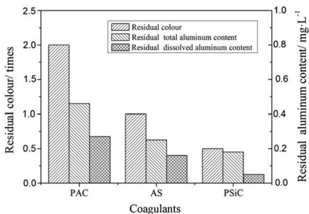
Fig. 8. Residual color and aluminum content in the effluent from secondary settler of a recycled paper mill treated with PSiC<sub>0.9</sub>, PAC, and AS.
