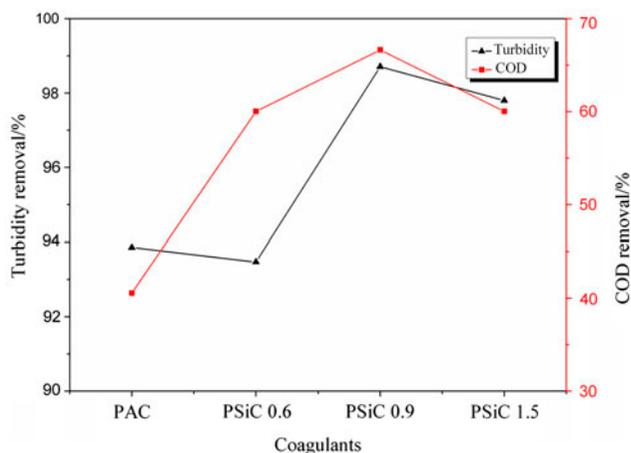
Fig. 7. Coagulation performance of PAC and PSiCs with different Si/(Al + Fe) molar ratios in the treatment of biologically treated effluent from a recycled paper mill.
