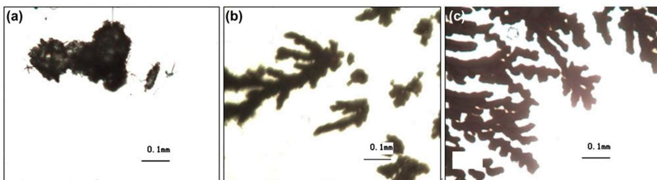
Fig. 4. Morphology of PSiC with Si/(Al + Fe) molar ratios of (a) 0.6, (b) 0.9, and (c) 1.5.
