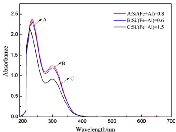
Fig. 3. UVA scanning spectra of PSiC with different Si/(Al + Fe) molar ratios.
