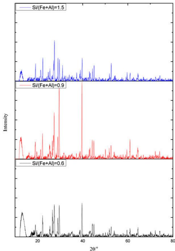
Fig. 1. XRD spectra of PSiC with Si/(Al + Fe) molar ratios of (a) 0.6, (b) 0.9, and (c) 1.5.
