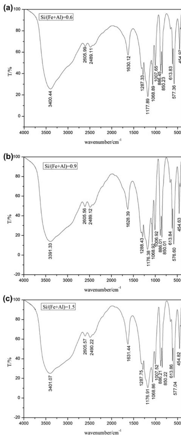
Fig. 2. IR spectra of PSiC with different Si/(Al + Fe) molar ratios of (a) 0.6, (b) 0.9, and (c) 1.5.
