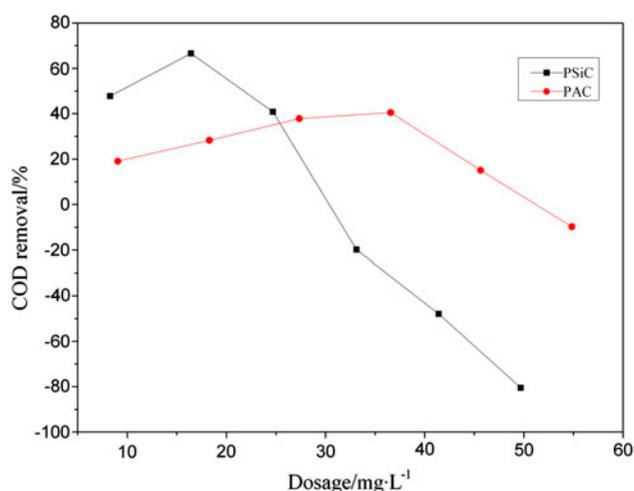
Fig. 5. COD removal of PAC and PSiC<sub>0.9</sub> with different dosage in the treatment of biologically treated effluent from a recycled paper mill.
