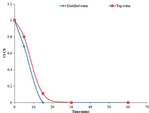
Fig. 11. Effect of purity of water used to prepare NaF solution on rate of defluoridation of NaF solution (AR grade),  $C_i = 5.23$  mg/L, volume of solution = 1 L, seven bipolar electrodes, speed of stirring = 300 rpm, current = 250 mA, voltage = 10.5 V.
