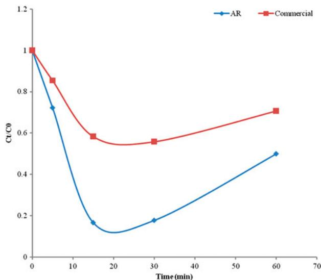
Fig. 12. Effect of purity of NaF solution on rate of defluoridation of NaF solution,  $C_i = 13.02$  mg/L, volume of solution = 1 L, seven bipolar electrodes, speed of stirring = 300 rpm, current = 250 mA, voltage = 10.5 V.
