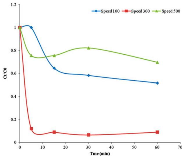
Fig. 3. Effect of speed of stirring on rate of defluoridation of NaF solution (AR grade),  $C_i = 12.76$  mg/L, volume of solution = 1 L, seven bipolar electrodes, current = 250 mA, voltage = 10.5 V.
