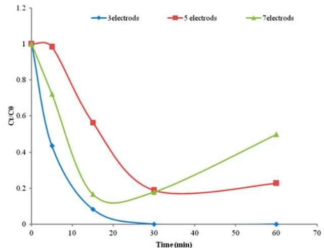
Fig. 4. Effect of number of electrodes on rate of defluoridation of NaF solution (AR grade),  $C_i = 13.43$  mg/L, volume of solution = 1 L, seven bipolar electrodes, speed of stirring = 300 rpm, current = 250 mA, voltage = 10.5 V.
