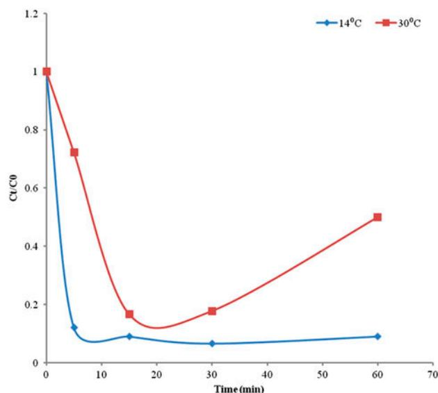
Fig. 10. Effect of temperature on rate of defluoridation of NaF solution (AR grade),  $C_i = 11.9$  mg/L, volume of solution = 1 L, seven bipolar electrodes, speed of stirring = 300 rpm, current = 250 mA, voltage = 10.5 V.
