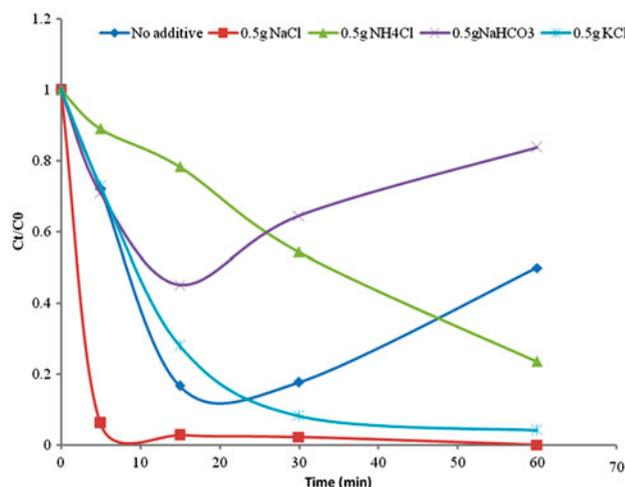
Fig. 6. Effect of using different additives rather than NaCl added as electrolyte on rate of defluoridation of NaF solution (AR grade),  $C_i = 11.7$  mg/L, volume of solution = 1 L, seven bipolar electrodes, speed of stirring = 300 rpm, current = 250 mA, voltage = 10.5 V.
