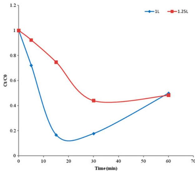
Fig. 7. Effect of volume of solution on rate of defluoridation of NaF solution (AR grade),  $C_i = 11.9$  mg/L, seven bipolar electrodes, speed of stirring = 300 rpm, current = 250 mA, voltage = 10.5 V.
