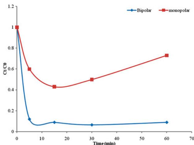
Fig. 9. Effect of electrode configurations on rate of defluoridation of NaF solution (AR grade),  $C_i = 11.5$  mg/L, volume of solution = 1 L, speed of stirring = 300 rpm, current = 250 mA, voltage = 10.5 V.
