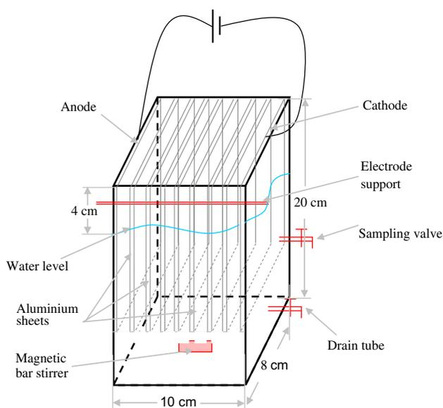
Fig. 1. Schematic diagram of setup.
