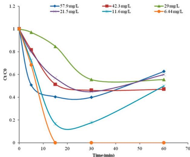
Fig. 2. Effect of initial concentration of fluoride in different AR grade NaF solutions on rate of defluoridation,  $C_i = 57.9$ – $6.44$  mg/L, volume of solution = 1 L, seven bipolar electrodes, speed of stirring = 300 rpm, current = 250 mA, voltage = 10.5 V.
