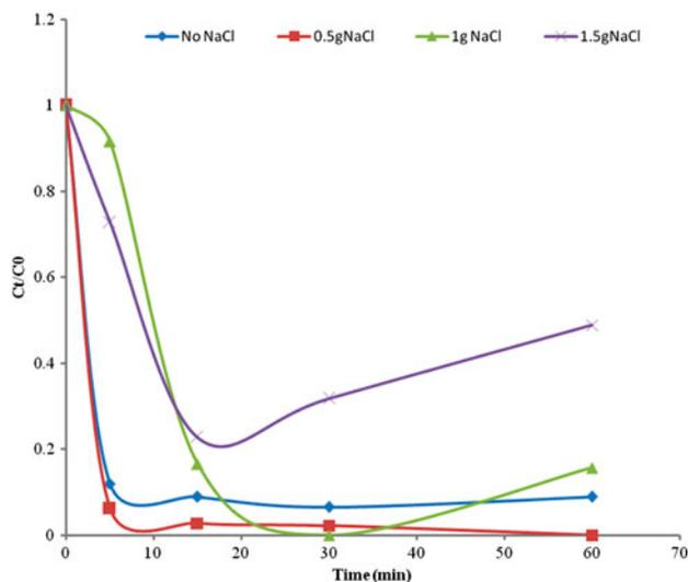
Fig. 5. Effect of amount of NaCl added as electrolyte on rate of defluoridation of NaF solution (AR grade),  $C_i = 12.24$  mg/L, volume of solution = 1 L, seven bipolar electrodes, speed of stirring = 300 rpm, current = 250 mA, voltage = 10.5 V.
