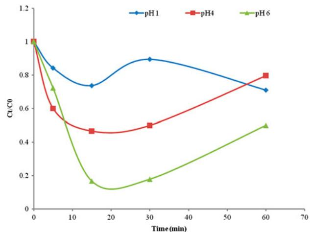
Fig. 8. Effect of pH on rate of defluoridation of NaF solution (AR grade),  $C_i = 11.53$  mg/L, volume of solution = 1 L, seven bipolar electrodes, speed of stirring = 300 rpm, current = 250 mA, voltage = 10.5 V.
