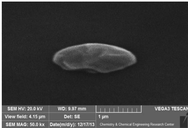
Fig. 7. SEM images of silica-filled hybrid membrane with 5 wt.% surfactant (Micelle formation around filler), magnification of 50k $\times$ .
