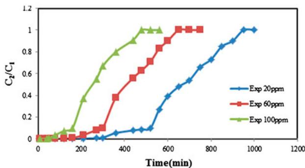
Fig. 8. The effect of the initial Cd(II) concentration on the breakthrough curve of Cd(II) adsorption on sesame waste (the bed depth of 2 cm; the flow rate of 3.5 mL min<sup>-1</sup>; the pH of 5.5).
