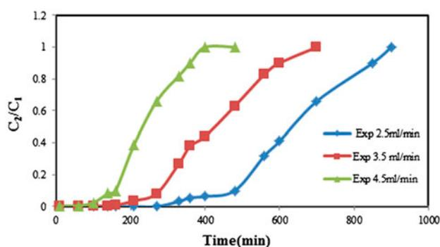
Fig. 7. The effect of flow rate on the breakthrough curve of Cd(II) adsorption on sesame waste (the bed depth of 2 cm, the initial Cd(II) concentration of 60 mg L<sup>-1</sup>; the pH of 5.5).
