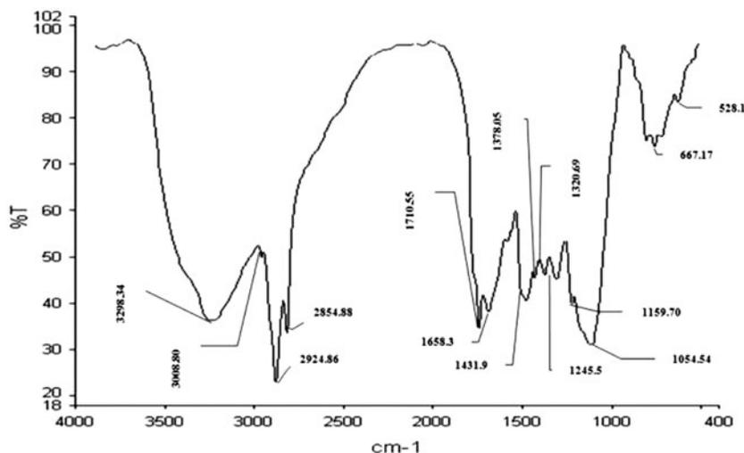
Fig. 3. FTIR spectra of sesame waste.
