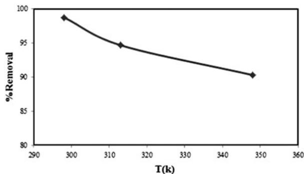
Fig. 4. The effect of temperature on the removal of Cd(II) (the initial Cd(II) concentration of  $60 \text{ mg L}^{-1}$ , the pH of 6; the stirring speed of 240 rpm and the adsorbent dose of  $3.33 \text{ g dm}^{-3}$ ).
