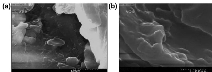
Fig. 2. Scanning electron micrograph of biosorbent (a) before Cd(II) adsorption and (b) after Cd(II) adsorption.
