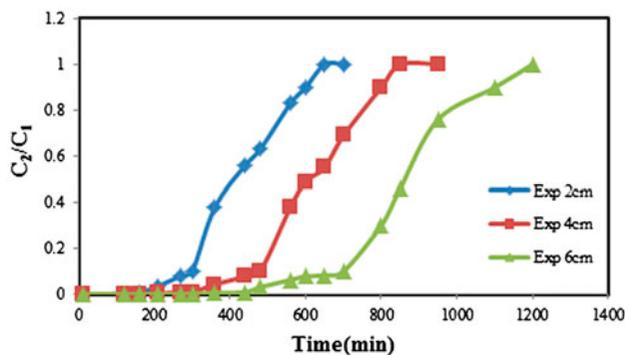
Fig. 6. The effect of bed depth on the breakthrough curve of Cd(II) adsorption on sesame waste (the initial Cd(II) concentration of  $60 \text{ mg L}^{-1}$ ; the flow rate of  $3.5 \text{ mL min}^{-1}$ ; the pH of 5.5).
