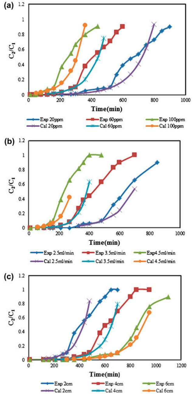
Fig. 9. Experimental and theoretical breakthrough curves based on Bohart–Adams model: the pH of 5.5 room temperature: (a) different flow rates, the influent Cd(II) concentration of  $60 \text{ mg L}^{-1}$ , the bed height of 2 cm, (b) different initial cadmium concentrations, the flow rate of  $3.5 \text{ mL min}^{-1}$ , the bed height of 2 cm, and (c) different bed heights, the influent Cd(II) concentration of  $60 \text{ mg L}^{-1}$ , the flow rate of  $3.5 \text{ mL min}^{-1}$ .
