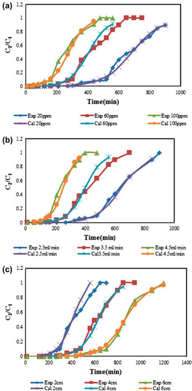
Fig. 10. Experimental and theoretical breakthrough curves based on Thomas model: at the pH of 5.5 and room temperature (a): different flow rates, the influent Cd(II) concentration of  $60 \text{ mg L}^{-1}$ , the bed height of 2 cm, (b) different initial cadmium concentrations, the flow rate of  $3.5 \text{ mL min}^{-1}$ , the bed height of 2 cm, and (c) different bed heights, the influent Cd(II) concentration of  $60 \text{ mg L}^{-1}$ , the flow rate of  $3.5 \text{ mL min}^{-1}$ .
