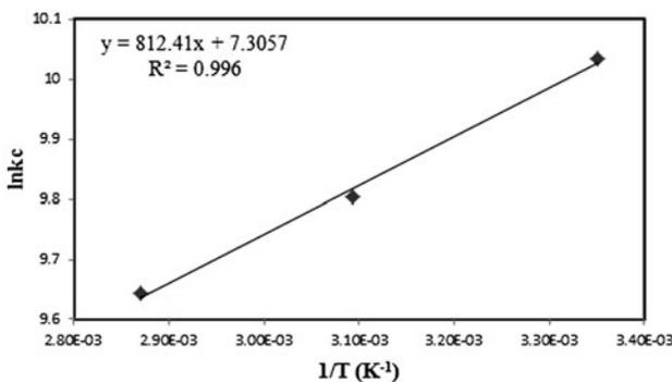
Fig. 5. Linear plot of  $\ln k_c$  vs.  $1/T$  (the initial Cd(II) concentration of  $60 \text{ mg L}^{-1}$ ; the pH of 6; the stirring speed of 240 rpm and adsorbent dose of  $3.33 \text{ g dm}^{-3}$ ).
