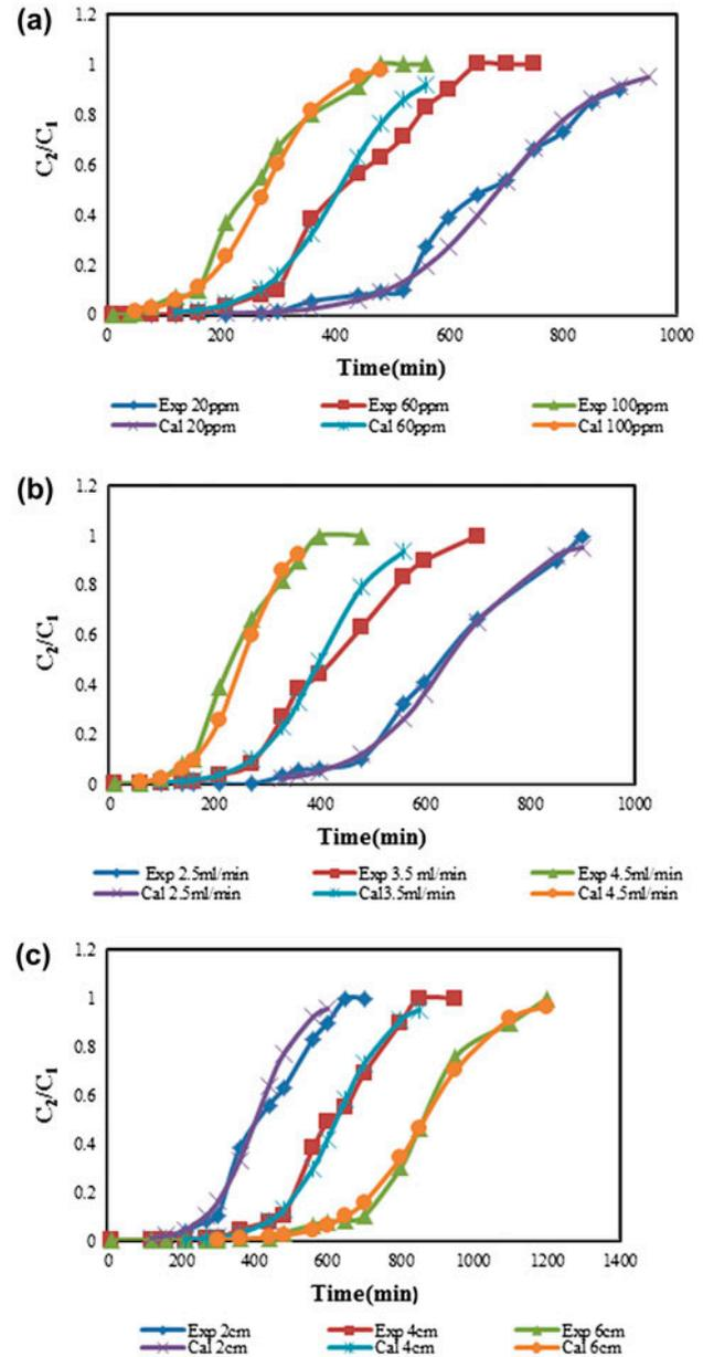
Fig. 11. Experimental and theoretical breakthrough curves based on Yoon–Nelson model: at the pH of 5.5 and room temperature (a): different flow rates, the influent Cd(II) concentration of  $60 \text{ mg L}^{-1}$ , the bed height of 2 cm, (b) different initial cadmium concentrations, the flow rate of  $3.5 \text{ mL min}^{-1}$ , the bed height of 2 cm, and (c) different bed heights, the influent Cd(II) concentration of  $60 \text{ mg L}^{-1}$ , the flow rate of  $3.5 \text{ mL min}^{-1}$ .
