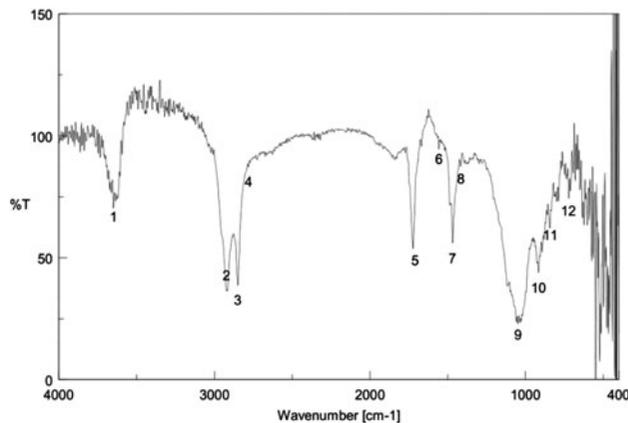
Fig. 4. FTIR spectra of UPR.
