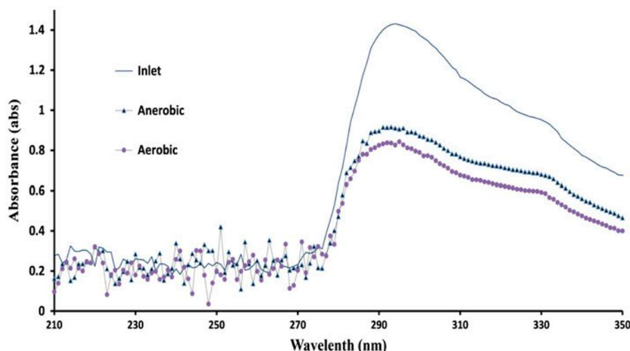
Fig. 8. UV-vis spectra of influent, effluent of anodic chamber and effluent of cathodic chamber.
