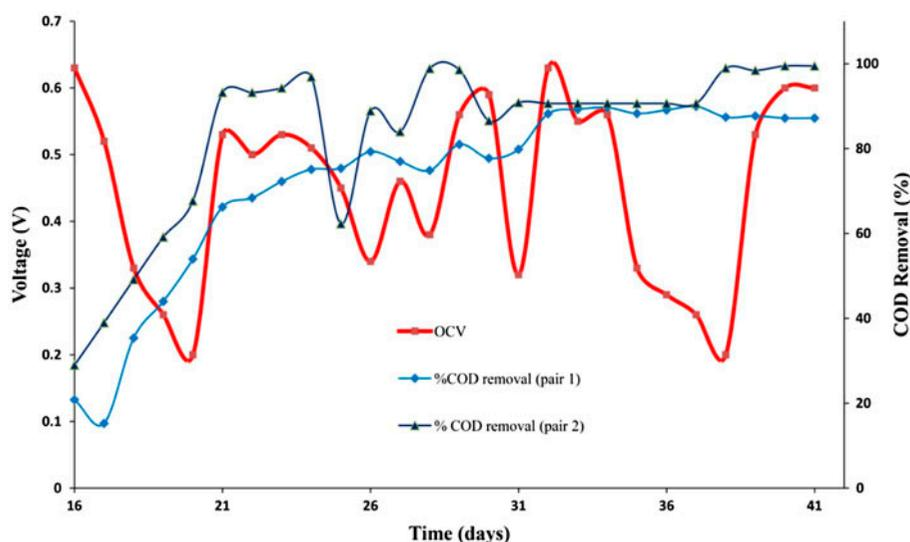
Fig. 2. Start-up values of OCV and percent COD removal of both pairs at 48 h HRT with domestic wastewater.
