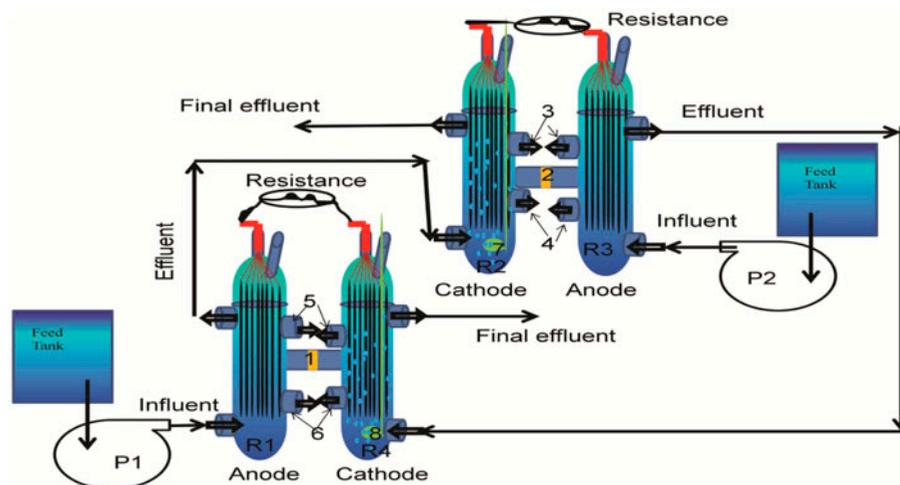
Fig. 1. Schematic sketch of CMFC used in the experimental study; R1 and R3 (anode) R2 and R4 (cathode), R1 and R4 form MFC 1, R2 and R3 form MFC 2; P1 and P2 are peristaltic pumps; 1 and 2 PEM; 3, 4, 5, and 6 sampling port; 7 and 8 are air spargers.
