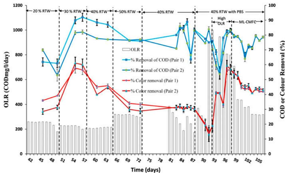
Fig. 3. Variation of COD and color removal at 24 h HRT with different percentage of RTW with, OLR and for ML-CMFC.
