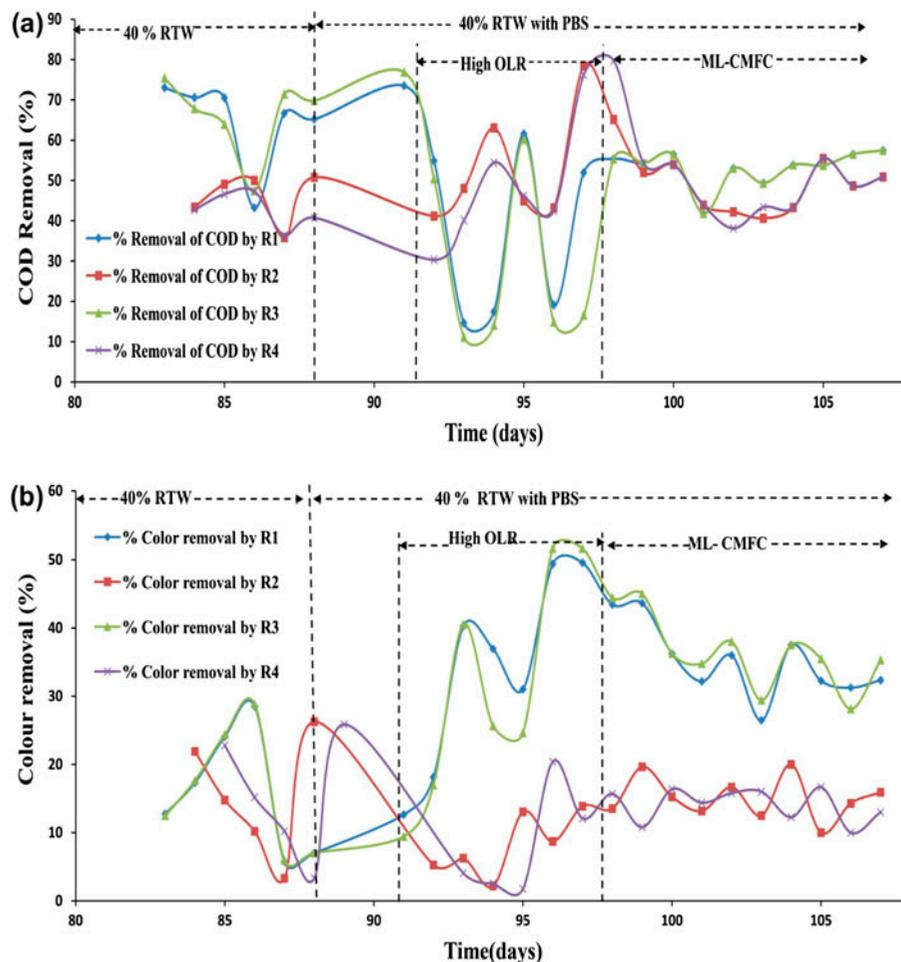
Fig. 5. (a) Percent COD removal (b) Percent color by R1, R2, R3, and R4 at 40% RTW and 40% RTW with PBS.
