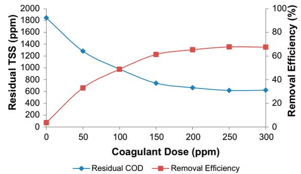
Fig. 9. Effect of alum sludge and chitosan on COD removal.
