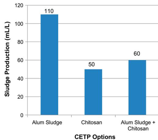
Fig. 10. CEPT options and sludge production.
