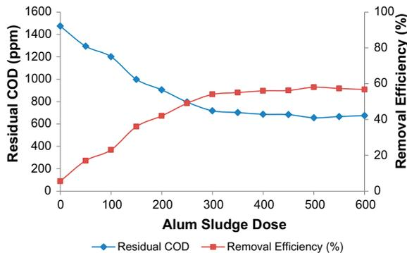
Fig. 3. Effect of alum sludge dose on COD removal.
