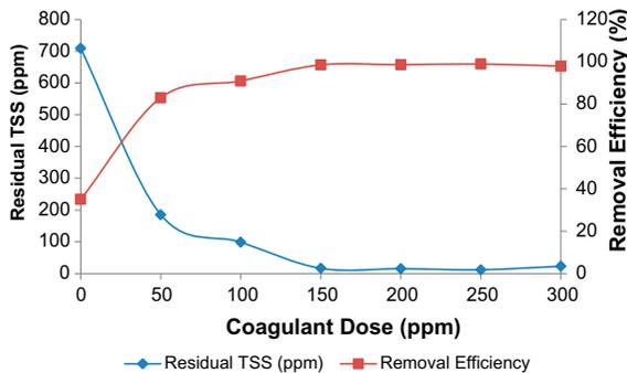
Fig. 7. Effect of alum sludge and chitosan on TSS removal.
