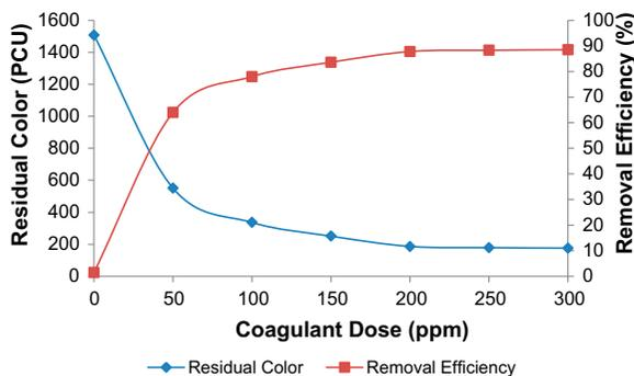
Fig. 8. Effect of alum sludge and chitosan on color removal.
