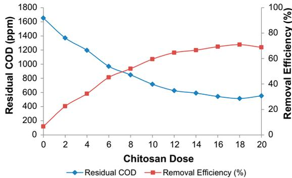
Fig. 6. Effect of chitosan dose on COD removal.
