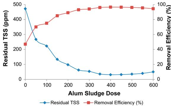
Fig. 1. Effect of alum sludge dose on TSS removal.
