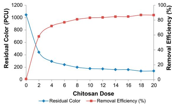
Fig. 5. Effect of chitosan dose on color removal.
