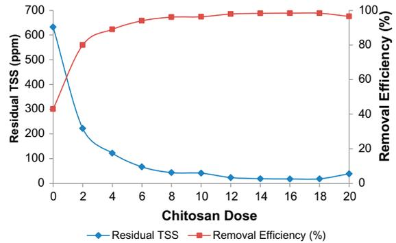
Fig. 4. Effect of chitosan dose on TSS removal.
