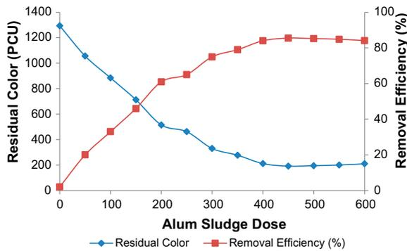
Fig. 2. Effect of alum sludge dose on color removal.
