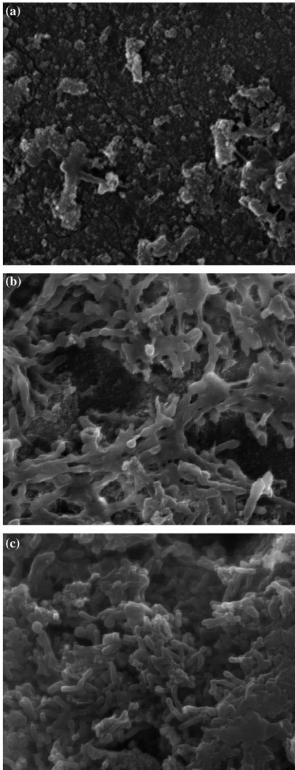
Fig. 3. Morphology of packing materials at various times. (a) Clean packing materials, (b) packing materials after running for 8 d, and (c) packing materials after running for 35 d.
