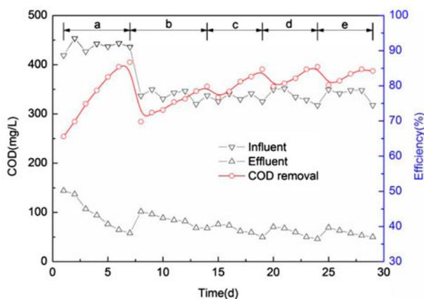
Fig. 2. Performance of BAF reactor at acclimation and stabilization stage. (a-glucose solution/wastewater = 1:1, HRT 24 h, 7 d; b-only wastewater, HRT 16 h, 7 d; c-only wastewater, HRT 12 h, 5 d; d-only wastewater, HRT 8 h, 5 d; e-only wastewater, HRT 6 h, 5 d).
