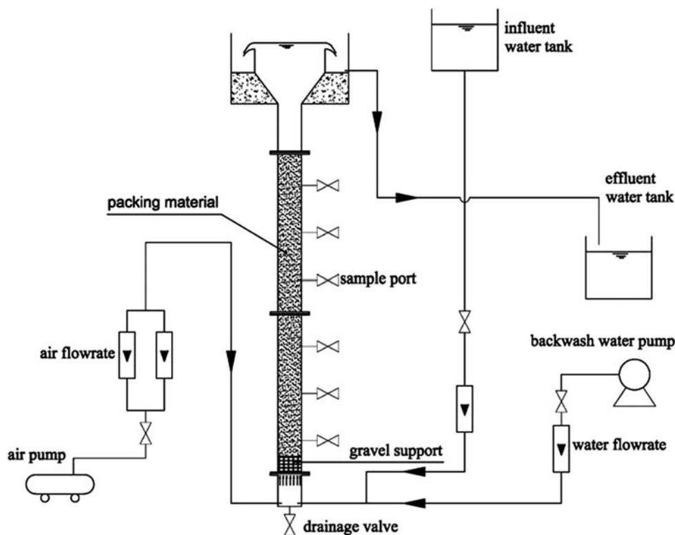
Fig. 1. Schematic configuration for the biological aerated filter reactor.
