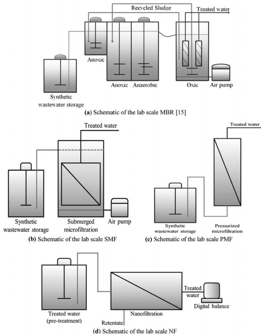
Fig. 1. Schematic diagram of lab scale: (a) MBR [15], (b) SMF, (c) PMF, and (d) NF processes.
