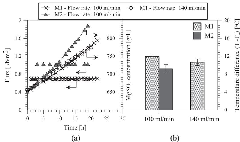
Fig. 5. (a) Transmembrane flux and  $MgSO_4$  concentration (b) temperature difference for MCr treatment of  $MgSO_4$  solution (initial concentration = 651 g/l).
