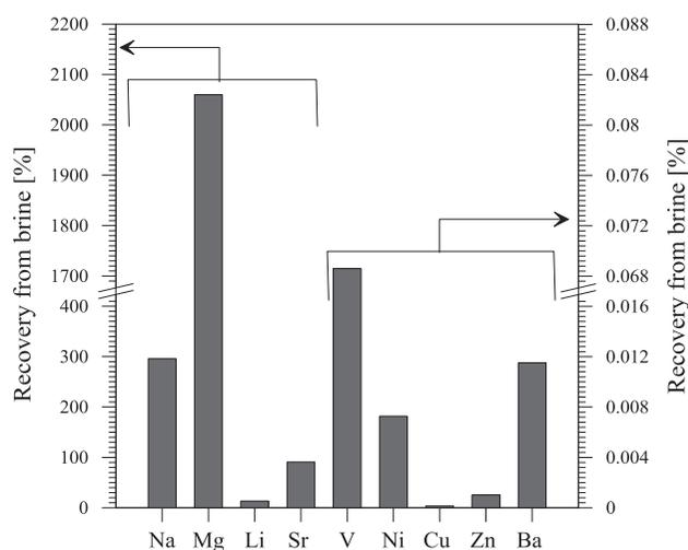
Fig. 7. Potential recovery of different metals from brine with respect to the annual mining. The annual mining is based on US Geological Survey [34]. The amount of Mg and Li mined in US is not available.
