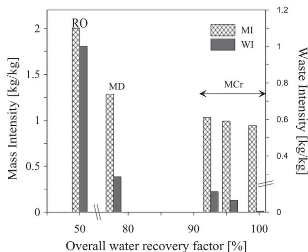
Fig. 10. Decrease in mass and waste intensities for the integrated membrane system consisting of RO, MD, and MCr (Only NaCl production has been taken into account).
