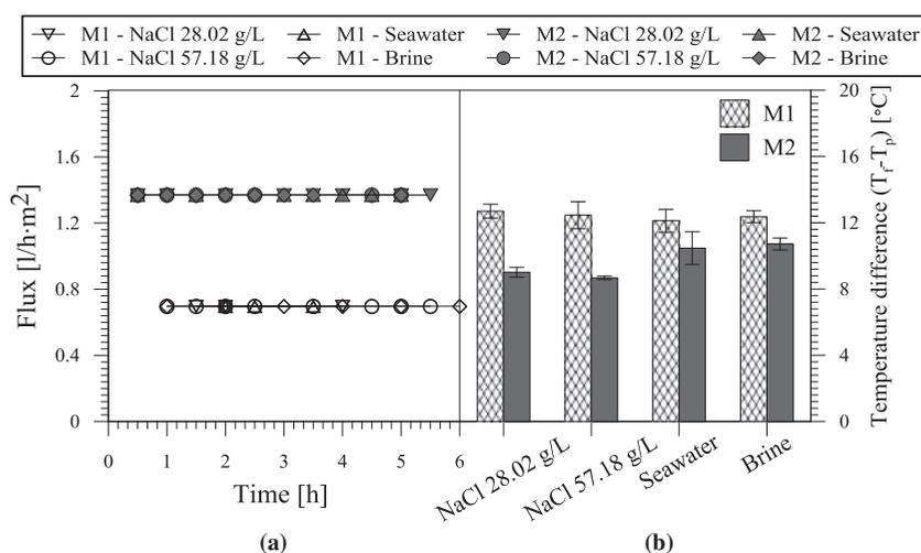
Fig. 3. (a) Transmembrane flux and (b) temperature difference for DCMD treatment of NaCl solutions, synthetic sea water and RO brine.
