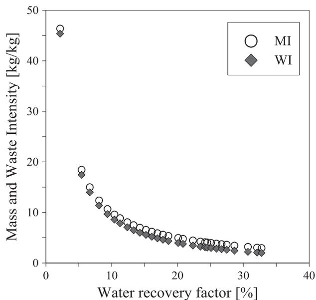
Fig. 8. Mass and waste intensity for a lab-scale MD and MCr plant. The water recovery factor is with respect to the concentration of RO brine.
