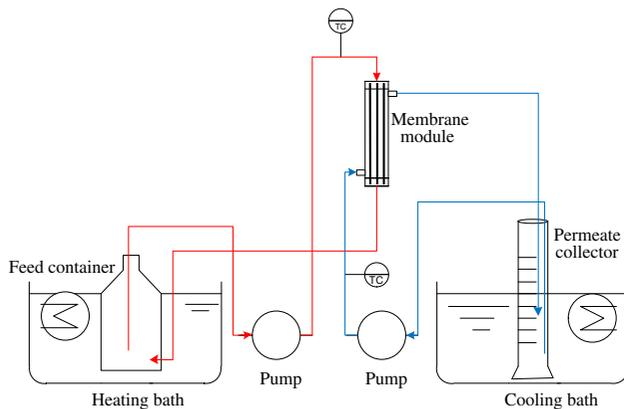
Fig. 2. Schematic representation of the lab-scale MD plant used for MD and MCr tests.
