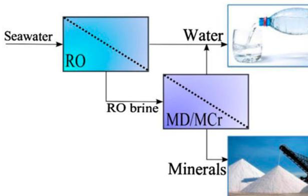
Fig. 1. Flow sheet for integrated systems for approaching ZLD in desalination.
