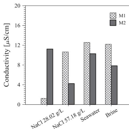
Fig. 4. Conductivity of permeate for the carried out DCMD tests with NaCl solutions, sea water, and RO brine used as feed.
