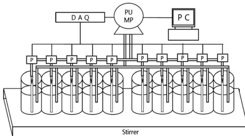
Fig. 2. Schematic diagram of a device for TMP measurement of MF hollow fiber.
