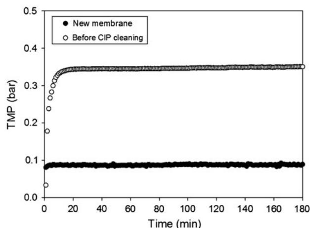
Fig. 1. Comparison of TMP profiles between new and fouled membranes.
