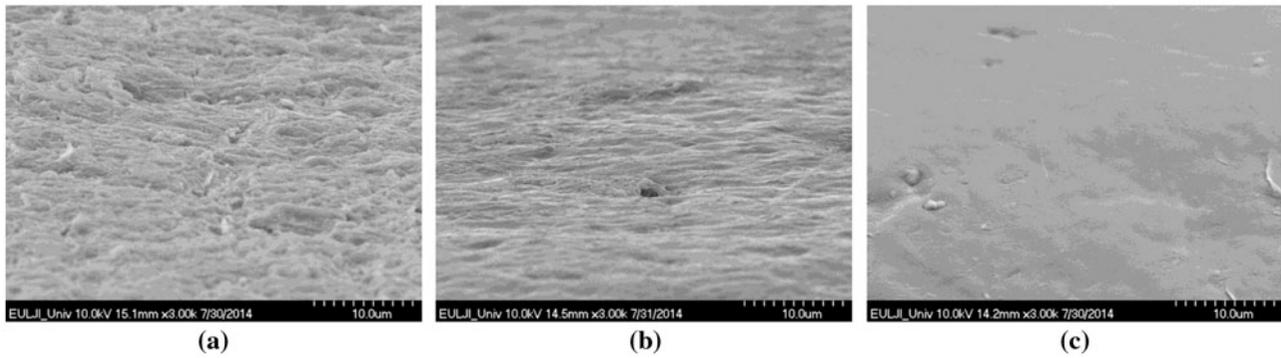
Fig. 4. SEM images of (a) used membrane before treatment, (b) used membrane after chemical cleaning, and (c) new membrane.
