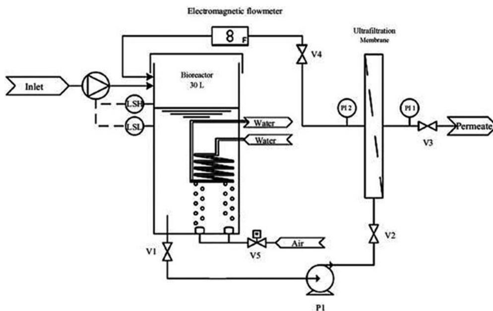
Fig. 1. Experimental set up of MBR. P: pump, V: valve, LSH: level security high, LSL: level security low, PI: pressure indicator.
