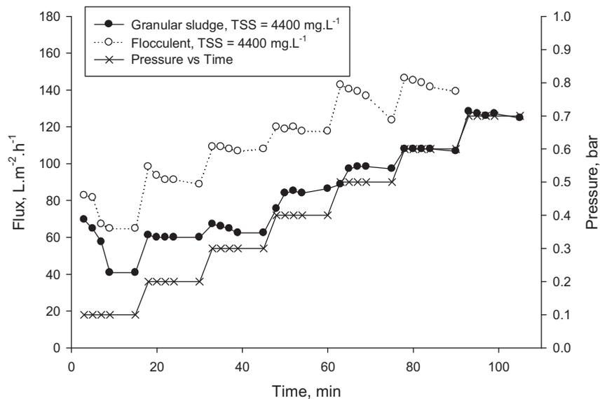
Fig. 5. Flux vs. time for granular and flocculent sludge at different pressures (TSS = 4,400 mg L<sup>-1</sup>).
