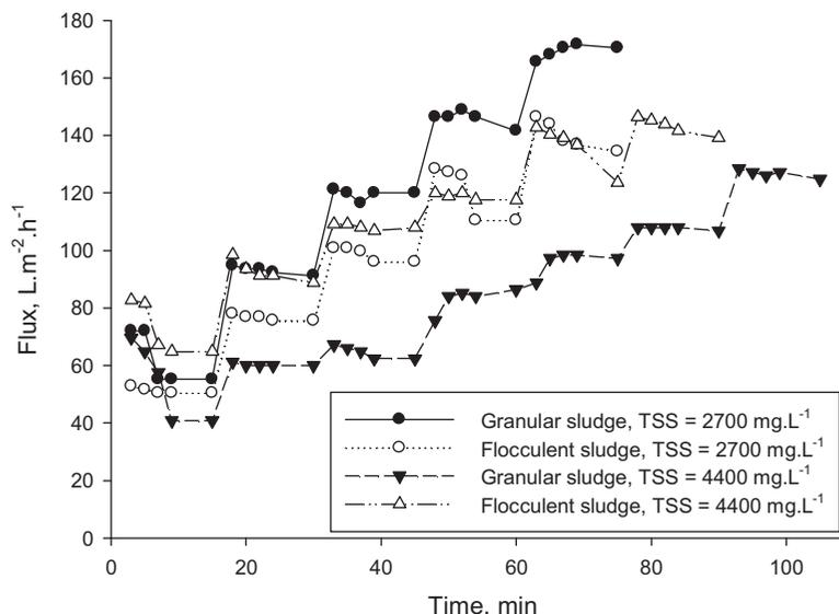
Fig. 6. Flux over time for both granular and flocculent sludge at TSS values of 2,700 and 4,400 mg L<sup>-1</sup>.
