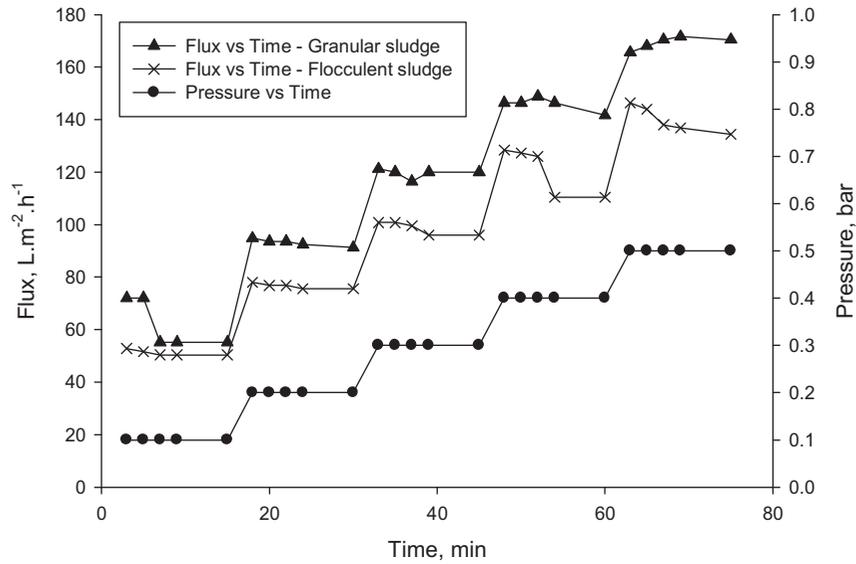
Fig. 4. Flux vs. time for granular and flocculent sludge at different TMP (TSS = 2,700 mg L<sup>-1</sup>).
