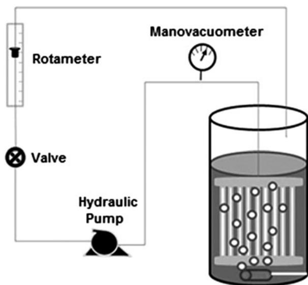
Fig. 1. Schematic flow diagram of the microfiltration system.
