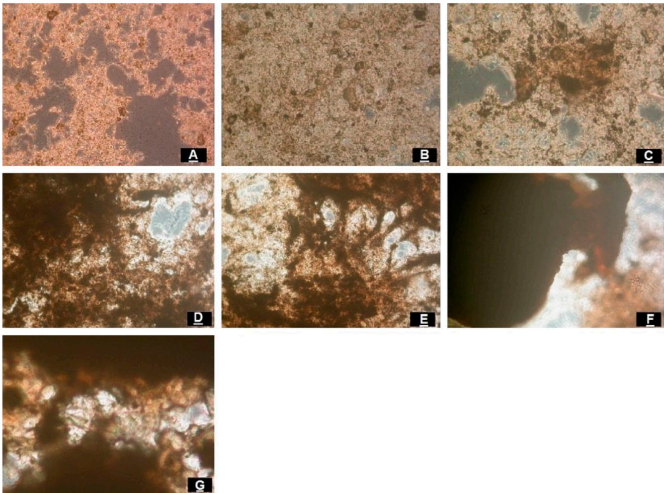
Fig. 2. Photomicrographs of the granular sludge reactor as settling time was reduced. (1)–(3) Flocculated sludge; (4) beginning of granule production; (6) majority of sludge formed by granules; (7) granular sludge.
